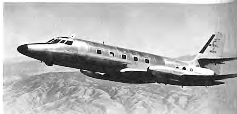
Lockheed JetStar has been fitted with "variable stability" characteristics to duplicate as closely as possible the control responses of the supersonic transport.
