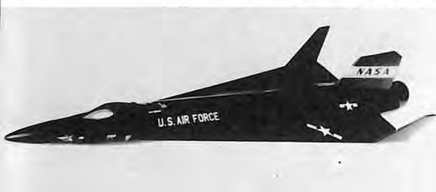
X-15 will be modified to provide a delta wing configuration. This research aircraft, built by North American, will be flown at Mach 8 to obtain aerodynamic and structural data.
