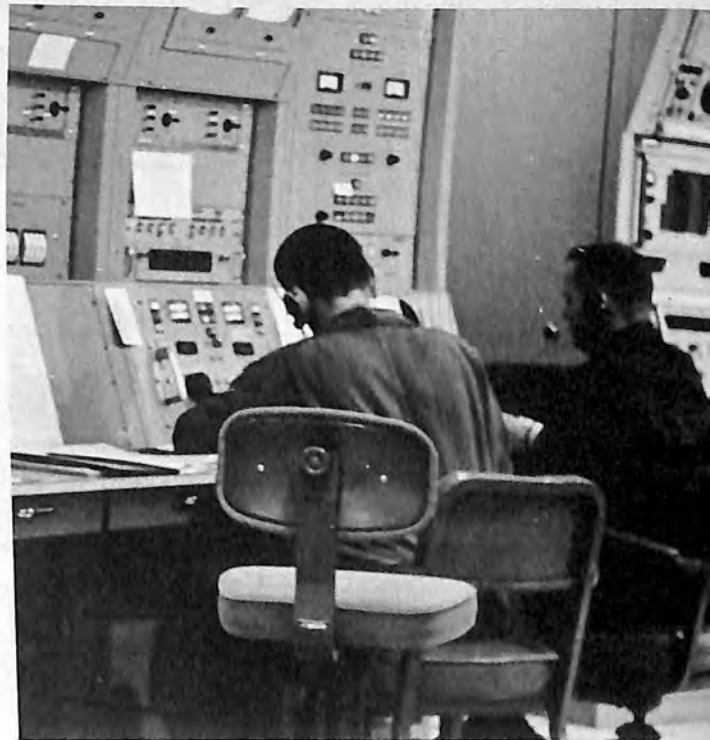
The 210-foot antenna is checked out by technicians at the servo control console.
