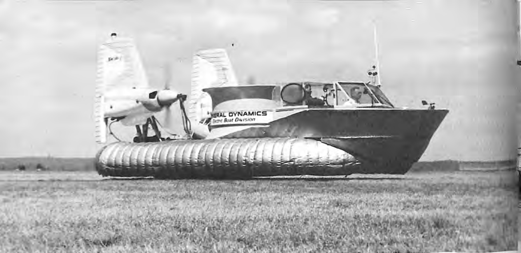
This 22-foot surface effect ship was built by the Electric Boat Division of General Dynamics Corp. Above, the craft moves across land. This vessel has achieved 60 knots over water.
