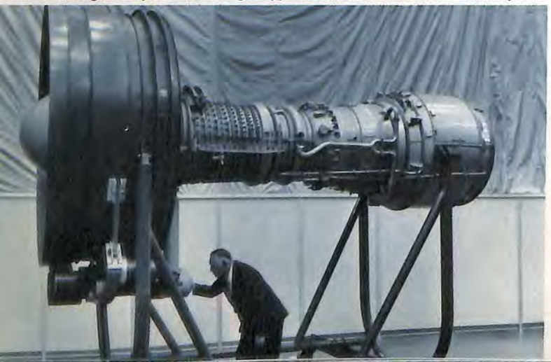
Three General Electric CF6/36-6 high bypass turbofan engines power the DC-10. Large fan provides a high bypass ratio for low fuel consumption.
