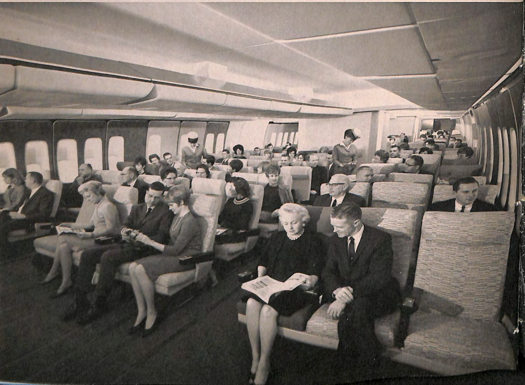
Mockup of Boeing 747 shows the three economy class sections. The 20-foot fuselage allows use of wider seats than current jetliner economy sections. (See Jet Transports: The Third Generation , page 10).
