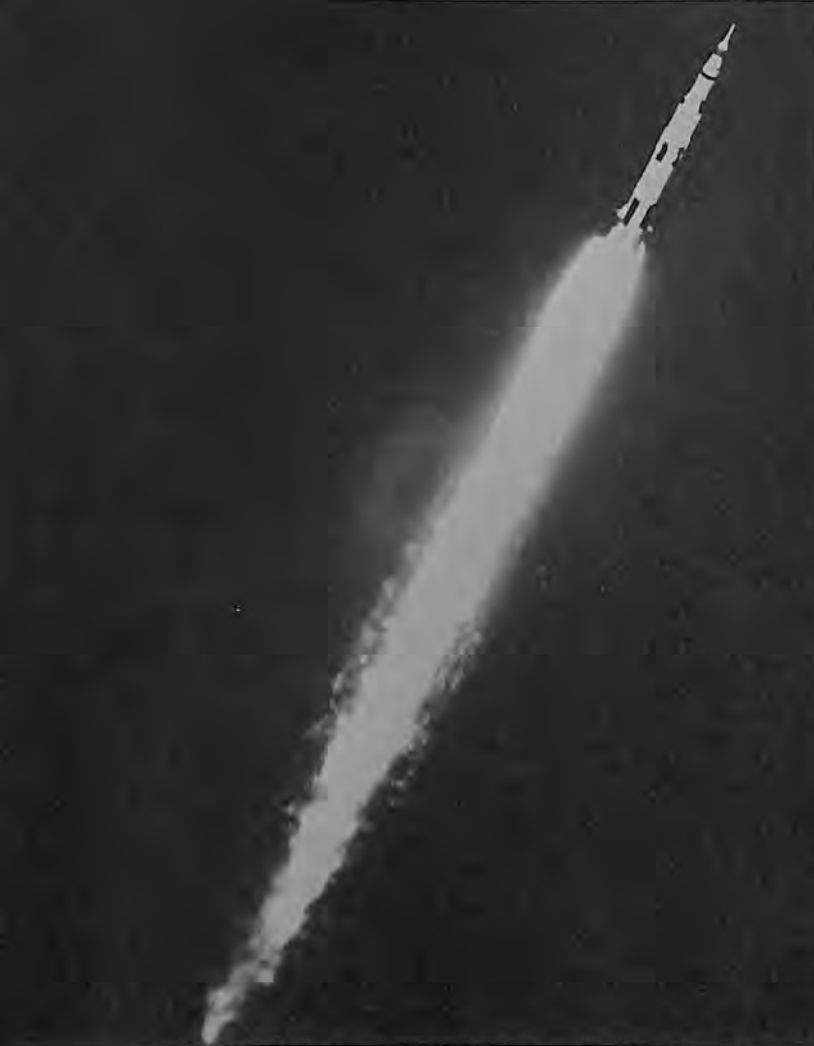
Apollo 4 takes off on its historic mission. The five F-1 engines, in addition to providing the primary thrust of 7,500,000 pounds, demonstrated their ability to "gimbal" or change the thrust line and make course corrections.
