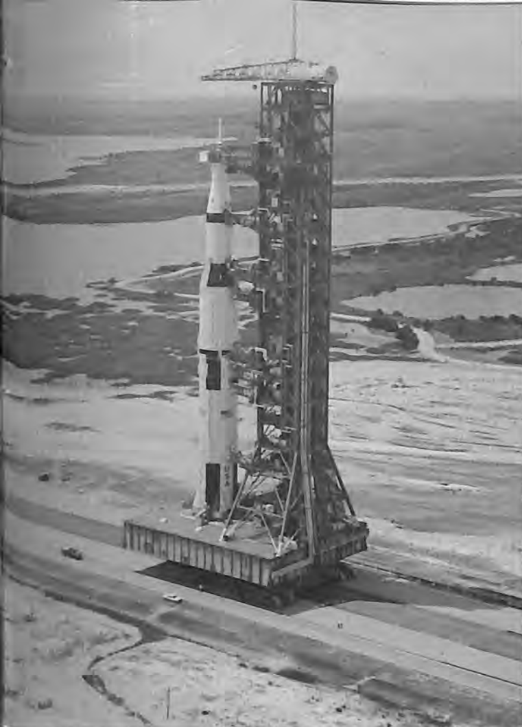
Apollo 4 starts on its journey from the Vertical Assembly Building to the launch pad. The mobile launch concept achieved its major goal of reducing the time the launcher/stack must spend unprotected on the pad.
