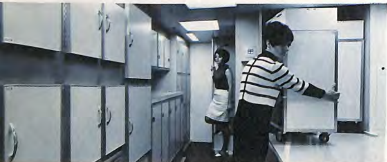
A centralized food preparation center in the DC-10 is located on the deck below the main passenger area.
