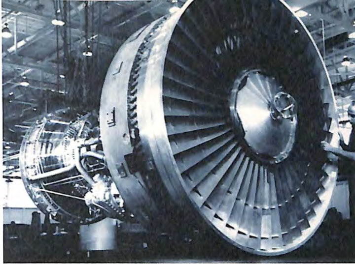
Four Pratt & Whitney Aircraft JT9D advanced technology turbofan engines power the 747. Each engine produces more than twice the thrust of the JT3D which powers the 707.
