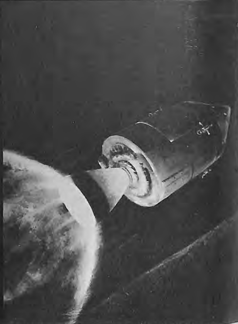
Artist's conception shows the Apollo spacecraft Service Module engine firing. This engine handles all major velocity changes on a moon mission such as course corrections and injection into orbit around the moon.
