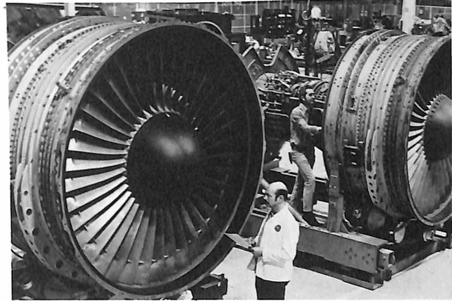
General Electric CF6-50 engines, rated at 50,000 pounds of thrust, have been shipped for use in the McDonnell Douglas DC-10 Series 30 aircraft, Airbus Industries A300B and the Boeing 747-300.
