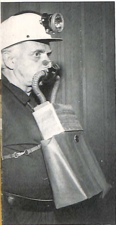
A Lockheed engineer demonstrates an experimental self-rescue breathing device designed to provide a one-hour emergency supply of oxygen to miners in the event of an underground disaster.
