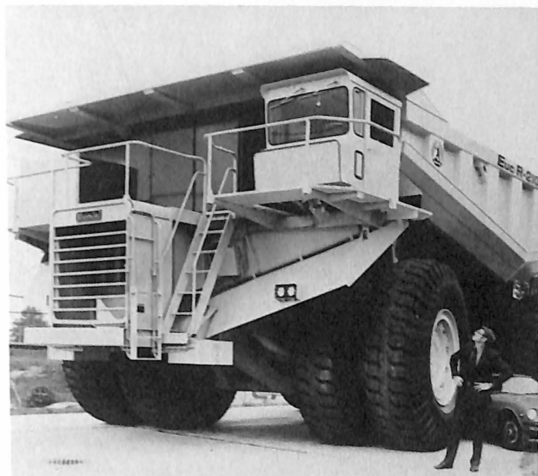
An Avco Lycoming gas turbine engine powers this 210-ton ore hauler. The engine provides the power for interchangeable electric motors at each of the truck's four wheels.
