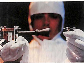
A miniature thruster (right) for a Strategic Defense Initiative system is compared with a previous configuration of comparable power by a technician of The Marquardt Company, a subsidiary of ISC Defense and Space.
