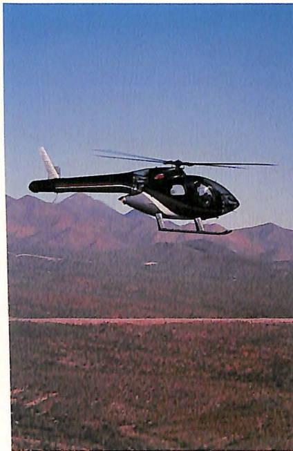
McDonnell Douglas Helicopter Company was conducting research with an experimental NOTAR (No Tail Rotor) helicopter.
