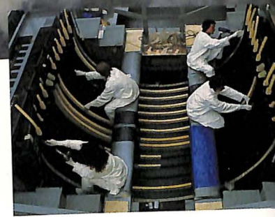
Heath Tecna Aerospace initiated fabrication of the all-graphite MD-11 center engine inlet duct, designed for substantial weight saving.
