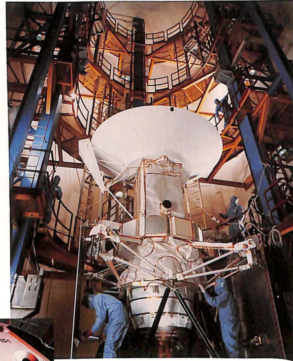
NASA's Magellan spacecraft, which will map Venus after April 1989 launch, is shown being prepared for a stress test. Martin Marietta is spacecraft contractor.
