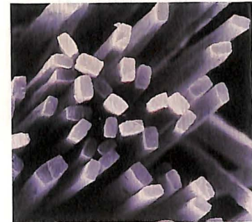
BASF Structural Materials' Celion Carbon Fibers division completed construction of a facility for production of new types of "melt-spun" noncircular fibers that offer improved strength in composite applications.
