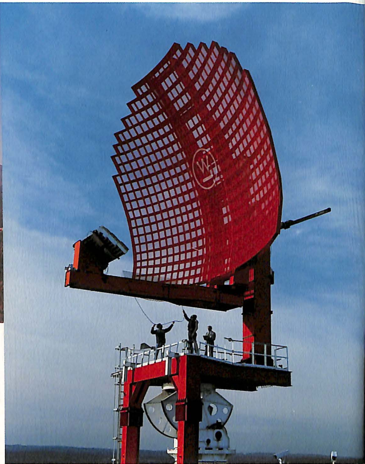
Westinghouse Electronic Systems Group was working on an order for 40 long-range ARSR—three dimensional radar systems for joint use by the Federal Aviation Administration for air traffic control and the USAF for air defense.
