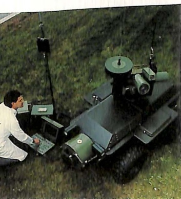
Martin Marietta Aero & Naval Systems developed a Tactical Multipurpose Automated Platform (TMAP) that can perform reconnaissance in high-threat battlefield areas as far as four miles from its soldier-operator.
