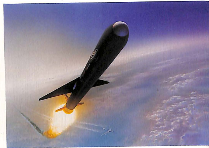
Artist's concept of the Pegasus air-launched space booster after separation from its carrier aircraft. Pegasus, targeted for mid-1989 first flight, is a private development of Hercules Aerospace and Orbital Sciences Corporation.
