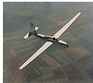
In flight test status was the record-setting all composite EGRETT, intended for such applications as search/rescue, geophysical survey, and coastal/border patrol. Powered by a Garrett turboprop, it was jointly developed by E-Systems and the West German firm Grob TFE.
