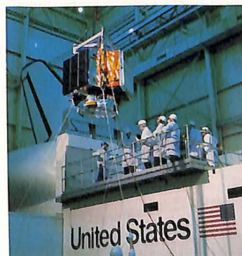
Shown undergoing test at Goddard Space Flight Center is Fairchild Space Company's Multimission Modular Spacecraft, which will be the platform for the GE-instrumented Upper Atmosphere Research Satellite.
