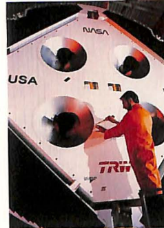
An engineer is making an adjustment to a full-scale model of the Orbital Maneuvering Vehicle being developed for NASA by TRW Space & Technology group.
