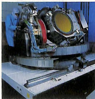
Hughes Aircraft developed an advanced longwave infrared sensor that will be used to assess the feasibility of using optical sensors for ballistic missile tracking and detection.
