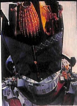
Principal payload of STS-26 was the TRW-built Tracking and Data Relay Satellite. Visible at top photo are the large umbrella-like parabolic antennas developed by Harris Corporation.
