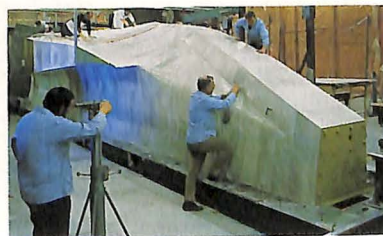
Heath Techna Aerospace neared completion of the 60-foot wing-to-body fairing master model for the Air Force/McDonnell Douglas C-17 airlifter, scheduled for first operational service in 1992.
