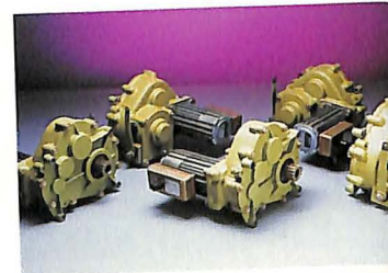
Lucas Aerospace was producing these components for the Boeing 747, units associated with the gearbox drive that moves cargo containers into and out of the airplane.
