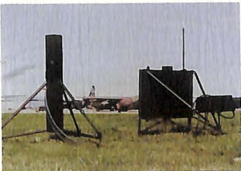
Bell Aerospace Textron was awarded an Air Force contract to develop a Mobile Microwave Landing System, enabling aircraft to locate and land at strips in a forward battle area.
