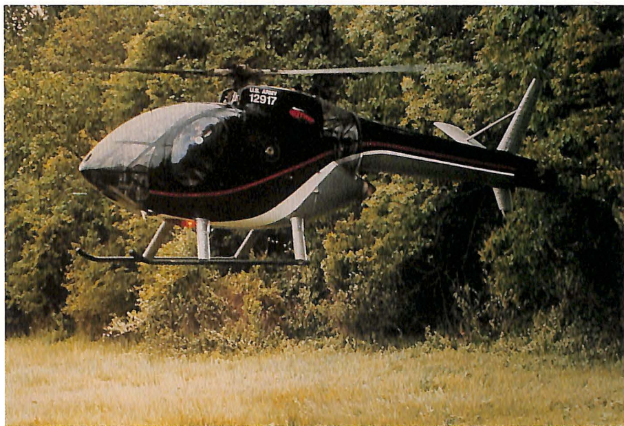
McDonnell Douglas Helicopter Company's MD530N NOTAR (No Tail Rotor) helicopter made its first flight in December.
