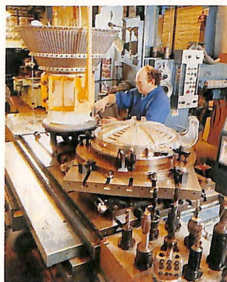
An Aerojet technician works on a Titan rocket engine thrust chamber. Aerojet provided the liquid rocket engine for the Titan IV military launch vehicle and the Commercial Titan.
