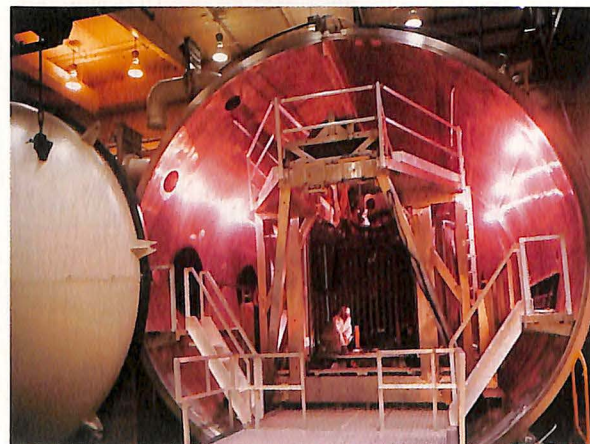
Sensors for the Defense Support System (DSP) satellites undergo test at GenCorp's Aerojet ElectroSystems plant. ElectroSystems developed the sensor payload for the TRW-built DSP satellites.
