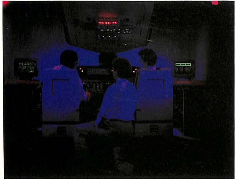
Honeywell engineers conduct an avionics software test in a specially designed MD-11 simulator; Honeywell is avionics systems integrator for the MD-11 trijet.
