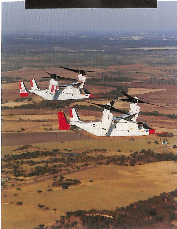
The Bell-Boeing V-22 Osprey tilt rotor military aircraft began its flight test program in March. The photo shows the first formation flight of two prototypes, accomplished in November.
