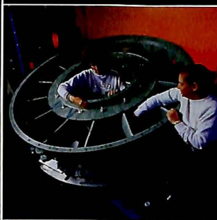
Precision Cast Parts Corp. produces this turbine rear frame casting for a Boeing 777 engine.
