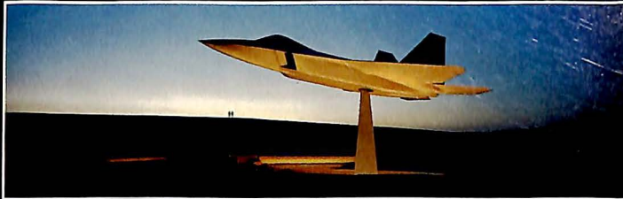
A high-fidelity pole model of the USAF/Lockheed F-22 advanced tactical fighter was built for radar cross-section measurements to evaluate the aircraft's low observable (stealth) characteristics.
