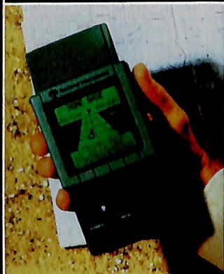
Rockwell's Collins Avionics & Communications Division developed a lightweight, hand-held airborne navigation system for use with the Navstar Global Positioning System. It is designed for both military and civil use in portable and vehicular applications.
