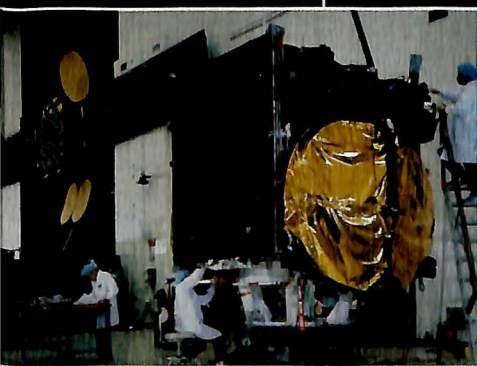
The Transfer Orbit Stage (TOS) undergoes checkout prior to its launch as the upper stage of a Titan III launch vehicle on the Mars Observer mission. Martin Marietta manufactured the TOS for Orbital Sciences Corporation.
