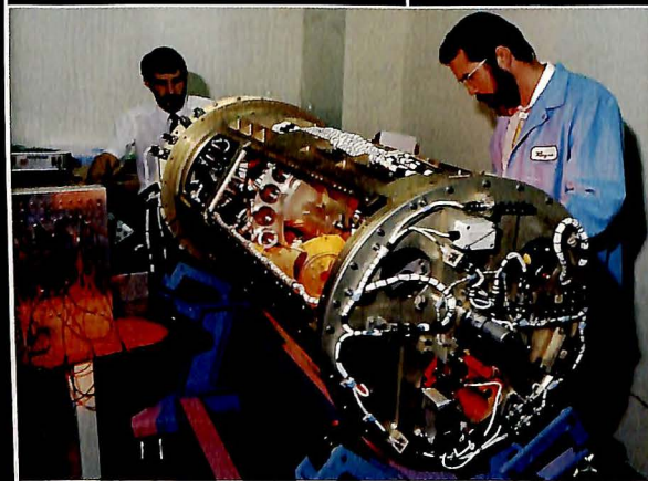
Flown on the June/July U.S. Microgravity Laboratory mission was the Crystal Growth Furnace developed by Teledyne Brown Engineering.
