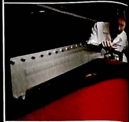
A BFGoodrich Aerospace engineer checks the first production unit of a new all-composite Pneumatic Impulse Protection system.
