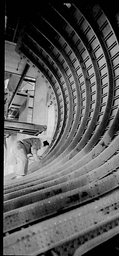
Using improved techniques and technology, Northrop significantly reduced its airborne emissions by reducing the amount of paint used in each Boeing 747 center fuselage section (pictured) by 1,000 pounds.
