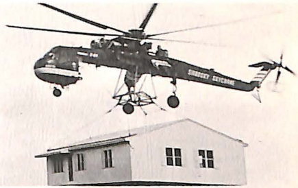
A Sikorsky Skycrane lifts a complete house to demonstrate aerial delivery of assembly line dwellings from factory to home site. This offers a far-reaching potential for applying modern production techniques to meet the world's critical demand for low-cost housing.
