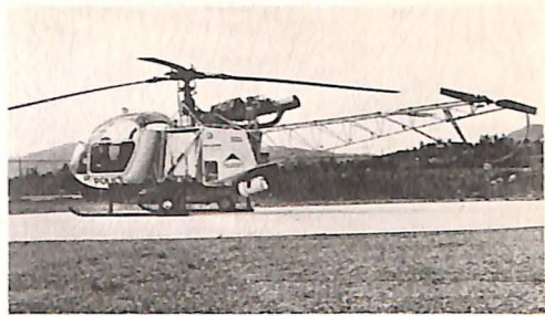
New York's Suffolk County Police operate this Alouette II — 5-place, turbine powered helicopter for traffic survey and crime patrol.
