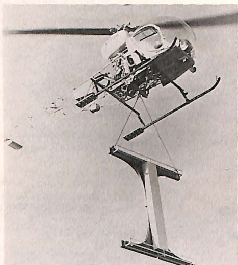
This "I" in the sky is enroute to the top of the International Hotel, Calgary, Canada, via a United Helicopters Ltd., Bell 47G-3B-2. Eighteen of the huge letters were airlifted from six blocks away to the roof of the hotel, 310 feet above ground, in one hour and 45 minutes. Each is 12 feet high and weighs about 450 pounds.
