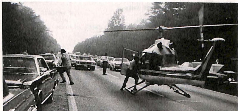
A Fairchild Industries turbine-powered FH-1100 ambulance helicopter, equipped with two inside litters, seat for medical attendant, plus pilot, lands near a highway accident.
