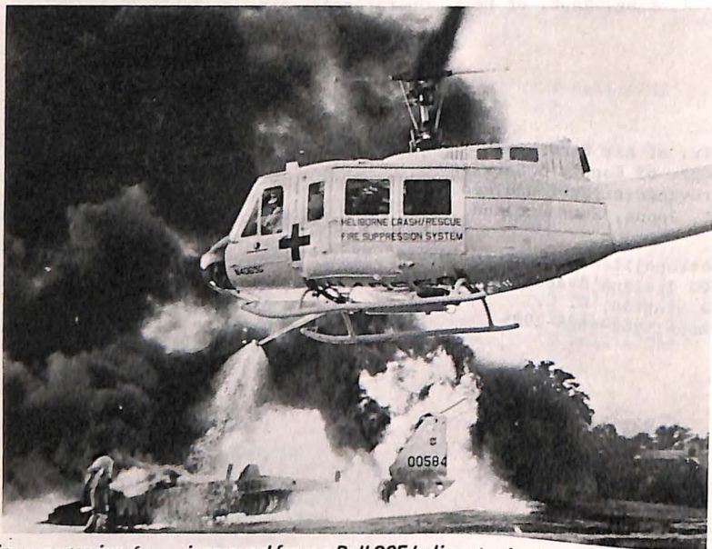
Fire-suppressing foam is sprayed from a Bell 205 helicopter in demonstration of new techniques for evacuating persons from burning aircraft. System, developed for military purposes, is now being used by civil agencies.
