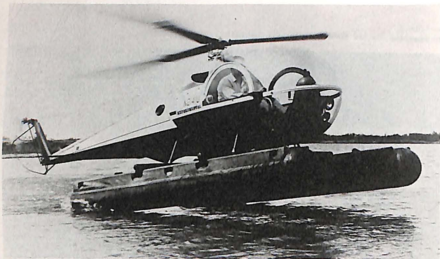
A Brantly-Hynes Model B-2B -- equipped with floatation gear -- ready for water rescues or to land where the fish are biting.
