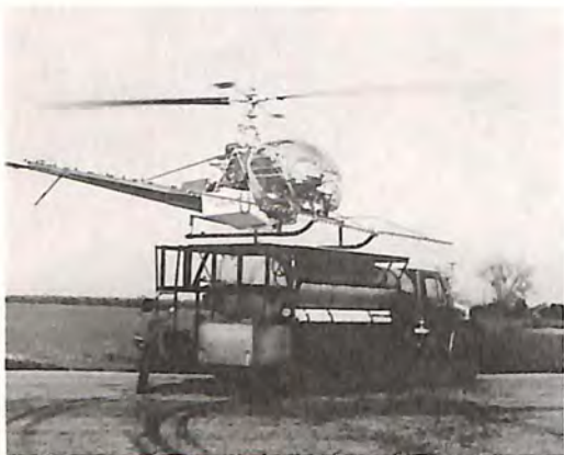
In Creston, Iowa, Moore Helicopter Services' Bell 47G-2 lands on this truck-top helistop to re-load for spraying.
