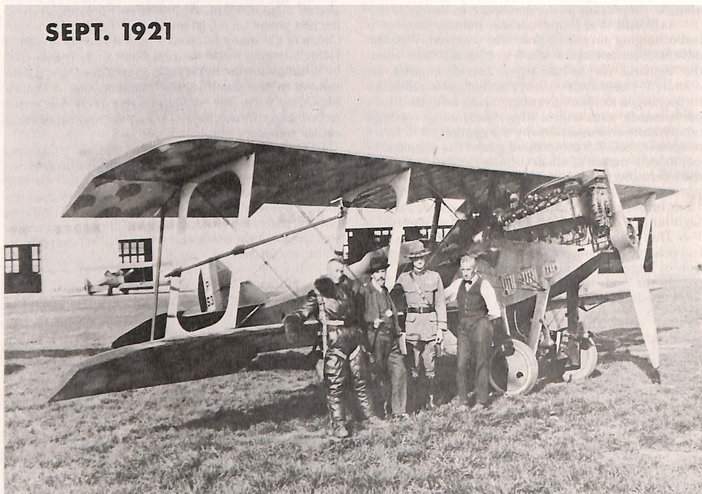
In 1921, the LePere biplane with General Electric's supercharged engine set an altitude record of nearly eight miles.
