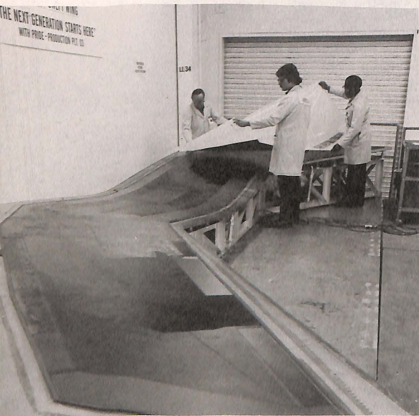
Technicians work on the composite forward-swept wing of Grumman Corporation's highly maneuverable X-29 experimental aircraft. Composites have a direct impact on aircraft aerodynamics and have made the performance of the X-29 possible.
