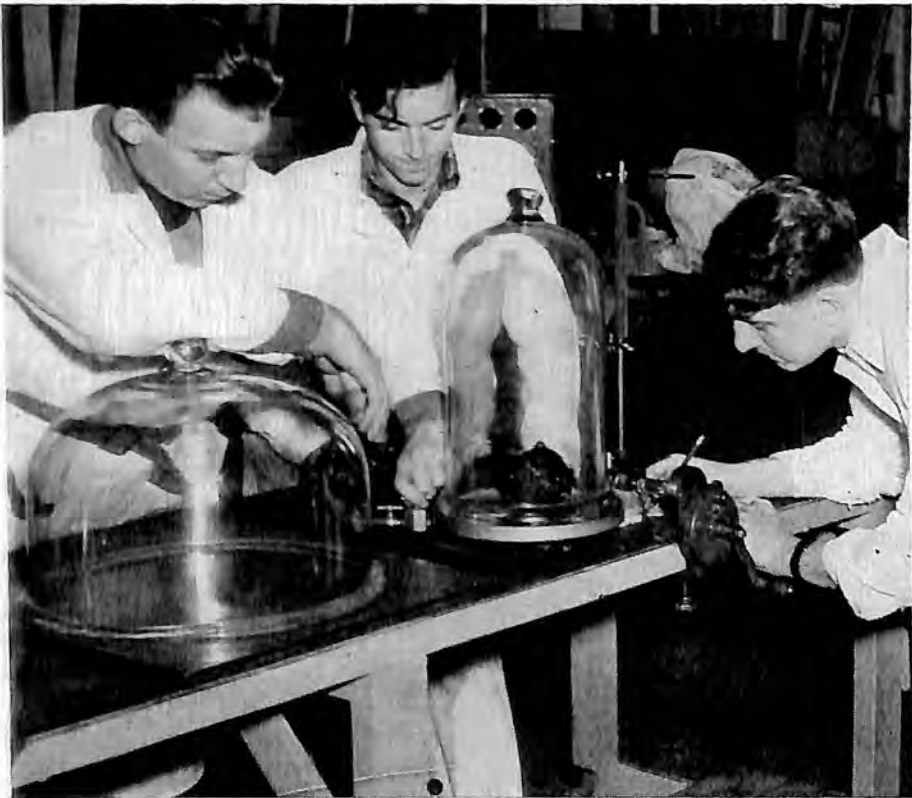
AT ROOSEVELT AVIATION SCHOOL Testing an altimeter in the instrument department.
