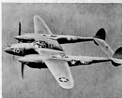
3. LOCKHEED P-38 "LIGHTNING," two-engine, twin-boom fighter in service on all important battle fronts.
