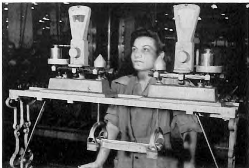
Measuring the weight distribution of an articulated rod for Wright Cyclone engine for the B-29 Superfortress. Wright Aeronautical Corporation, Paterson, N. J.
