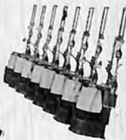
Battery of AWP Seat Grinders used by one manufacturer.
