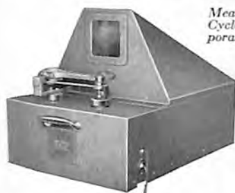
SHADOWGRAPH, an electrically operated weighing unit of high accuracy for connecting rod balancing and selection.
