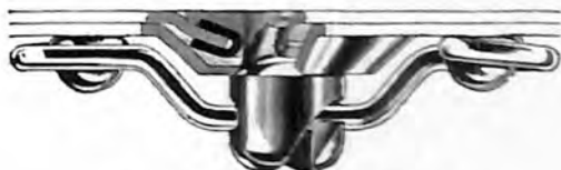
Complete assembly of the DZUS spiral cam fastener.
