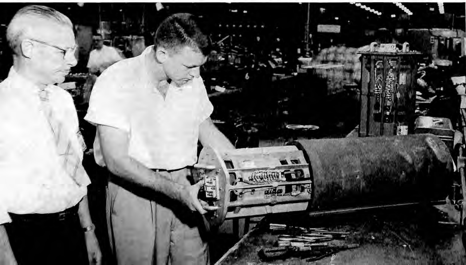
Engineer instructing removal of inverter from canister at Bendix-Red Bank.
