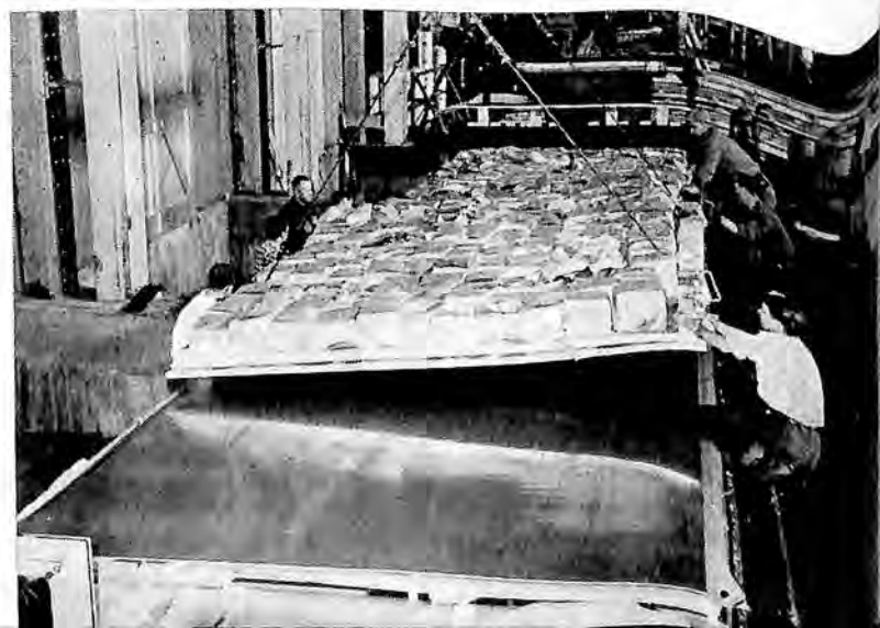
Alcoa's aluminum sheet is packed in dry ice for trip to Douglas plant.
