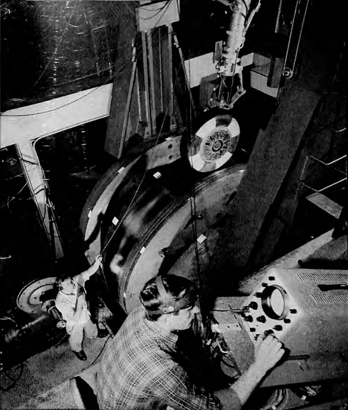
Giant landing gear test facility is 60 feet high. It simulates conditions that heavy, high-speed planes actually meet.
