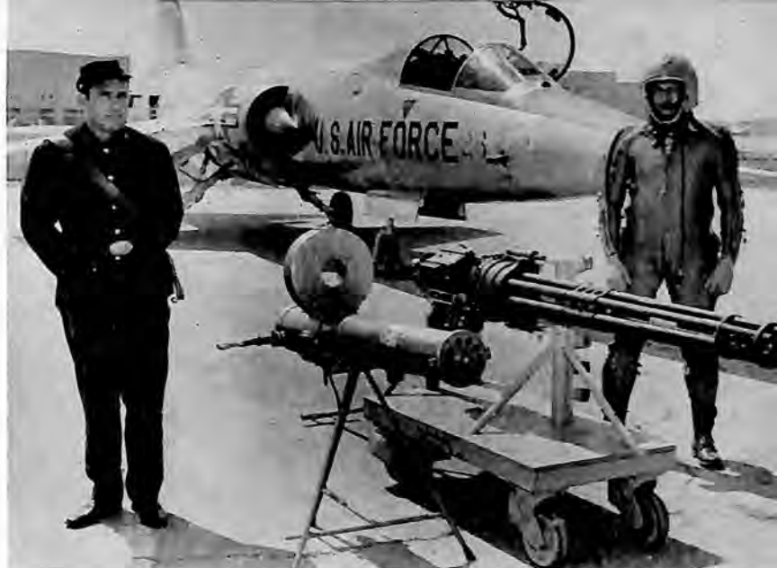
General Electric adapts Civil War Gatling Gun to arm Lockheed's F-104A Starfighter.
