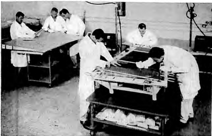
Lay-up room of the Hi-Temp Sandwich Structure department where stainless steel honeycomb core is assembled.
