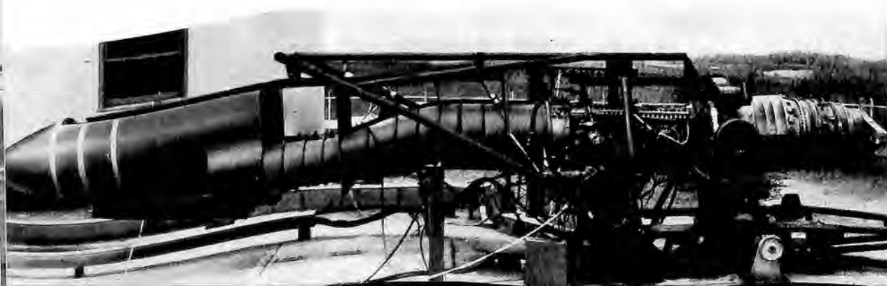
Rig used to test the Westinghouse J-34-WE-46 and T2J-1 inlet duct.
