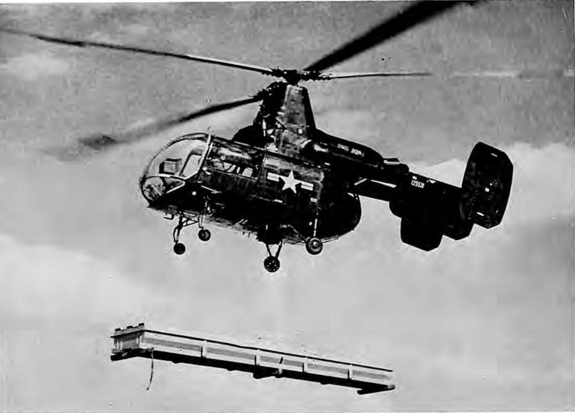
Kaman H-43B uses its external cargo hook for easy loading.
