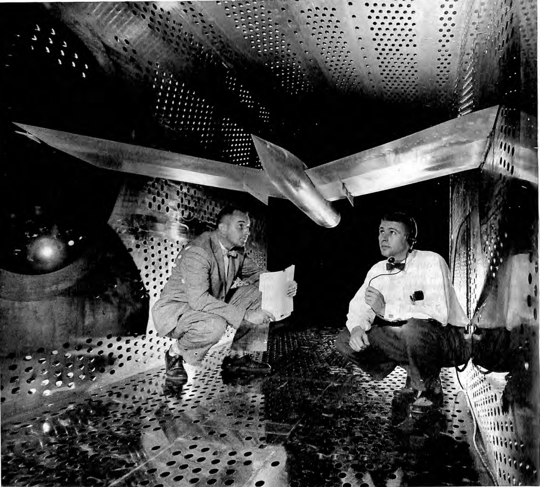
Scientists check model in test section of NACA wind tunnel.
