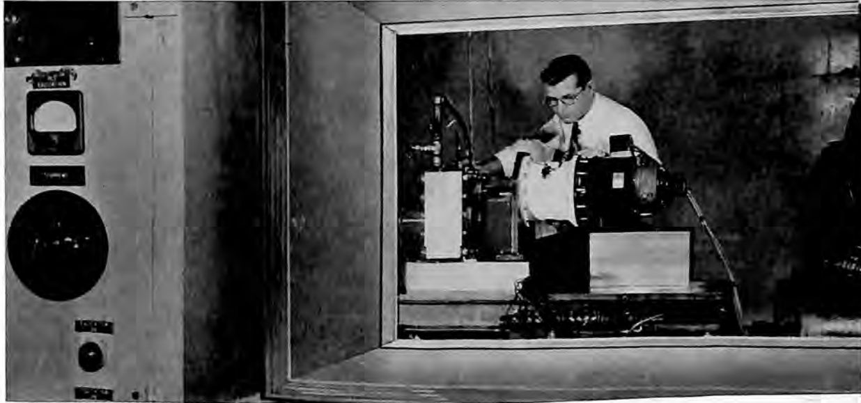
Lycoming engineer adjusts constant output speed drive in laboratory test cell.
