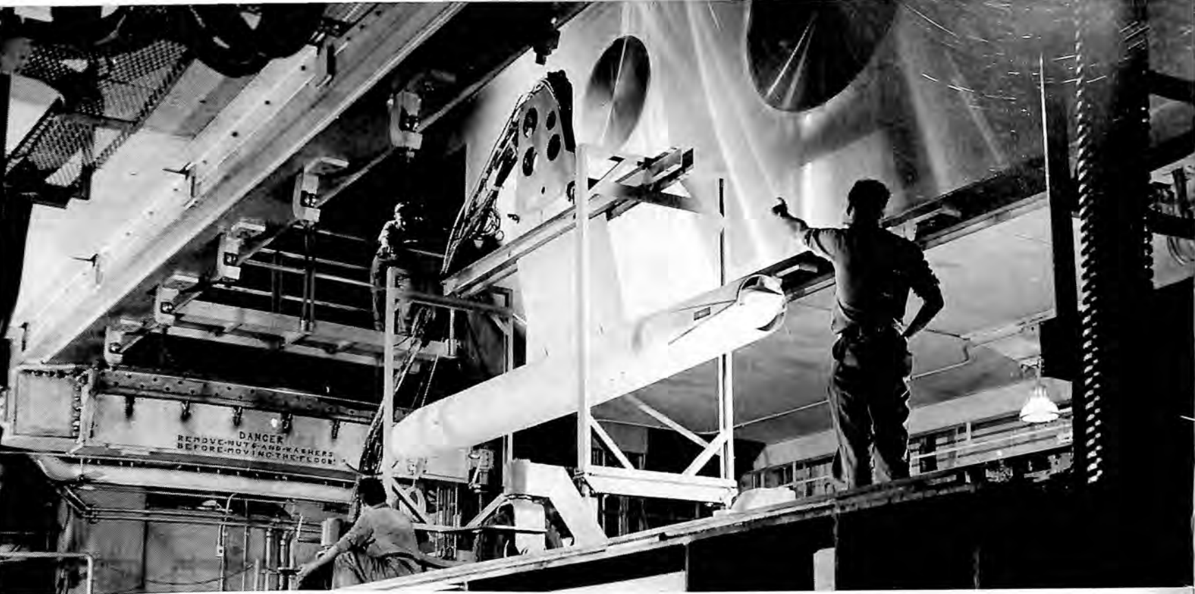
NACA 16-inch ramjet is elevated in Lewis Unitary Plan Wind Tunnel.
