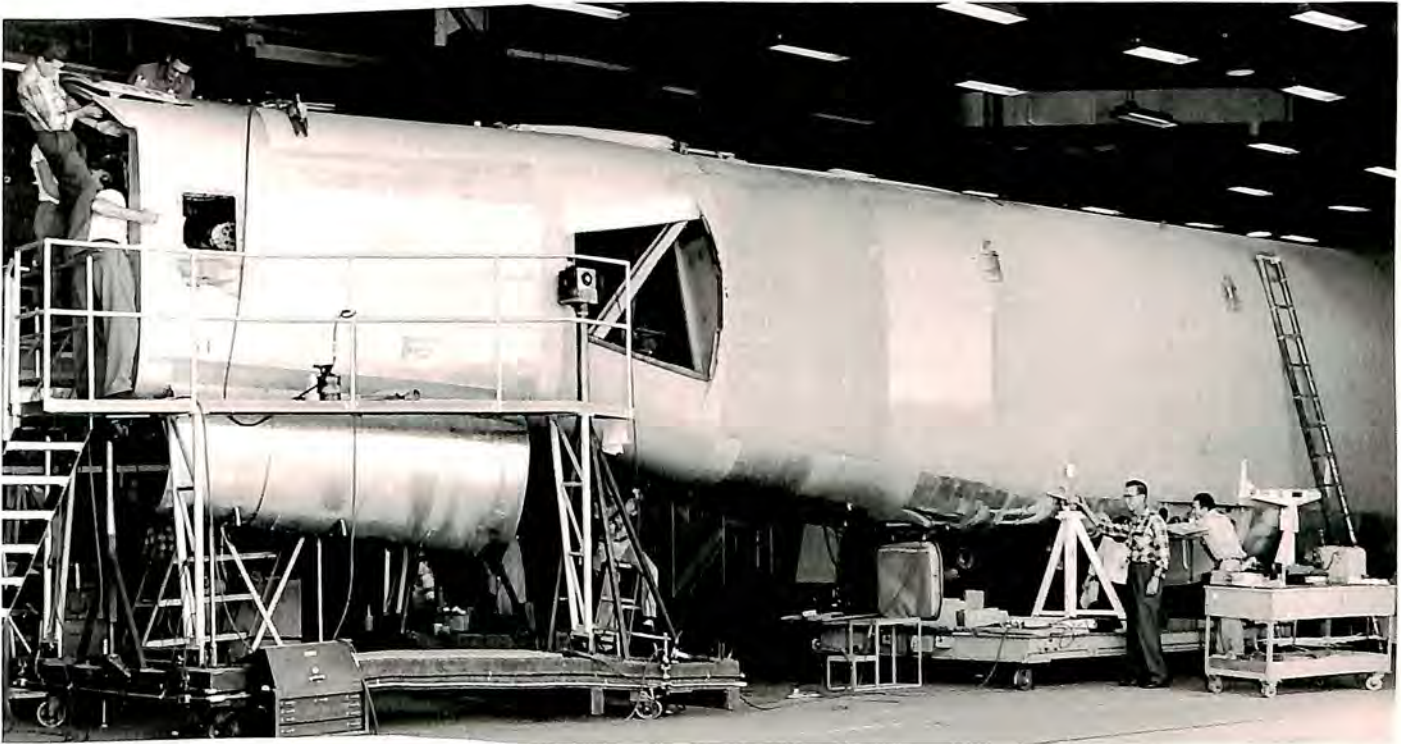
Boeing B-52 fuselage section nears completion at Temco's Dallas plant.
