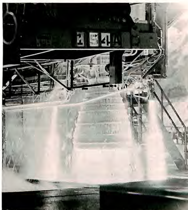
Thor engine in environmental chamber.
