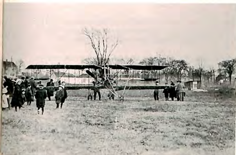
James Nolan's 1910 biplane with tail in front, engine in rear, had 32 horsepower Metz engine.
