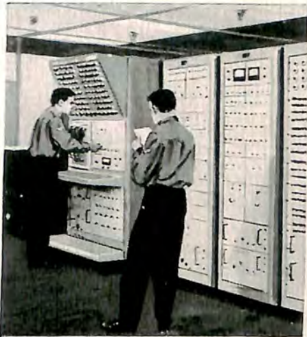
HIGH SPEED COMPUTERS housed in tower calculate target information from radar and provide intercept-destroy data.
