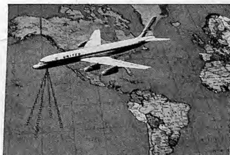
Bendix Doppler Radar bounces beams off the earth's surface, gives pilot pinpoint navigation data, permits him to take advantage of most favorable winds.
