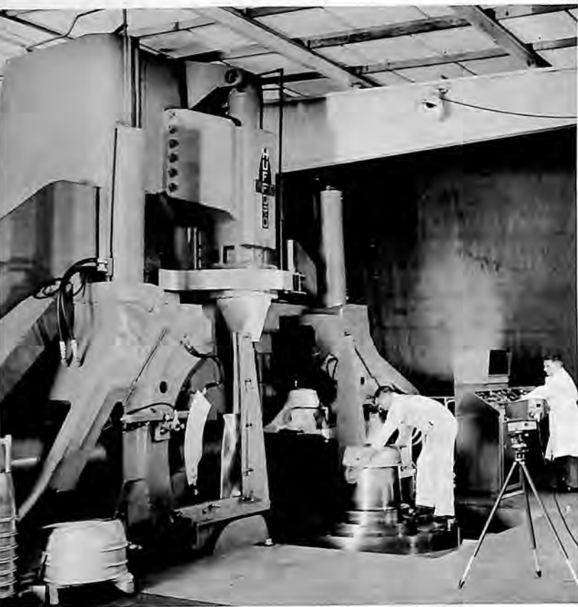
Ramjet parts on Marquardt forging machine.
