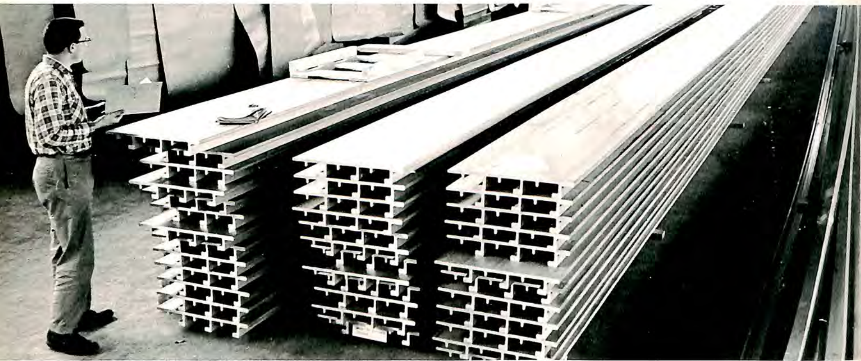
Aluminum wing panels for the B-52 are extruded on Dow's 13,200-ton press.
