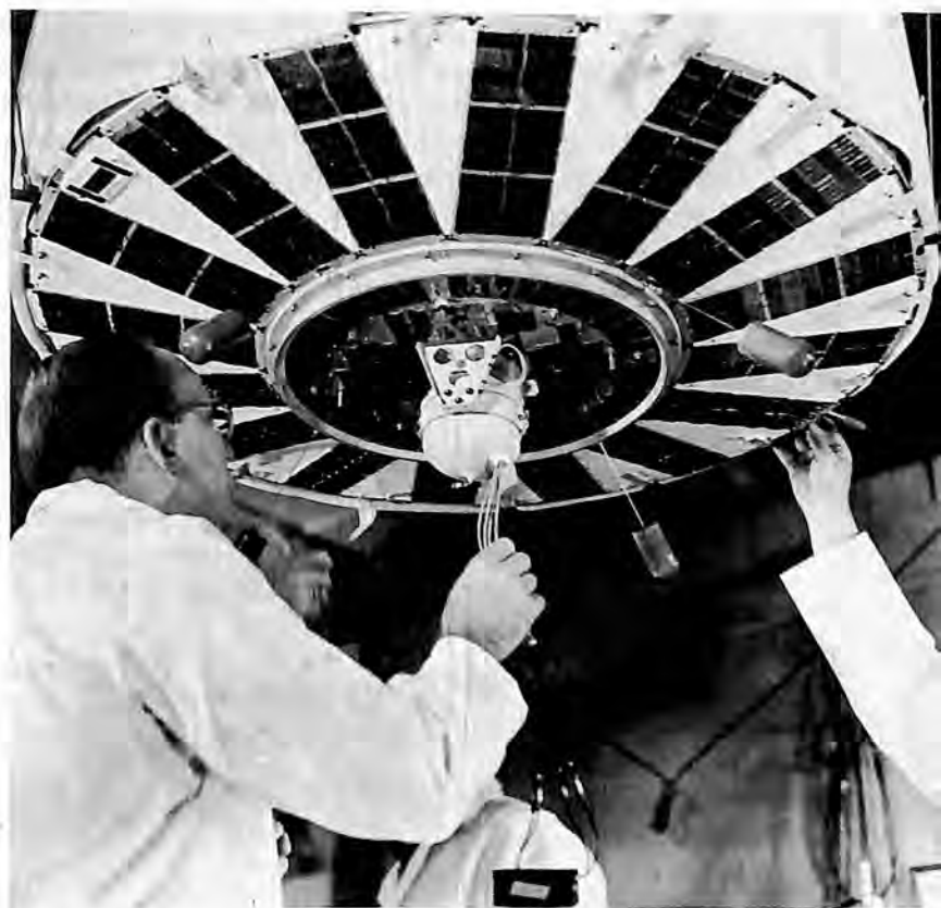
Martin's SNAP generator is fastened to Transit satellite prior to vibration tests.
