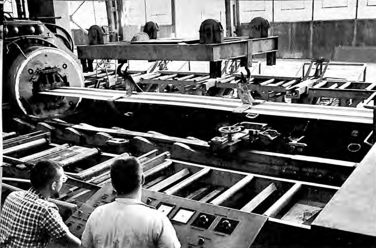
Dow extruded aluminum body panels for the Titan missile.
