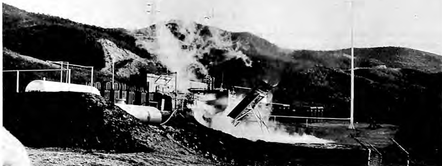
Marquardt demonstrated liquid air cycle operation, burning liquid air with hydrogen in 18-inch thrust chamber.
