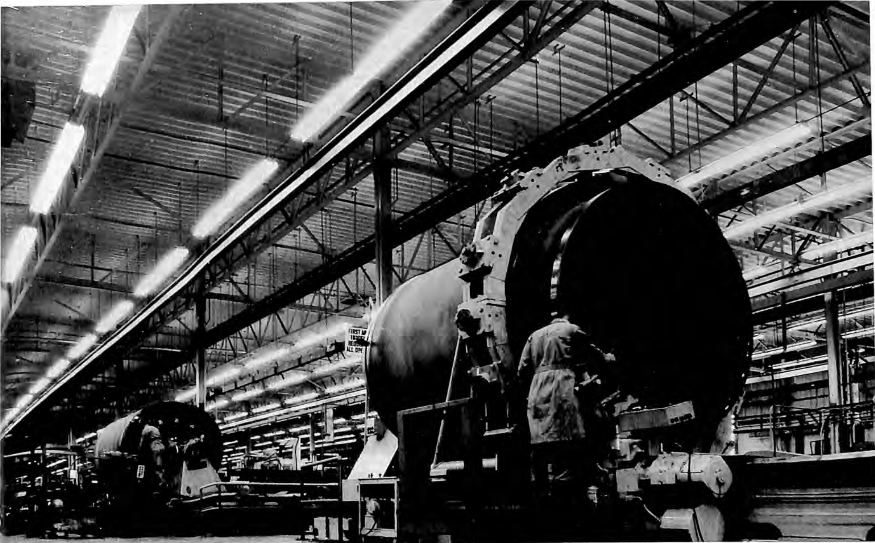
Aerojet's chamber segments for the 100-inch diameter solid rocket motor undergo final machining operations.
