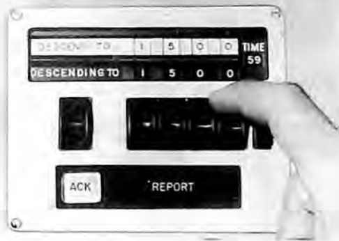
Lear was developing push-button air traffic communications display.
