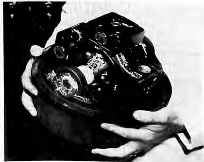
Lear's lightweight, gas-driven inertial guidance system.
