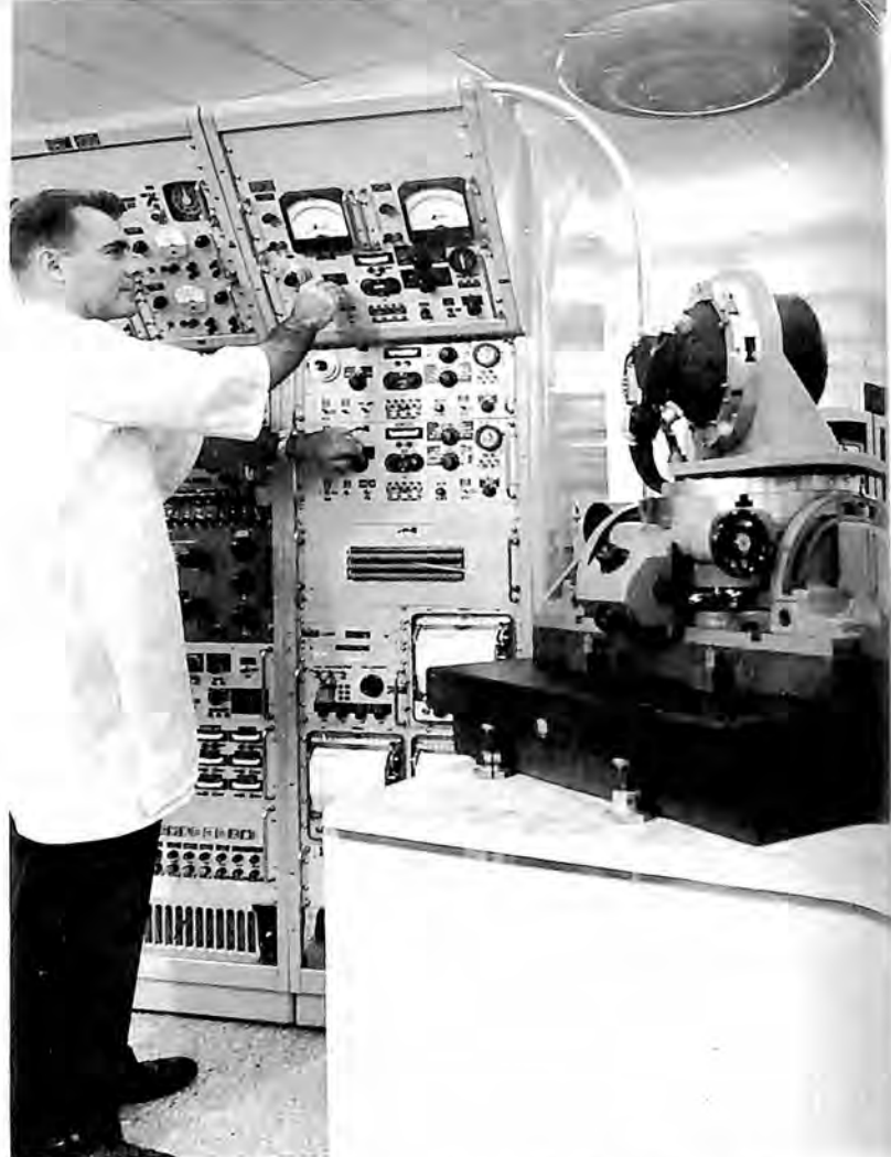
Above: Kearfott facility tests Missile Guidance Inertial System Platform (see p. 179)
