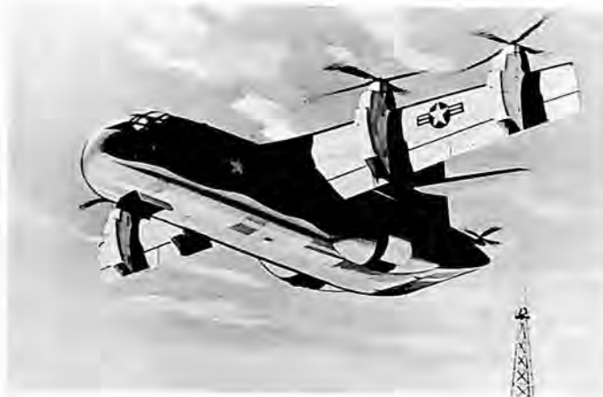
Artist's conception of tri-service VTOL craft under development by Chance Vought Corporation.
