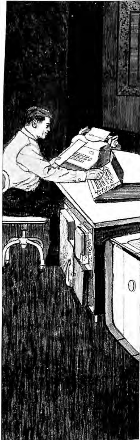
ELECTRONIC COMPUTERS. Re-comp II, the first all-transistorized compact computer, is manufactured by North American for industrial and scientific use. It telescopes hours of problem solving into seconds.
