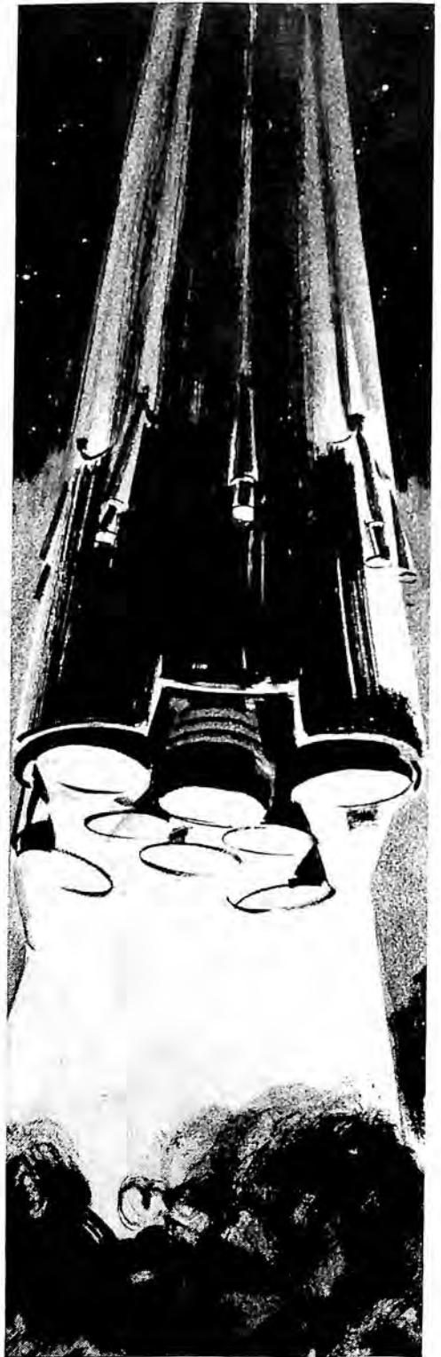
ROCKET ENGINES. NAA is producing the engines for the Saturn space booster which will have 1½-million-lb. thrust at launch. For Nova-class vehicles, NAA is developing the F-1, a 1½-million-lb. thrust single unit.
