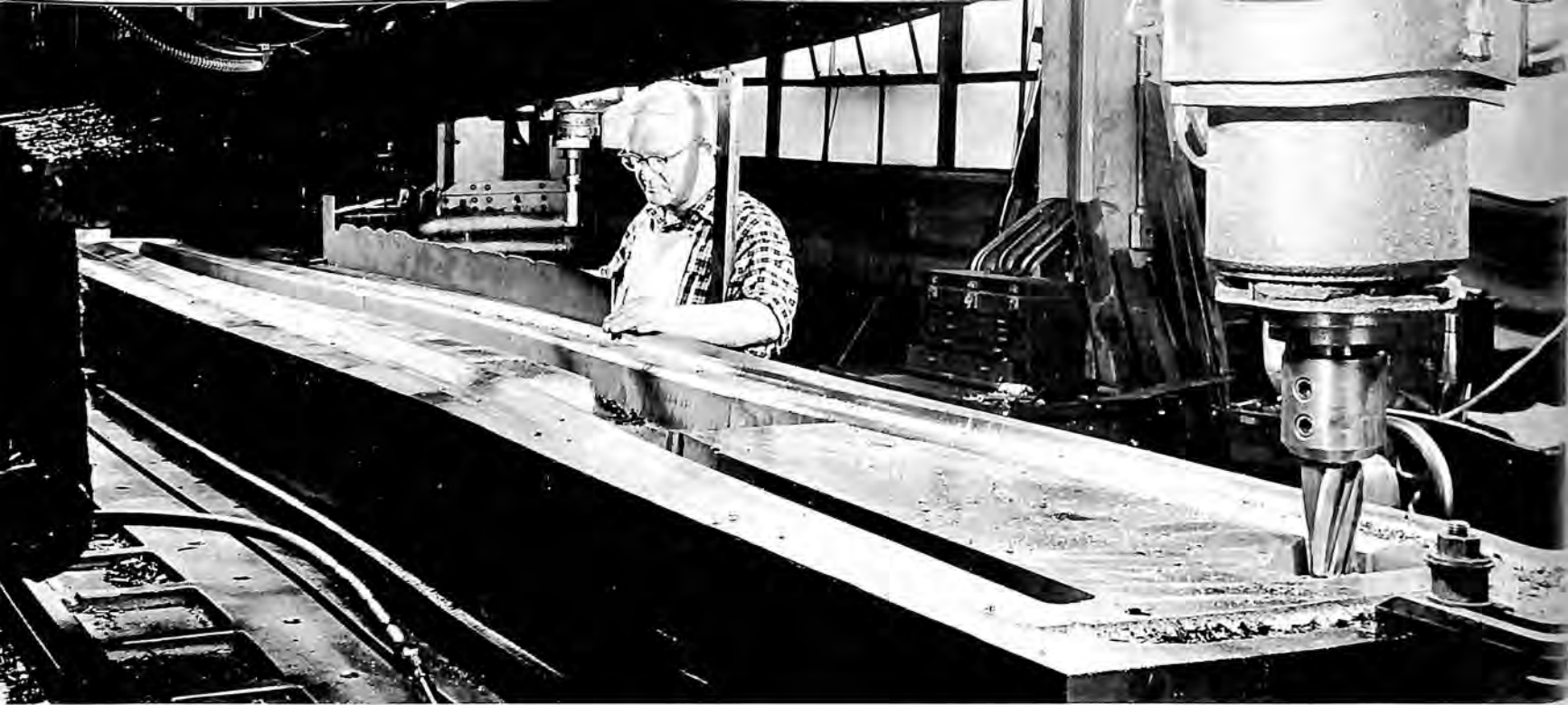
Alcoa forged aluminum front wing spars for the Navy's F4H fighter-interceptor.
