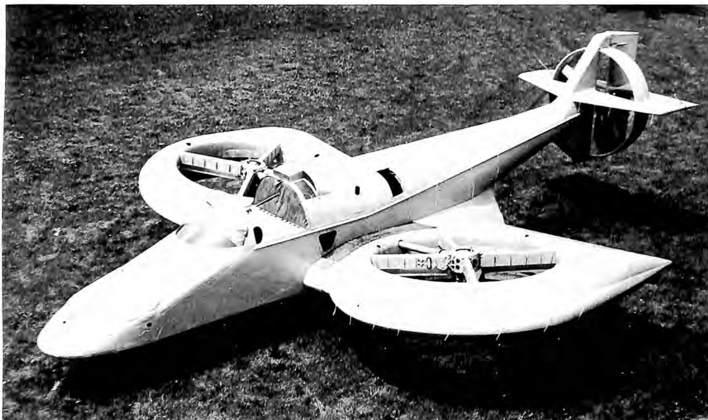
Vanguard refined the design of its "Omniplane," a turbine-powered "fan-in-wing" aircraft, and conducted full-scale wind tunnel tests.
