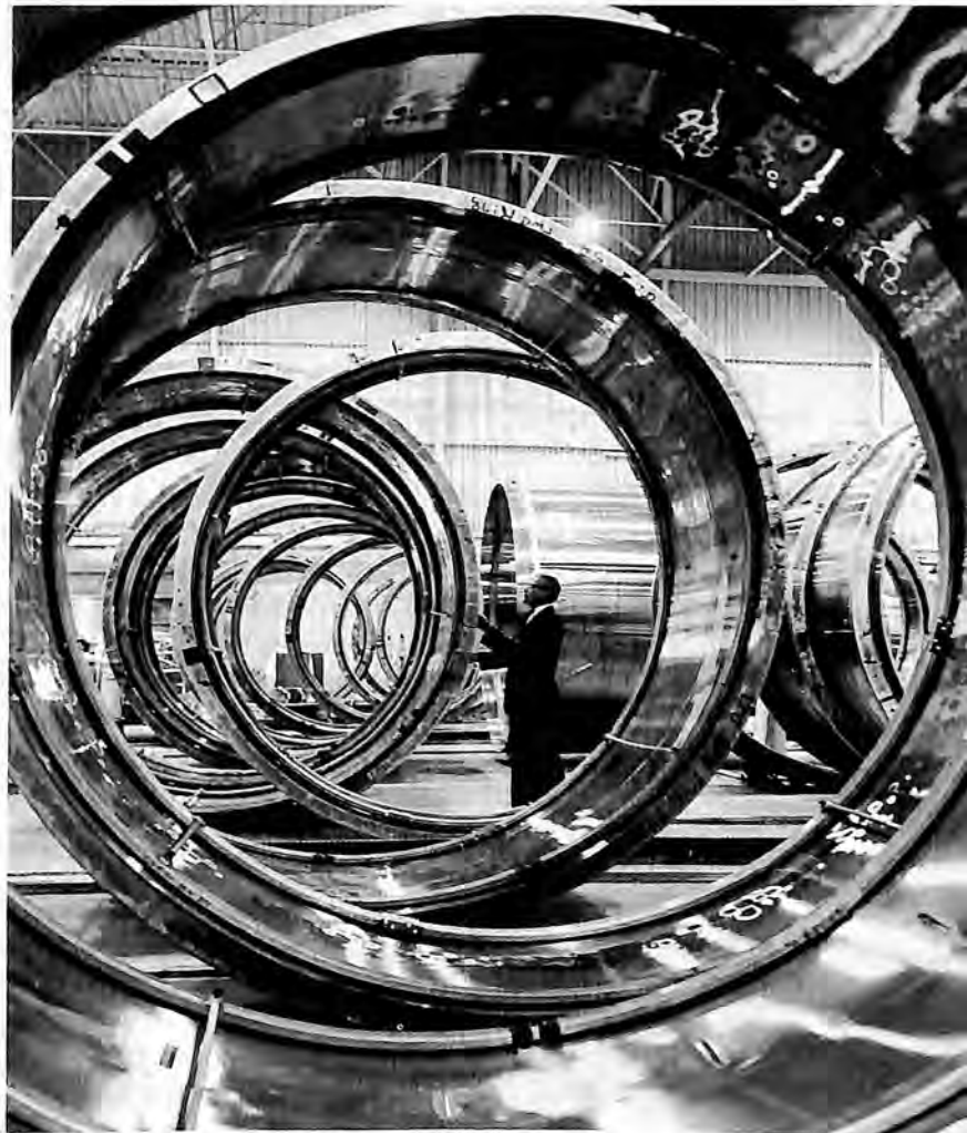
Stainless steel tank sections for Atlas await welding.
