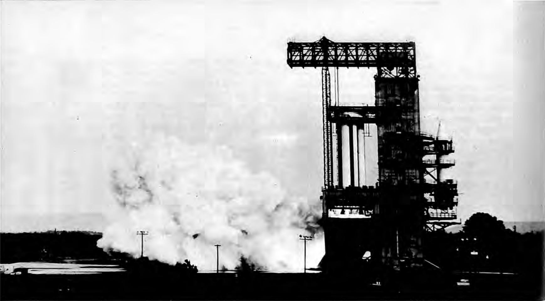
The eight-engine Saturn booster in static test at NASA's George C. Marshall Space Flight Center.
