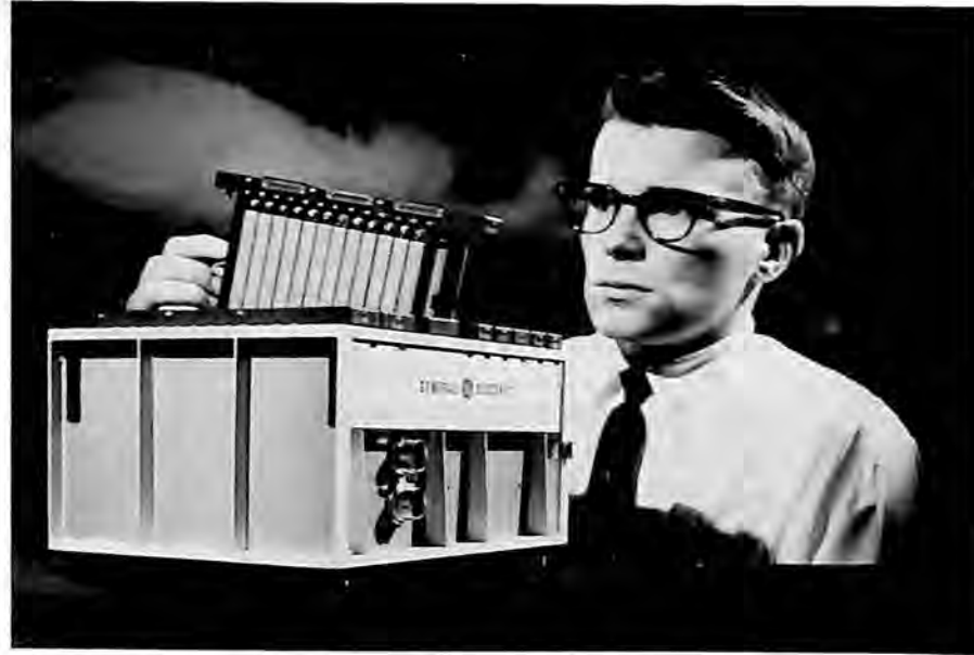
GE designed this 18-pound microelectronic computer, capable of performing more than 16,000 operations a second, for defense and other aerospace uses.
