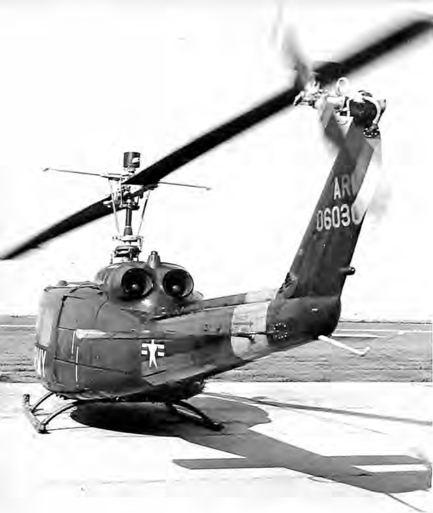
A modified Army UH-1D, built by Bell, was equipped with two free turbine engines for a flight program to test the concept of a twin-turbine power plant in a medium-size helicopter.
