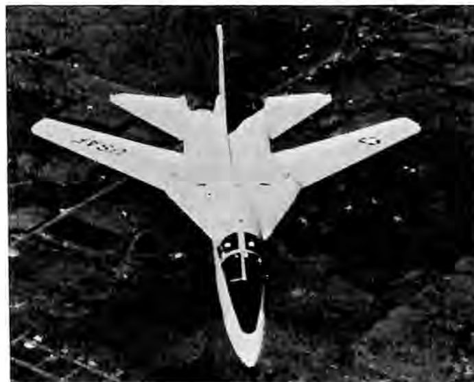
The trisonic F-111A successfully demonstrates its variable sweep wing.
