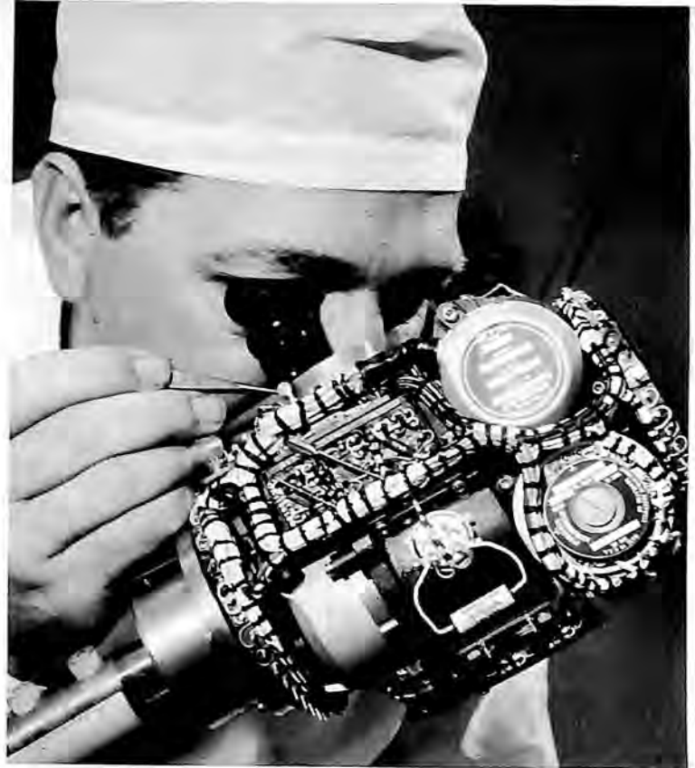
Heart of the guidance platform in the Gemini spacecraft is the azimuth block, here being adjusted by a Honeywell engineer.
