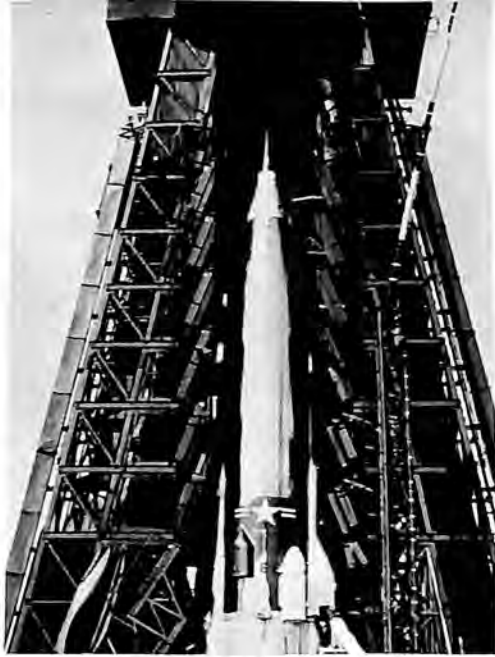
ABRES vehicle, a research tool in a program aimed at development of more effective ICBM nose cones, is readied for launch aboard Atlas.
