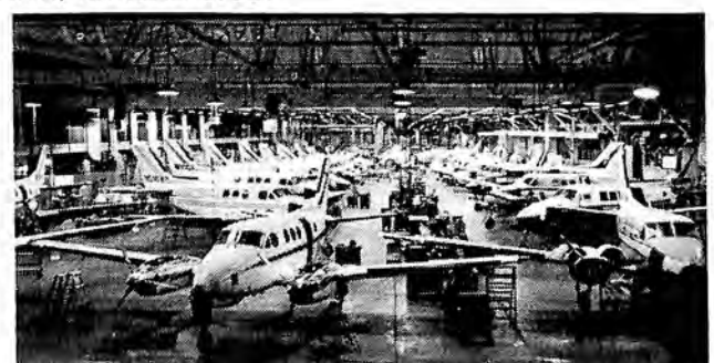
Part of the 1,230,000 square feet of production area at Beechcraft's Wichita Plant I. Shown in production are Beechcraft King Airliners, Queen Airliners and Super H18's.
