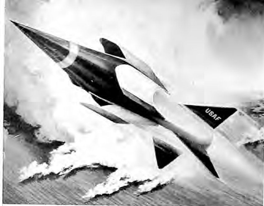
Artist's conception of a test vehicle for the Scramjet being developed by Marquardt.
