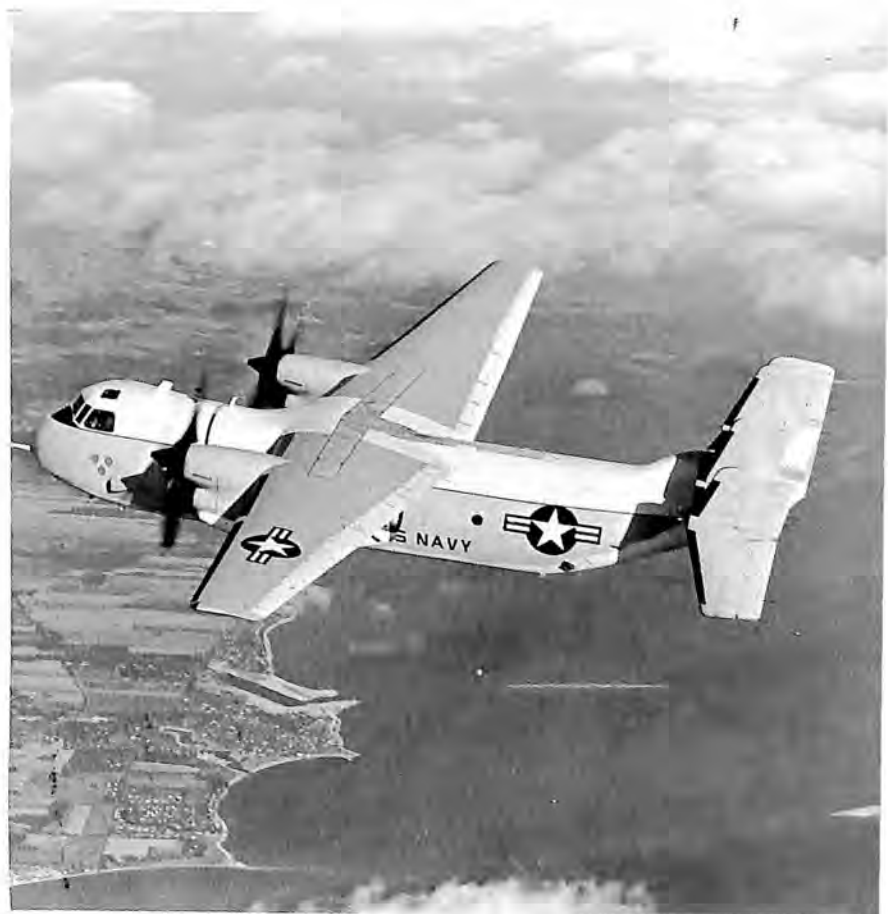
C-2A Greyhound was developed by Grumman to meet U. S. Navy requirements for an improved utility transport to deliver cargo and personnel to and from aircraft carriers at sea.
