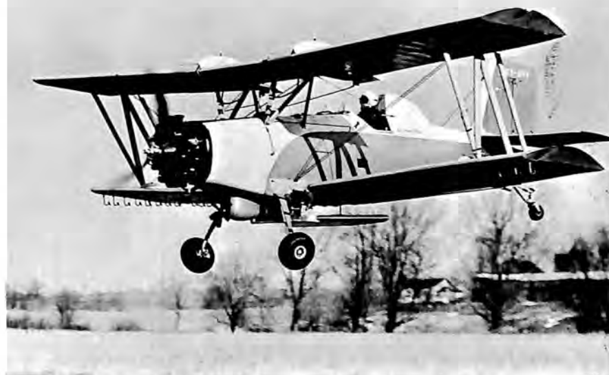
Grumman Ag-Cat is utilized for crop dusting, spraying, seeding and a host of other utility jobs.
