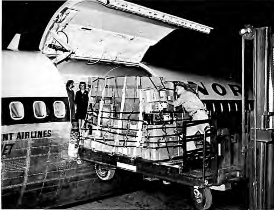
One of Northwest's 1965 re-equipment moves was acquisition of 5 707-320C convertible passenger/cargo airliners.
