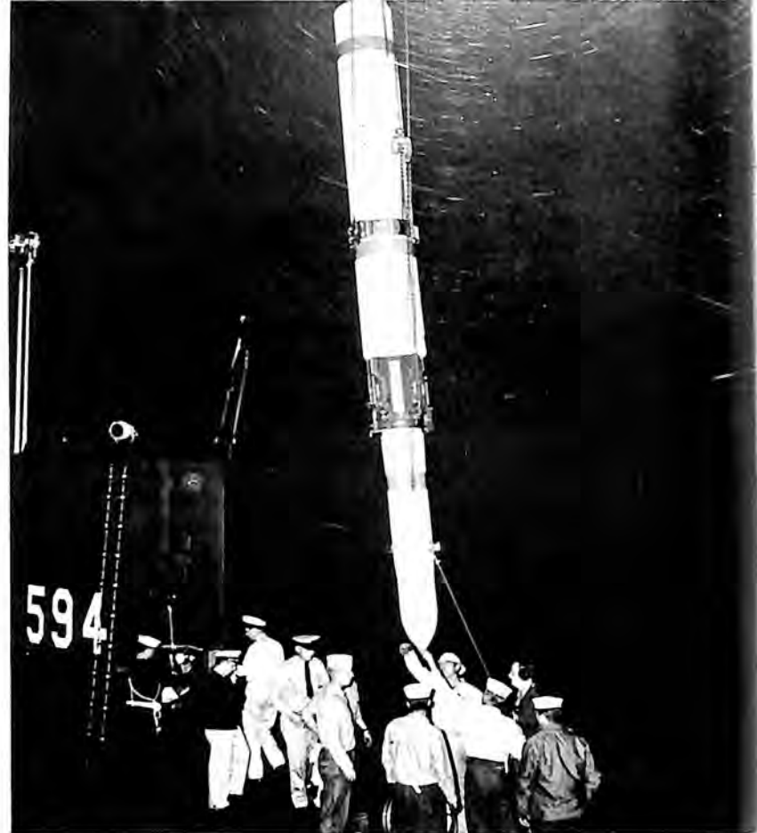
SUBROC missile built by Goodyear Aerospace Corporation hangs from crane during loading aboard submarine for Pacific tests. Missile is fired through conventional torpedo tube and travels through water and air to reach objective.
