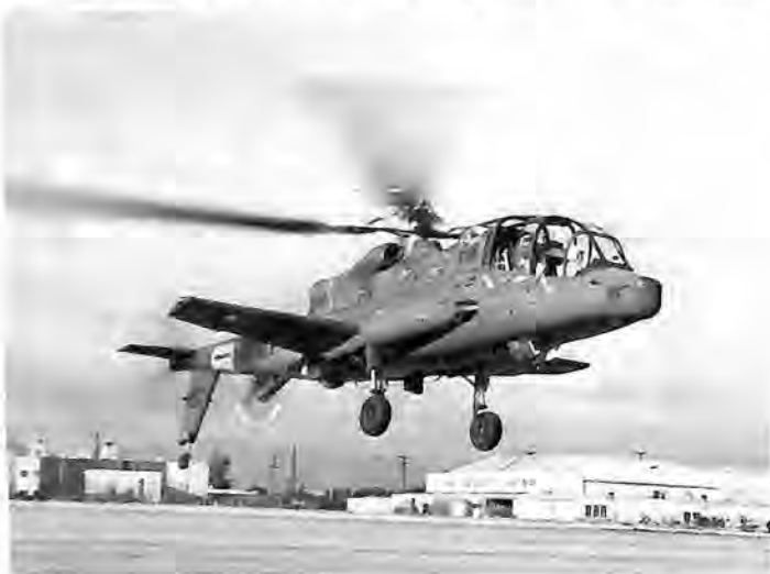
The Army's major aircraft development program involved the AH-56A Cheyenne, the first armed helicopter designed from inception to integrate vehicle, avionics, weapons and fire control.
