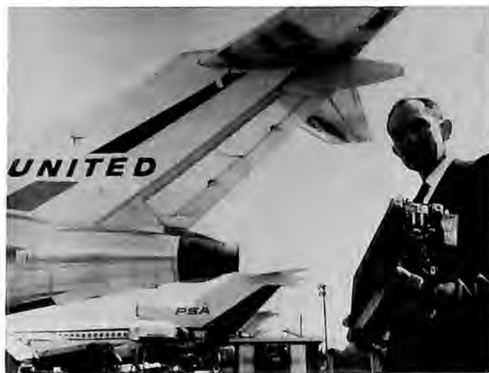
Honeywell's Aerospace Division started volume production of air data computers, such as the one displayed by field service engineer, designed for the Boeing 700 series transports.
