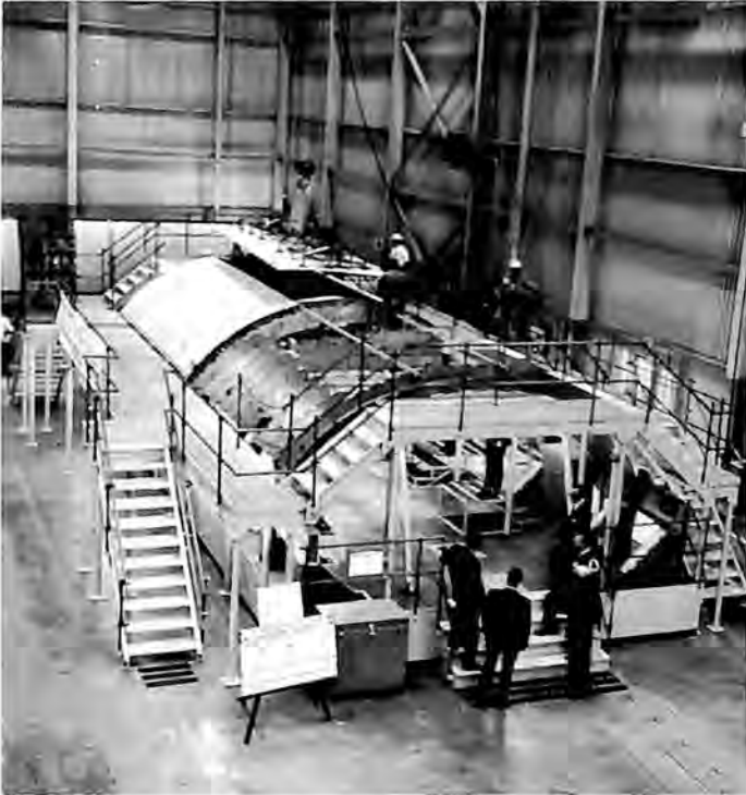
Northrop Corporation started fabrication of 153-foot passenger sections of the Boeing 747 jetliner.
