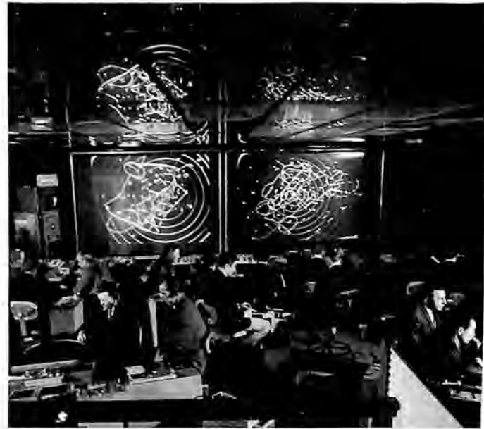
At its National Aviation Facilities Experimental Center, FAA was testing 9- by 12-foot large screen projection displays which provide a composite picture of radar/beacon video and computer-processed alphanumeric flight data for air traffic controllers.
