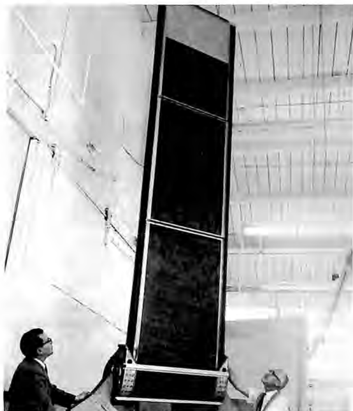
Ryan Aeronautical Company developed a deployable solar array for Jet Propulsion Laboratory's 1969 Mars probe.
