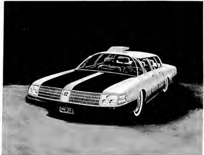
Fairchild Hiller's Republic Aviation Division developed the Safety Car, incorporating many of the safety features found in the cockpits of fighter aircraft, for the State of New York.
