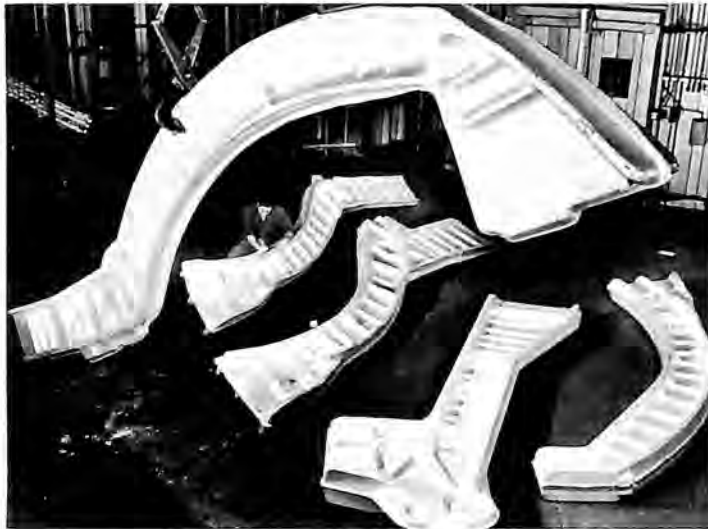
Alcoa was supplying huge aluminum forgings as structural elements of the USAF's Lockheed-Georgia C-5A transport.
