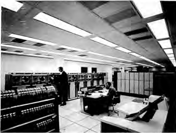
NASA's advanced computing capability for manned space missions was beefed up during 1967 with the completion of a UNIVAC 1108 real-time computer complex at the Manned Spacecraft Center in Houston.
