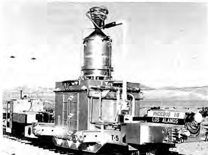
In February, a Phoebus 1B reactor was operated at design power of 1,500 megawatts for 30 minutes as part of the AEC/NASA Rover program for the development of nuclear-powered space rockets.
