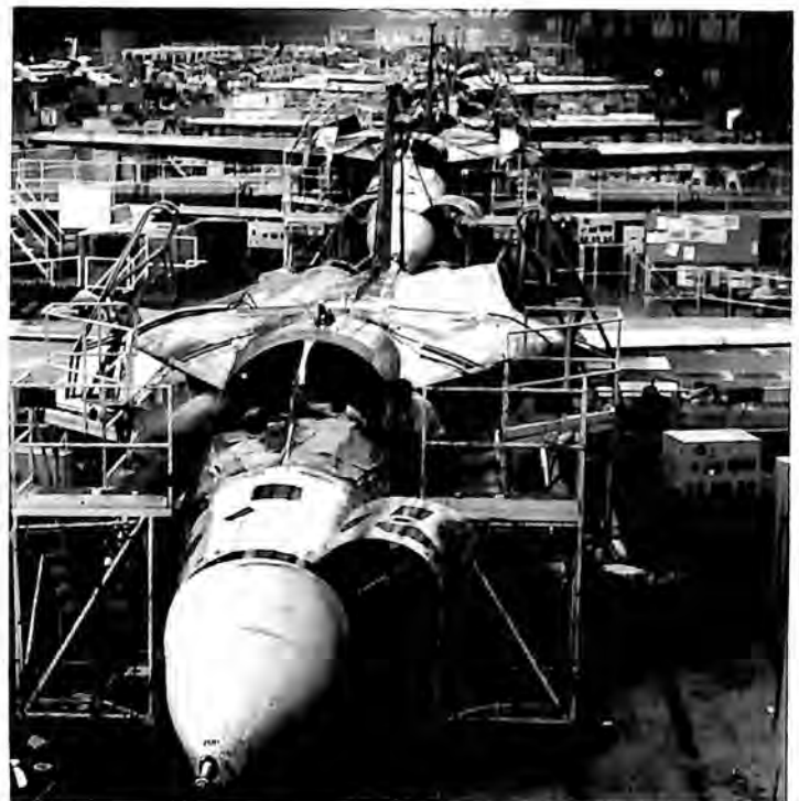
The F-111 production line at General Dynamics' Fort Worth division geared up to turn out 443 variable-sweep tactical and strategic aircraft for the U.S. Air Force, U.S. Navy, and Australia.
