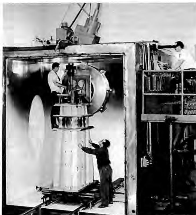
Aerojet-General installed the largest U.S. electron beam welding unit and vacuum chamber at Aerojet Downey's Fullerton, California, facility.
