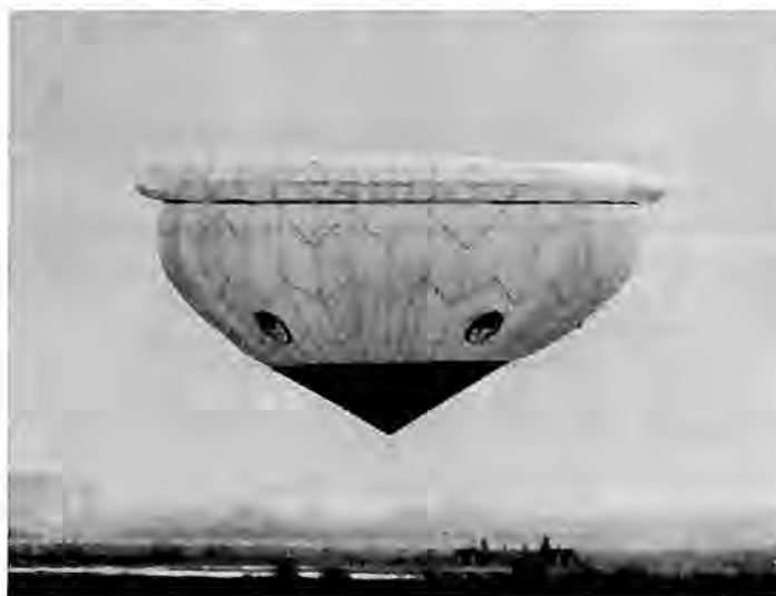
NASA tested this Goodyear-built 30-foot Ballute, an air-filled fabric bag with potential for slowing a spacecraft.
