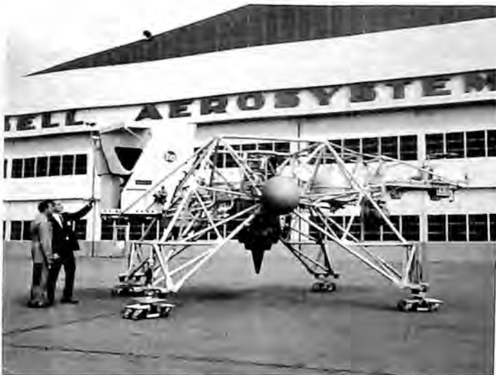
NASA accepted the first of 3 Lunar Landing Training Vehicles built by Bell Aerosystems.
