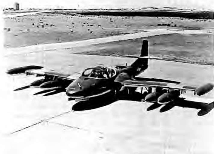
Cessna started production on an order for 39 A-37A attack aircraft and a later order for 127 A-37Bs. The craft are modified versions of the T-37 trainer.
