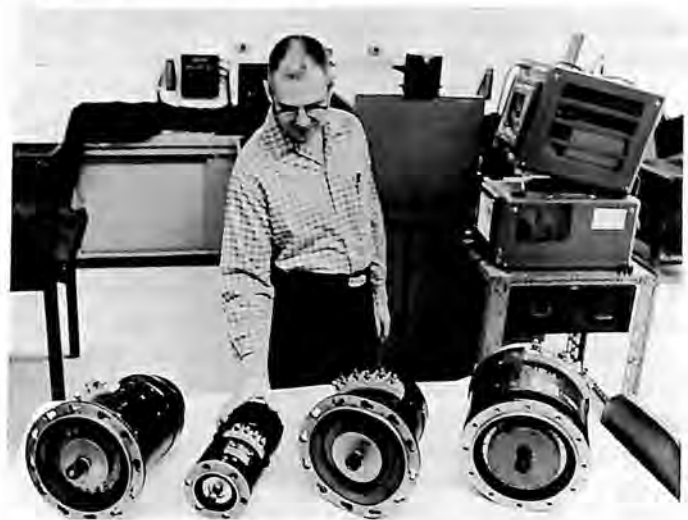
Test engineer handles new compact brushless generator developed by Bendix Electric Power Division for the Lockheed AH-56A helicopter. Generator is compared with conventional design (far left) of similar output.
