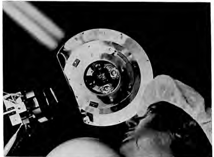
Hughes technician checks alpha-scattering device carried aboard the successful Surveyors 5 and 6, built by the company for NASA.
