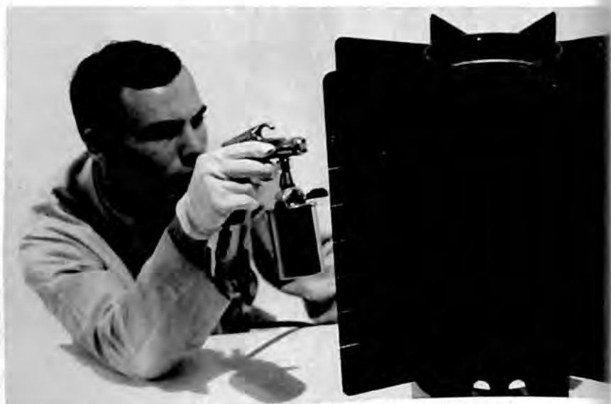
Beryllium structure built by Solar for lunar power system
