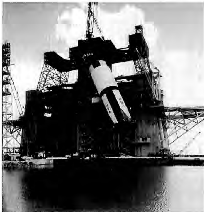
Saturn V first stage is lifted into test stand at the Mississippi Test Facility. GE provides NASA with operational support at the facility.
