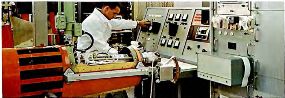
The never-ending search for highest reliability from all Beech-built products led to the design of this General Purpose Automatic Tester. It is shown here being applied to all functional areas, both electrical and mechanical, of an MQM-37A supersonic target missile produced by Beech for the U. S. Navy. The taped read-out will become a permanent record of the test, eliminating the chance of human error in reading, evaluating and recording.
