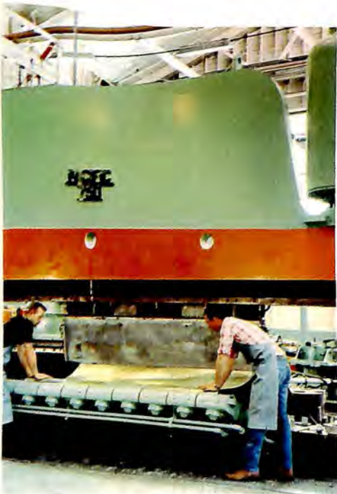
Forming of sheet metal and extrusions is an important requirement of any aerospace facility. At Beech, forming capabilities have been developed to handle complex jobs in a wide range of materials.
