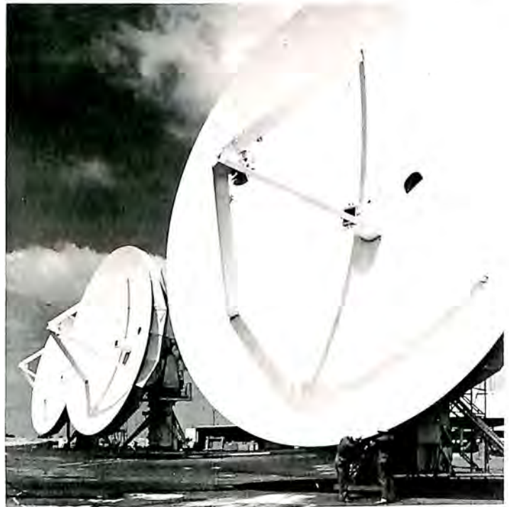
Hughes Aircraft technicians make final test of a Mark 1B satellite communications ground-link terminal at the company's Fullerton plant, where 14 of the stations were built.
