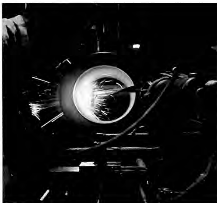
Inner worn surface of a T56 compressor section is restored at Aerodex with oxyacetylene torch "metal spray" technique.
