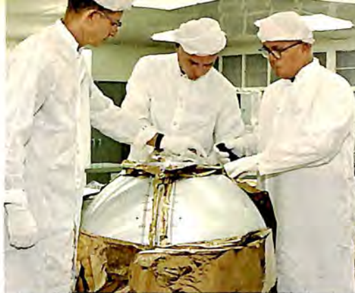
The design and fabrication of pressure vessels and cryogenic storage systems are highly developed at Beech. This cryogenic storage system was designed and built by Beech under contract with North American. It was the first of 13 major subsystems aboard the Apollo spacecraft to be man-rated by NASA.
