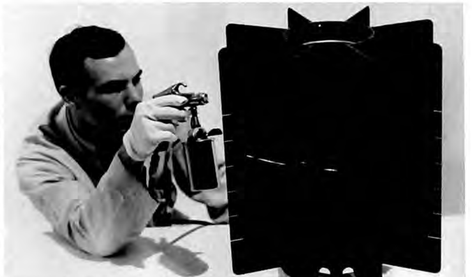
Beryllium structure built by Solar for lunar power system
