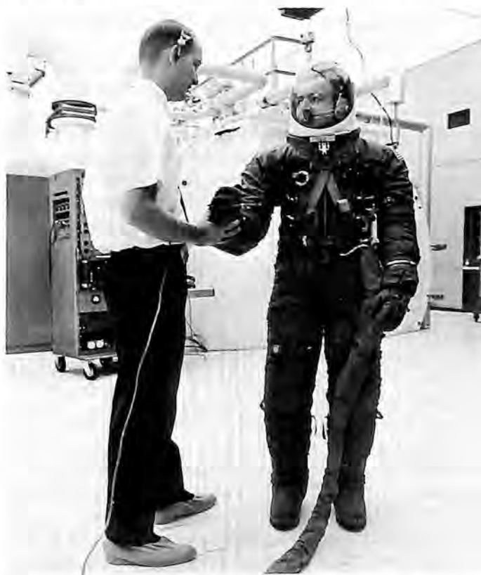
Hamilton Standard was developing an advanced space suit for future missions that offers considerably greater mobility than existing pressure suits.
