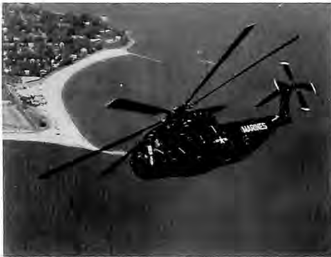
The Marine Corps CH-53A helicopter performed a series of loops and rolls, unprecedented maneuvers for an aircraft of its size, in a joint Naval Air Systems Command/Sikorsky flight test program to investigate rotor system dynamics and maneuverability.
