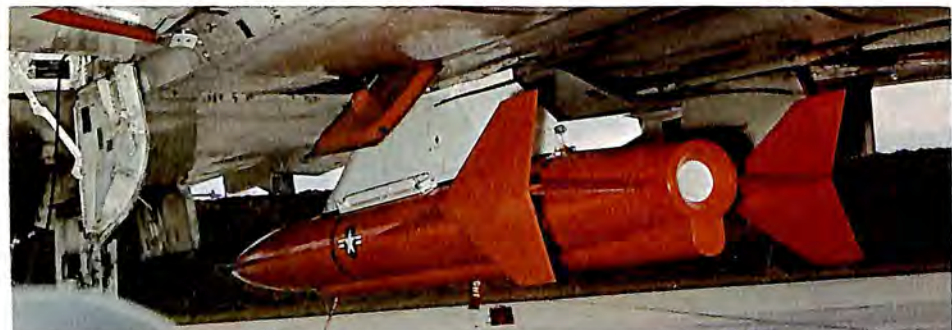
Sandpiper, the first maneuverable rocket-powered supersonic target missile has successfully completed first tests for the U. S. Air Force. The test vehicle was a modified Beech AQM-37A missile powered by the nation's first operationally-designed hybrid rocket engine. The engine, developed and produced by United Technology Center, uses both solid and liquid fuels and has sustained flight of Sandpiper during tests for an extraordinary full five minutes.
