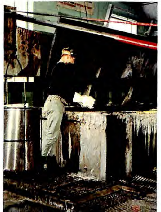
Heat-treating facilities include six aluminum heat-treat furnaces with capabilities of drop quenching and handling parts up to 9½ feet high, 8½ feet wide, and 24½ feet long. The facilities are furnished with aging furnaces having inside dimensions up to 8 feet wide, 6 feet high and 40 feet long.
