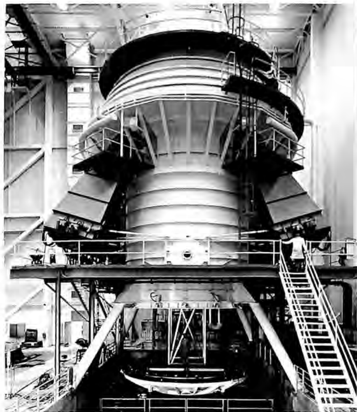
TRW Systems Group placed in operation at its Redondo Beach, California, facility this $2,400,000 space simulation chamber.
