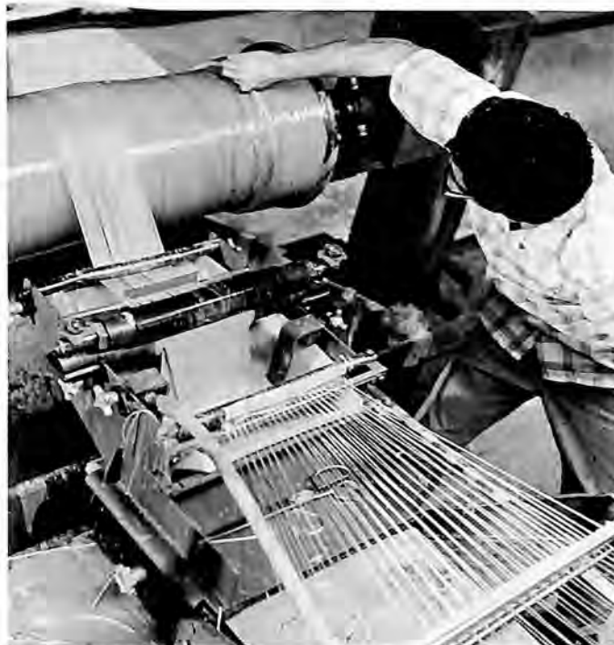
United Technology Center started manufacture of Techite, a reinforced plastic mortar pipe for use in fluid conveyance systems.
