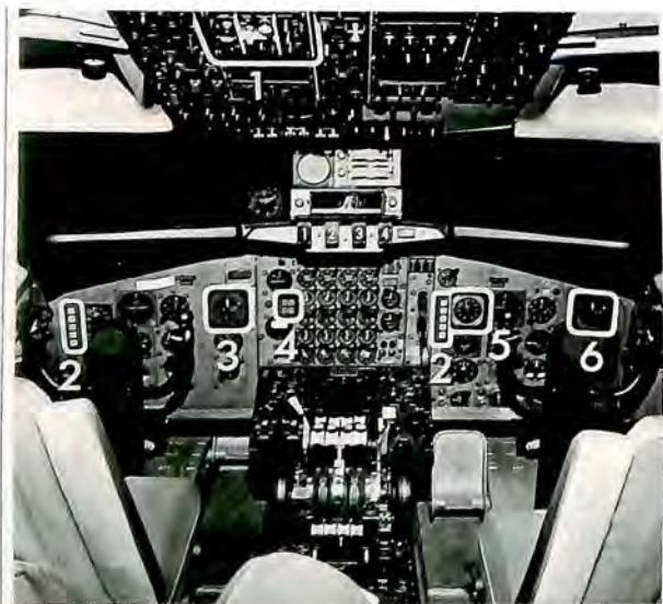
1. APPROACH CONTROL PANEL 2. APPROACH PROGRESS DISPLAY 3. LOW RANGE RADIO ALTIMETER No. 1 4. AUTOPILOT & AUTO THROTTLE WARNING LIGHTS 5. AIRSPEED IND. (AUTO THROTTLE CONTROL) 6. LOW RANGE RADIO ALTIMETER No. 2
