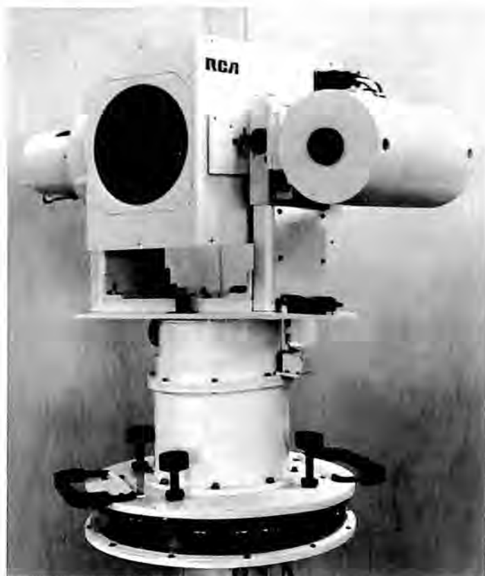
RCA's Defense Electronic Products developed under NASA contract a laser tracking and ranging unit capable of continuously monitoring the position of an astronaut as he moves about the lunar surface.
