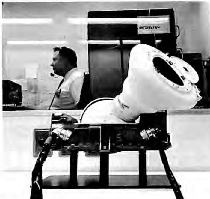
Kollsman star trackers, 6 of which help position the Orbiting Astronomical Observatory, demonstrated their reliability by completing a year of operation aboard OAO-2. In photo, one of the trackers is checked out under clean-room conditions.
