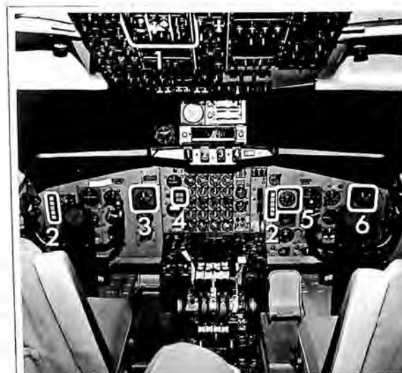
1. APPROACH CONTROL PANEL 5. AIRSPEED IND. (AUTO THROTTLE CONTROL) 2. APPROACH PROGRESS DISPLAY 6. LOW RANGE RADIO ALTIMETER No. 2 3. LOW RANGE RADIO ALTIMETER No. 1 4. AIRCRAFT 4. WING TIP WARNING LIGHTS
