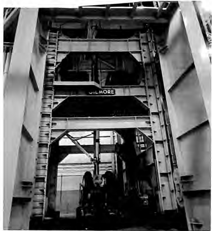
Pneumo Dynamics Corporation's Cleveland Pneumatic completed work on its $20,000,000 "big gear" complex. One of many new facilities is this drop test tower being used for check-out of Boeing 747 wing gears.
