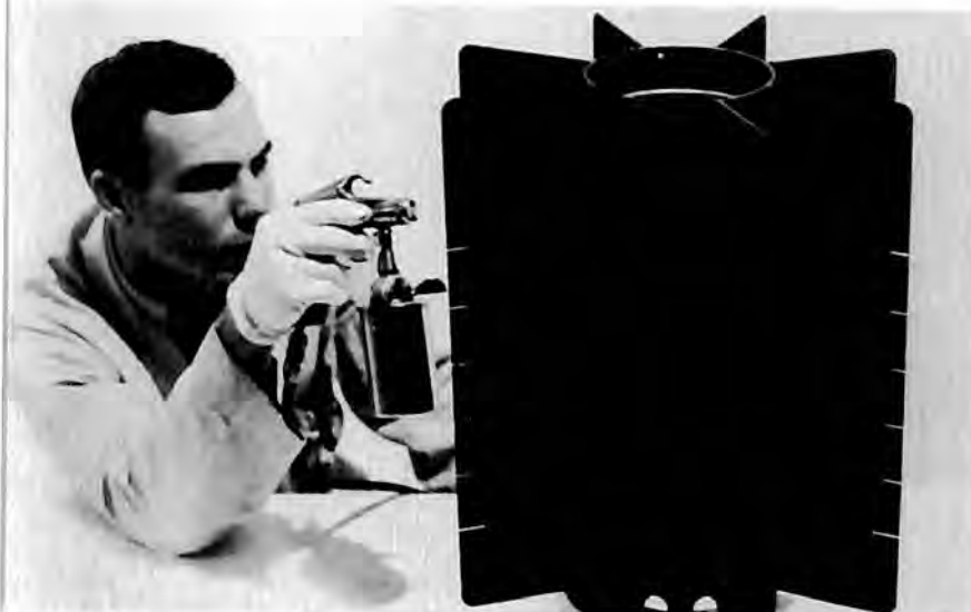
Beryllium structure built by Solar for SNAP 27 lunar power system
