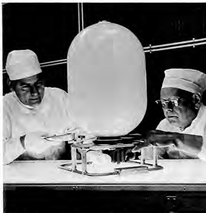
In a dust-free clean room, Bell Aerospace technicians check an inner bladder of an Apollo positive expulsion propellant tank. Bell provides 31 such tanks for each Apollo spacecraft.
