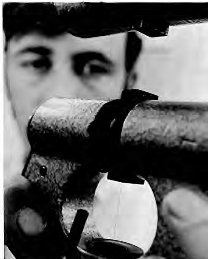
A Hamilton Standard technician puts an ultrathin boron filament from a production run through a tensile test. The filament, the reinforcement element in new composite structures, has an ultimate tensile strength of 400,000 pounds per square inch.
