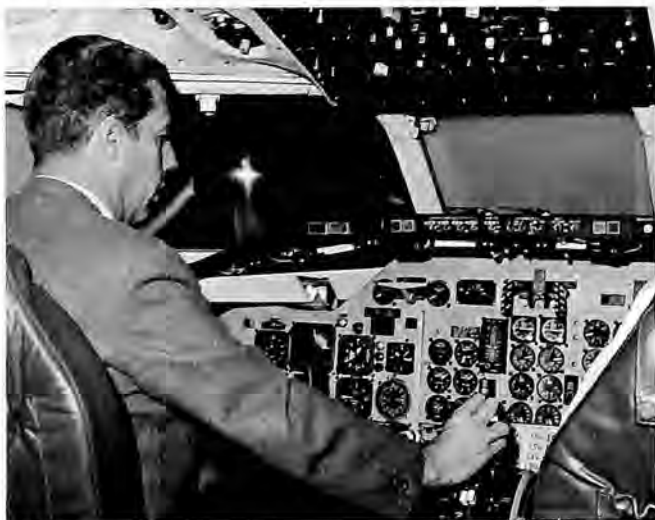
Delta Air Lines became the first airline to order and use the Link VAMP (Visual Anamorphic Motion Picture) system in its DC-9 simulator, here being flown by Captain Charles Green, system manager-flight training.
