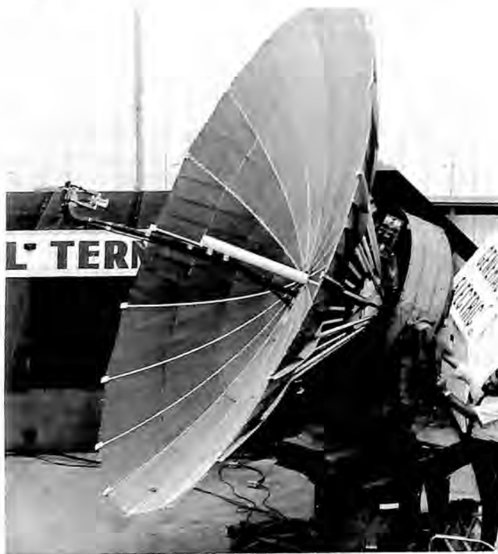
A key element in the transmission of Apollo recovery TV coverage was this paraboloid antenna, built by General Electric's Space Division, which folds like an umbrella for shipment.
