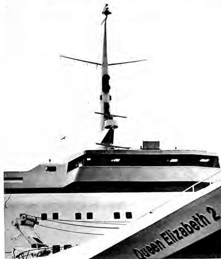
ITT Aerospace/Optical Division developed the unique conical antenna, high atop the mast of the Queen Elizabeth 2 , which permits the liner to receive satellite signals for precise position location data.
