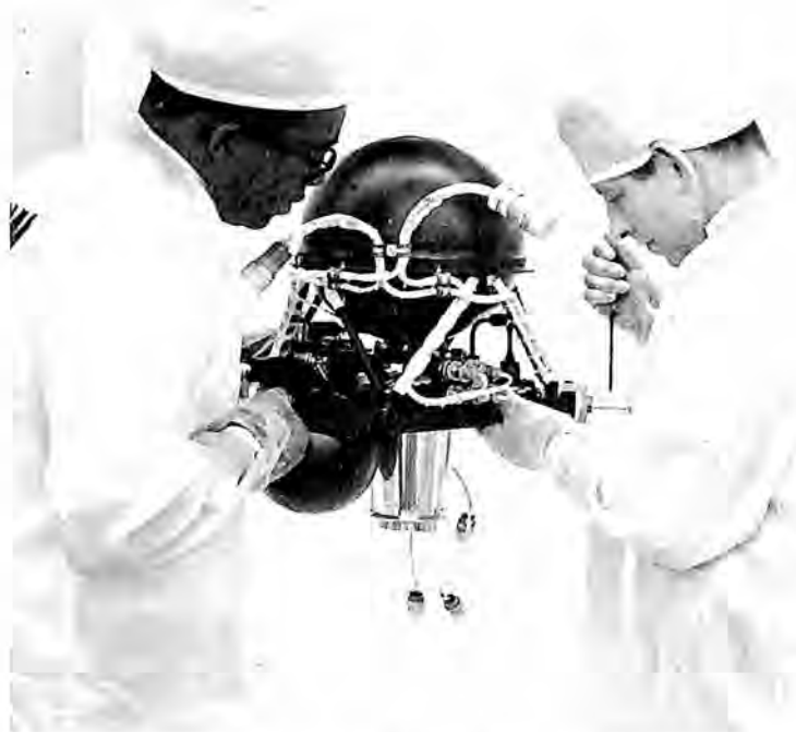
Technicians of TRW Inc. check over a unit of the company's hydrazine propulsion system, which performed flawlessly on the 1969 Mars flights of Mariners 6 and 7.
