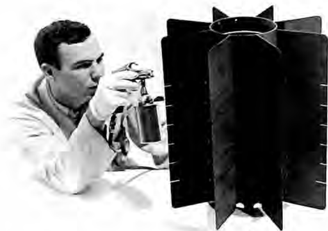
A Solar technician sprays coating on a beryllium container for the SNAP-27 nuclear auxiliary power system first used on Apollo 12. Solar manufactures the containers at San Diego.
