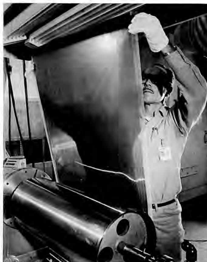
Northrop Corporation was conducting advanced research toward development of production techniques for the application of boron and graphite composites to future aircraft. In photo, technician unrolls a sheet of boron composite material.
