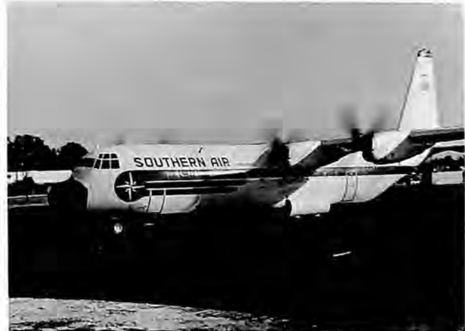
Southern Air Transport introduced into service the Lockheed-Georgia L-100-20 stretched Hercules transport, capable of carrying outsize cargo and payloads up to 48,000 pounds.
