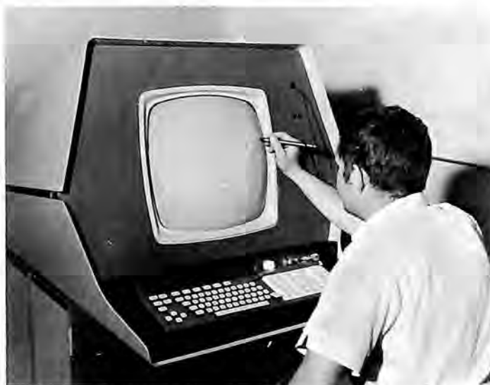
Sperry Rand's Univac Division delivered a UNIVAC 1557/1558 Graphic Display Subsystem to the Army's Safeguard System Evaluation Agency (SAFSEA). Tied into a UNIVAC 1108 computer, the subsystem is used to display information needed in evaluating critical aspects of the Safeguard ballistic missile defense system.
