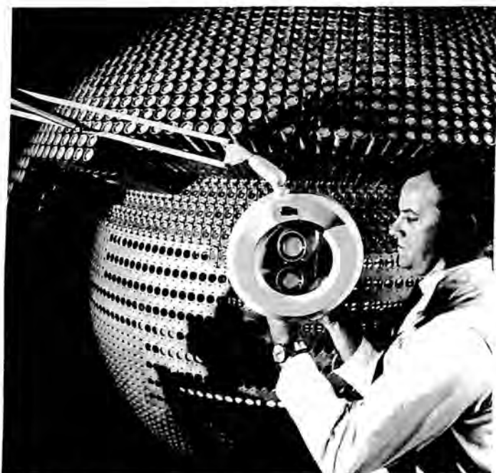
A Hughes Aircraft technician adjusts an antenna, one of several in the 1/10-scale prototype of ADAR, a new phased-array radar and the most powerful yet built by Hughes, a pioneer in the field.
