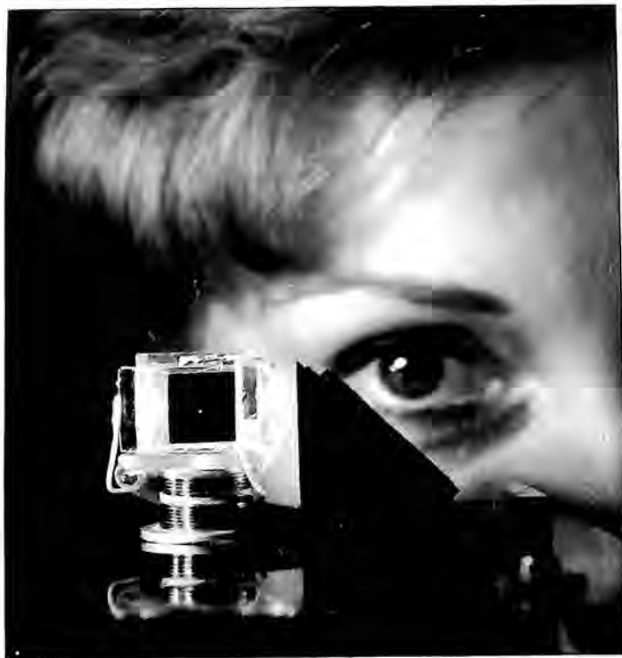
Martin Marietta's Orlando Division was conducting a research program involving the application of "particle reference" devices to inertial guidance equipment. These devices employ a tiny glass ball suspended in an electrical field to provide inertial reference for new types of accelerometers, gyroscopes, and gravity meters.
