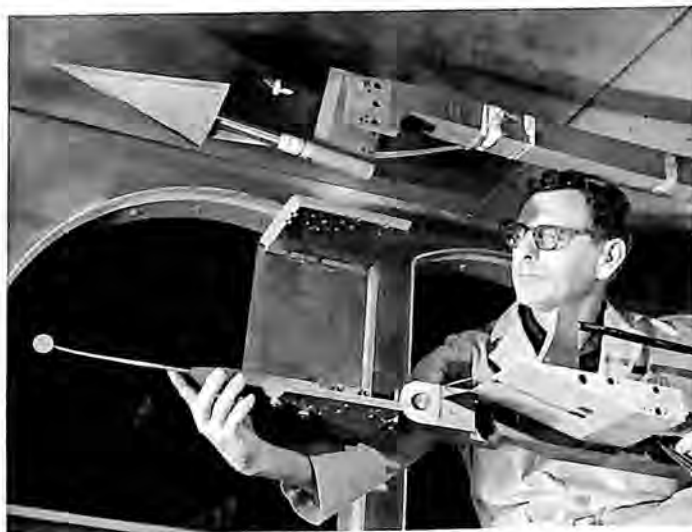
At Arnold Engineering Development Center, the Air Force's Systems Command was studying the feasibility of reducing sonic boom severity without losing aircraft performance.
