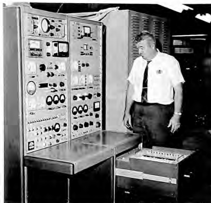
Bendix Electric Power Division's test system for checking electric systems used in 7 different aircraft includes this test console. The open drawer contains a program recorder which prints out test characteristics.
