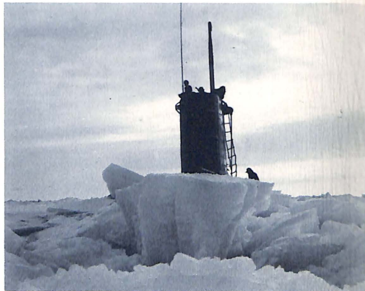
Rugged USS SARGO penetrates 48 inches of ice in surfacing operation. Navy conducts many experiments in Polar regions.
