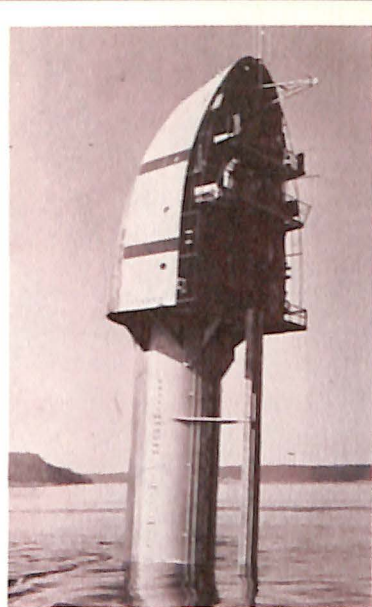
FLIP (Floating Instrument Platform) ship is readied for ocean tests. Note men on bow with ship at the vertical.
