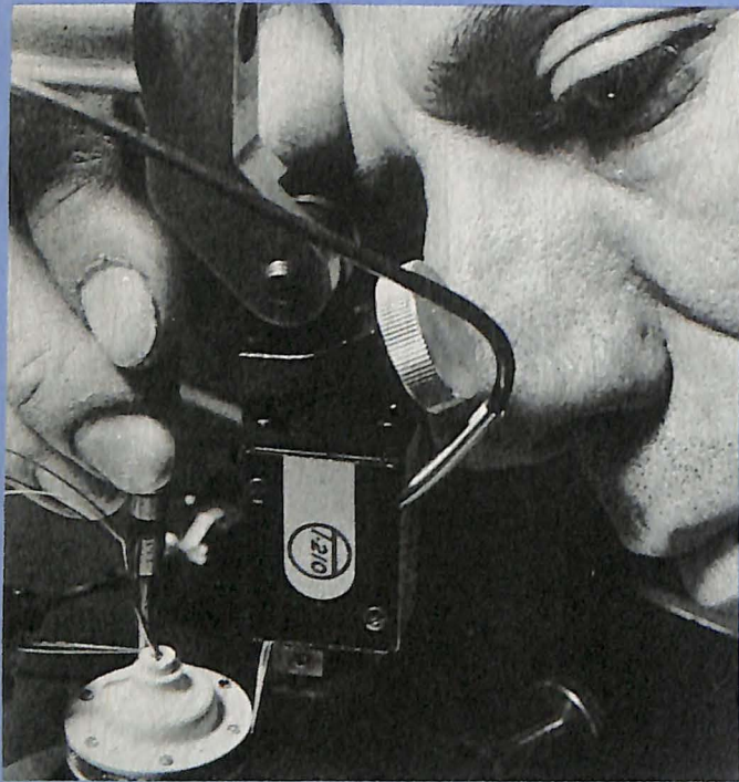
An electronic measuring device, calibrated in millionths of an inch, checks tolerances on a gyroscope's spin motor.
