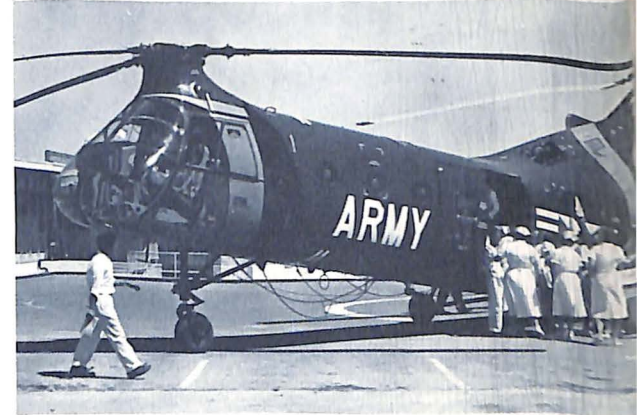
This huge helicopter can transport 67 passengers in the attached pod. The pod could be equipped as an emergency hospital and transported quickly to disaster areas.
