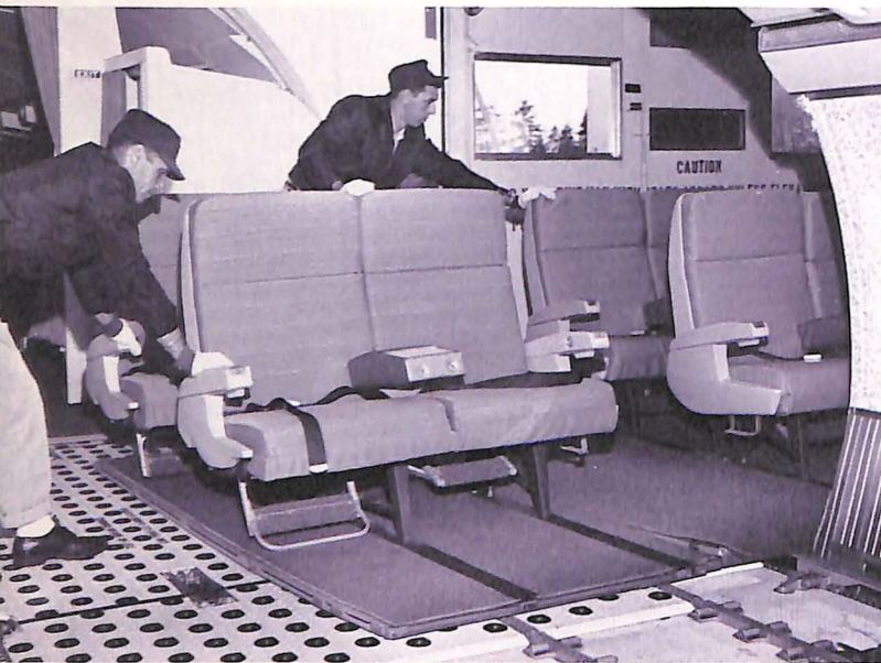
Boeing 727QC (quick change) crew members move seat and galley pallets to cargo door (above). Cleared of seat and galley pallets, cargo pallets are loaded (below). Change to cargo configuration has been made in eight minutes, increases utilization and earning power of the aircraft.
