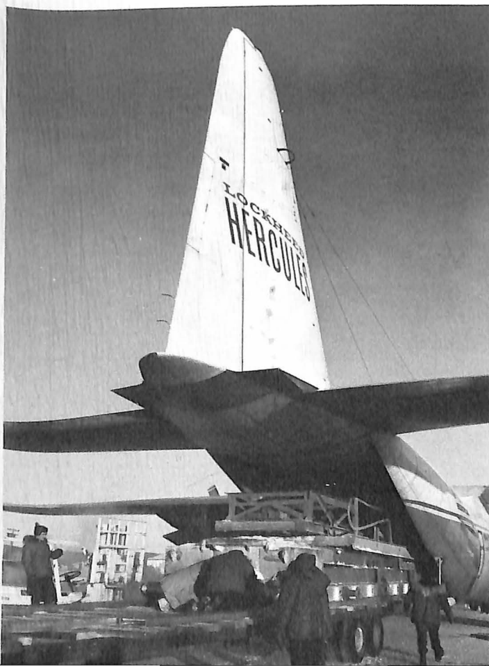
Twenty-ton drill rig is loaded aboard a Lockheed L382 Hercules commercial transport at Fairbanks, Alaska, for a flight across the Brooks Mountain range.
