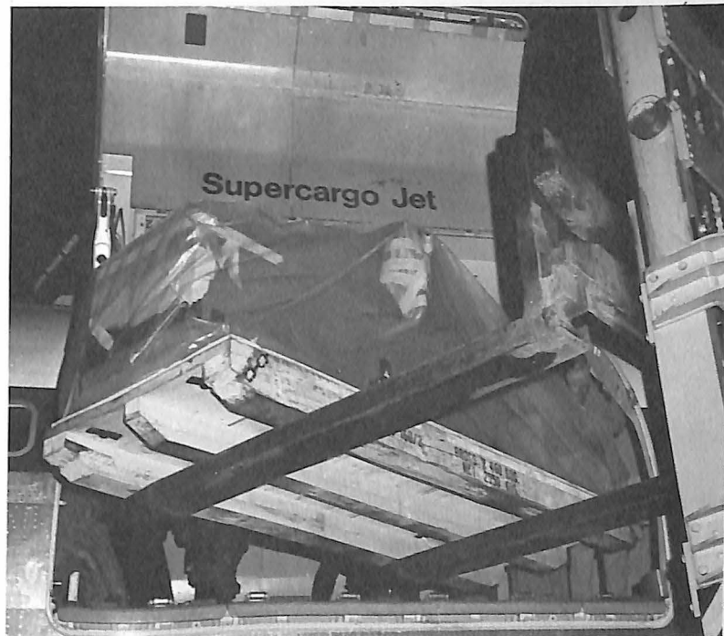
Under plastic wraps, profile borer unit mounted on skid is carefully hoisted through front cargo door of Lufthansa jet freighter during night loading at Stuttgart.
