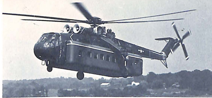
This huge helicopter can transport 67 passengers in the attached pod. The pod could be equipped as an emergency hospital and transported quickly to disaster areas.
