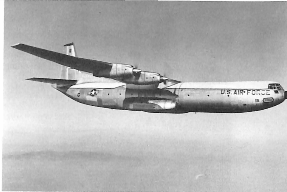
Douglas C-133 Cargomaster, largest operational aircraft in the Air Force, can take 100,000 pounds of cargo in its 90-foot cargo hold.
