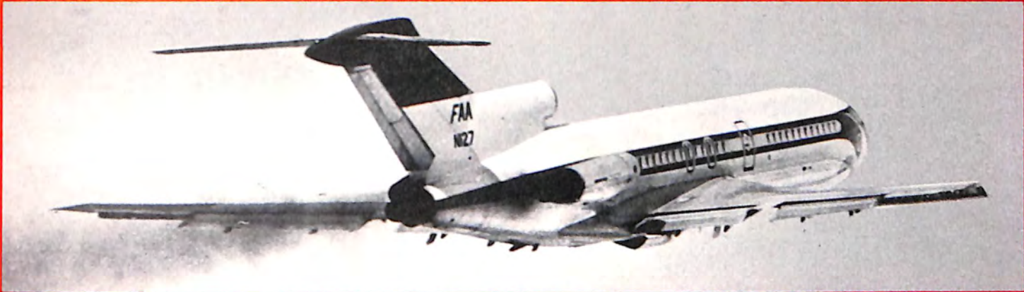
New technology turbine engines on the 747 show no smoke emission at takeoff. The aircraft in lower photo shows emission; however, the engines are being retrofitted with a new combustor which eliminates smoke.
