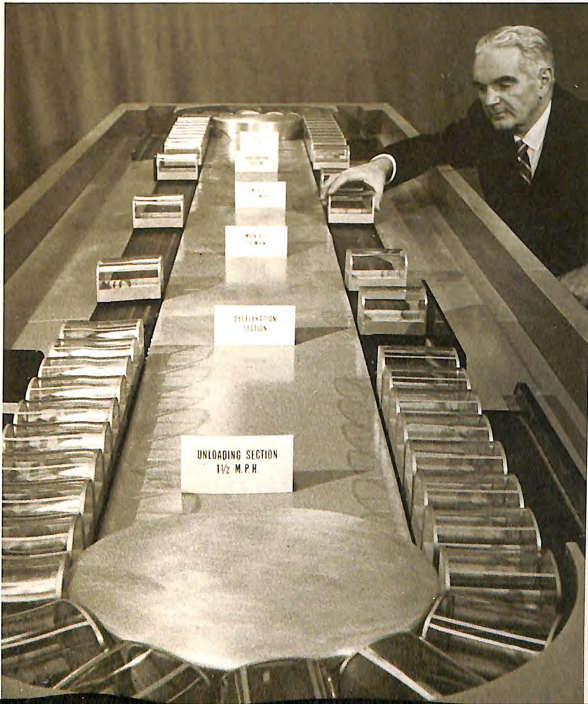
Demonstration model of Goodyear's Carveyor system. Passengers board cars from platform moving at 1½ mph, matching the speed of the cars. As cars leave station they pass over wheels that increase speed to 15 mph; another set of wheels decelerates inbound cars for passenger exit onto moving ramp.
