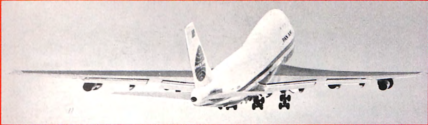
New technology turbine engines on the 747 show no smoke emission at takeoff. The aircraft in lower photo shows emission; however, the engines are being retrofitted with a new combustor which eliminates smoke.
