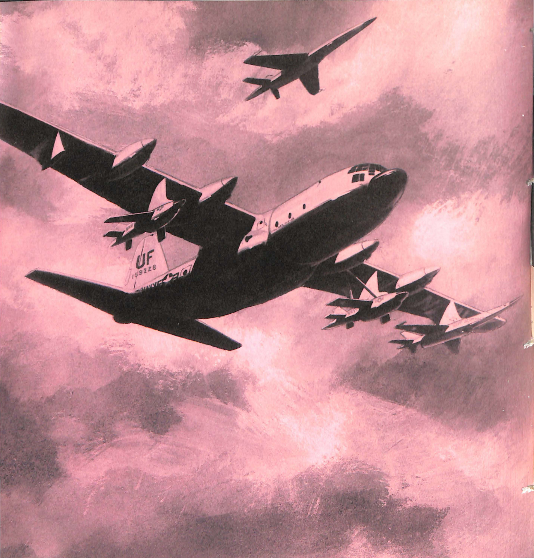
A Lockheed C-130 Hercules launches one of four pylon-mounted Teledyne Ryan Firebee RPVs. The National Aeronautics and Space Administration recently requested industry proposals for a study on civil uses of RPVs. (See A New Breed of Super Servants: Remotely Piloted Vehicles , p. 12).
