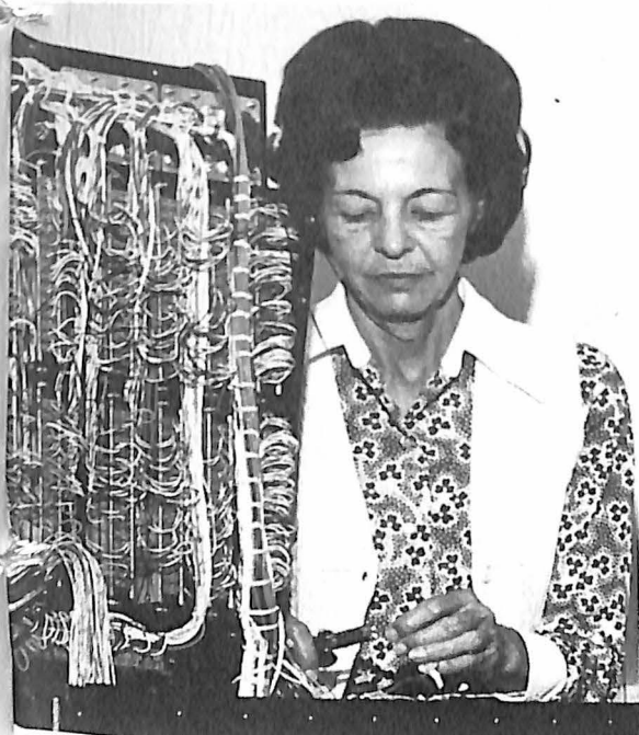
Another interesting RPV development is the completely de-manned aerial target for training pilots in air-to-air combat. The Sperry Rand Corporation has developed an electronic control package that can be mounted in a Convair Delta Dart F-102 which can be put through all paces of aerial combat and flown back to a smooth landing by the ground controller. Betty Schubert finishes wiring the pilot's "stand-in."
