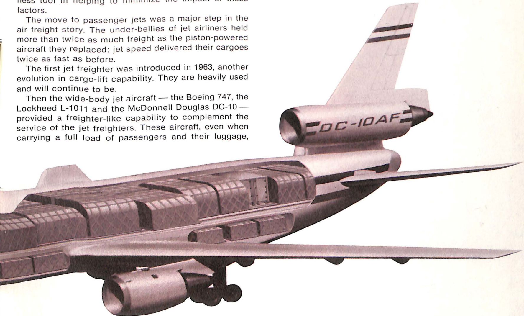
McDonnell Douglas DC-10 All Freighter is shown in an artist's conception. This version features two cargo decks with powered loading systems and large cargo doors.
