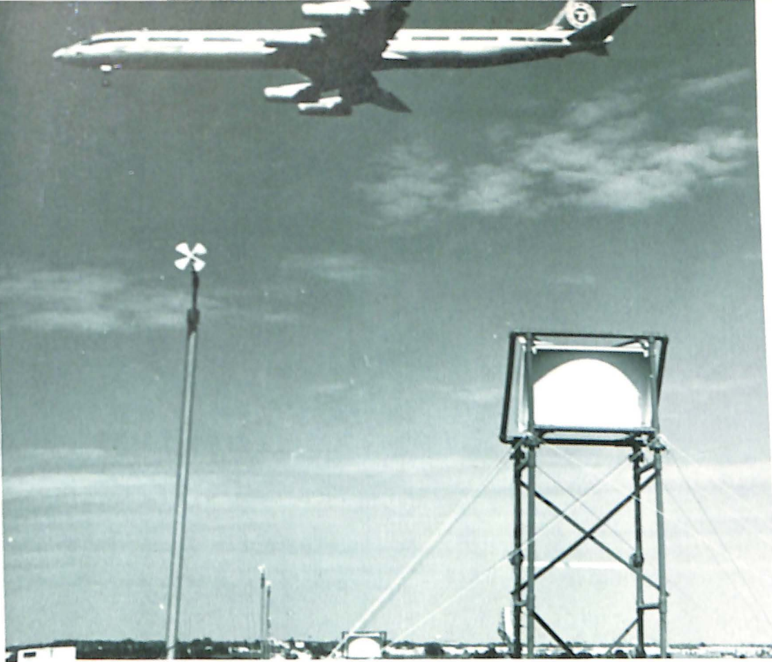
Trailing wake vortices generated by large aircraft present a hazard to following aircraft during approach and landing. Shown here is the instrumentation used to develop a wake vortex avoidance system.
