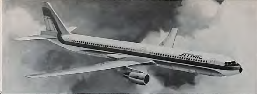
10. McDonnell Douglas ATMR . The projected Advanced Technology Medium Range twinjet is aimed primarily at airline regional routes. Its design is based on an advanced supercritical wing and the airplane would also have the latest in propulsion systems for reduced fuel consumption and lower exhaust emissions. In various seating configurations, it could accommodate from 166 to 200 passengers.
