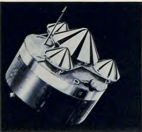
In the Pioneer Venus project, NASA will begin an intensive study of the planet Venus in 1978 with two separately-launched spacecraft. The one shown is the multiprobe bus, which will carry four probes that will descend through Venus' cloud cover and sample the atmosphere. The other spacecraft will report data while orbiting the planet for a year.
