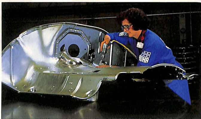
Rohr Industries made first deliveries of a superplastically formed heat shield for the General Electric CF6-80C2 engine.
