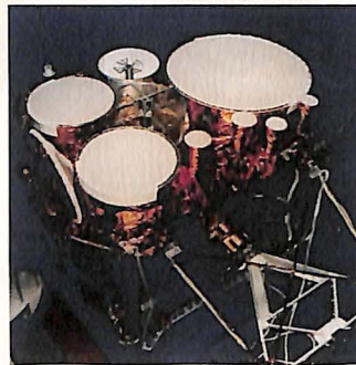
Among military space systems in development was General Electric's Defense Satellite Communications System (DSCS); here a DSCS III satellite is readied for solar simulator testing.
