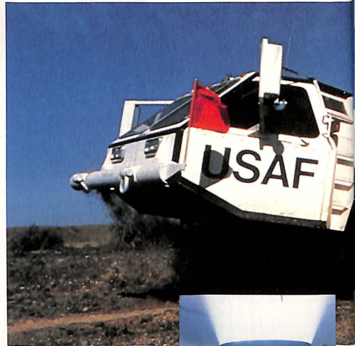
The Hard Mobile Launcher, developed by Boeing Aerospace and Loral Defense Systems for hauling and launching the USAF's Small ICBM, passed initial mobility tests in the summer.
