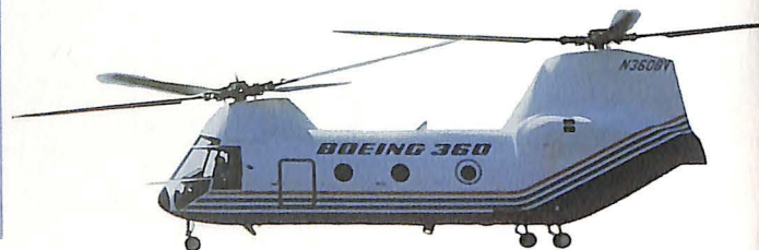
In June, Boeing Helicopter began a flight test program with its Model 360 Advanced Technology Demonstrator.
