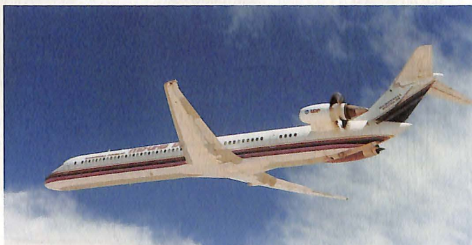
McDonnell Douglas flight tested an MD-80 transport powered by a General Electric UDF propfan. The company planned early 1990s introduction of propfan-powered airliners.
