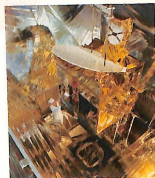
Shown being readied for test in a thermal-vacuum chamber is the GE Astro-Space GSTAR-III communications satellite, to be launched in 1988.
