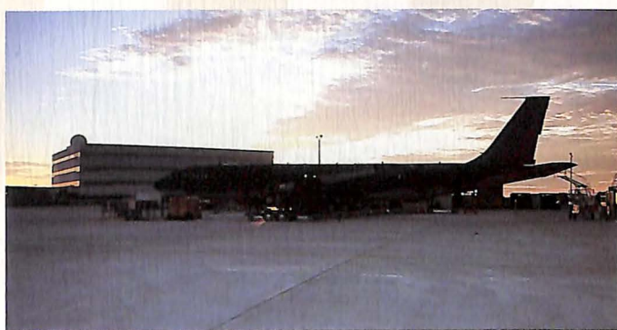
This modified Boeing 707 houses the airborne portion of the Joint STARS system being developed by a Grumman-led industry team for the Air Force and Army; it is a battle management system designed to detect, locate, classify and track large numbers of targets.
