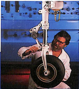
Colt Industries' Menasco Inc. teamed with Grumman Corporation to develop the JumpStrut advanced landing gear designed to reduce takeoff roll by up to 60 percent.
