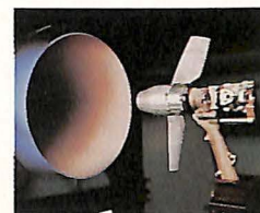
In development by Sundstrand Corporation in 1990 was the Ram Air Turbine for the USAF's C-17 airlifter. The power turbine is shown undergoing test in Sundstrand's wind tunnel facility.
