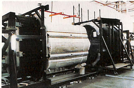
In research for the National Aero-Space Plane (NASP) program, Textron Specialty Metals developed a NASP fuselage assembly made of silicon carbide reinforced titanium.
