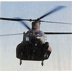
In June Boeing Defense & Space Group's Helicopter Division started flight tests of the MH-47E, a new member of the Chinook family designed for use by the Army's Special Operations Aircraft Regiment.
