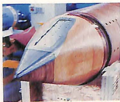
The January flight of the Army/McDonnell Douglas HEDI space interceptor demonstrated Aerojet's innovative platelet technology for reducing the 3,500-degree heat of hypersonic flight to a condition approaching room temperature.
