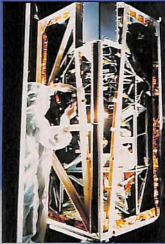
Martin Marietta Astronautics Group provided the Faint Object Spectrograph for the Hubble Space Telescope, which was Shuttle-launched in April.
