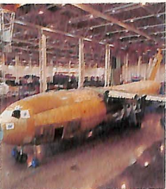
(Above) In July the first Air Force/McDonnell Douglas C-17 airlifter moved out of the automated major join tool to continue through the production line on its landing gear, on schedule for assembly completion by year-end. Artist's concept is at right.
