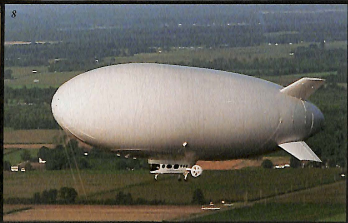
8. The Westinghouse Sentinel 1000 non-rigid airship made its first flight on June 26. It is a half-scale version of the Sentinel 5000 surveillance airship being developed under the DoD Air Defense Initiative program.
