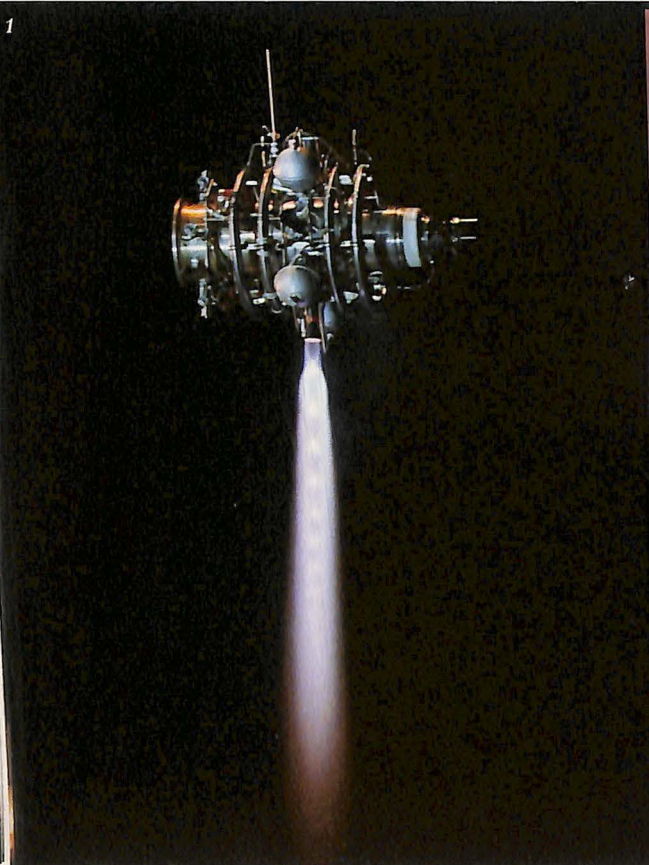
1. The Rockwell-developed LEAP III Lightweight ExoAtmospheric Projectile (shown) and the Hughes LEAP II successfully passed initial hovering tests and were slated for 1992-93 space tests. The space target acquisition systems are part of the Strategic Defense Initiative.
