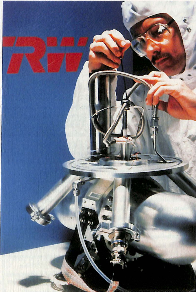
TRW INC. A technician at TRW's Space & Electronics Group puts the finishing touches on the thruster assemblies of a company-developed lightweight spacecraft that will carry NASA's TOMS-EP (Total Ozone Mapping Spectrometer-Earth Probe) in 1994 for accurate measurements of Earth's ozone layer.
