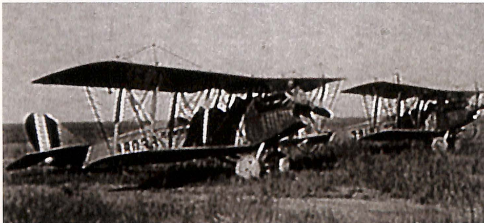
THE JENNY The Curtiss JN-4 training plane was the most widely produced American design of World War I and the mainstay of the U.S. civil and military aviation in the 1920s.
