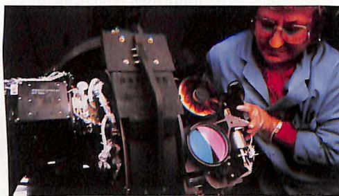
MARTIN MARIETTA CORPORATION A quality control technician inspects sensors on the TADS/PNVS system that enable Army AH-64 Apache helicopters to fly low level missions at night or in bad weather.
