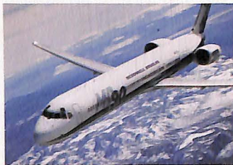
MCDONNELL DOUGLAS CORPORATION In February, the MD-90-30 entered flight test status. The MD-90-30, planned for certification in October 1994, is a 153-passenger stretched version of the MD-80. An extended range MD-90-50 is being offered for 1995 delivery.
