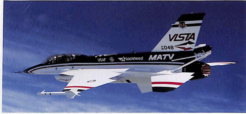
LOCKHEED FORT WORTH COMPANY/ GENERAL ELECTRIC COMPANY A joint USAF/industry program resulted in a successful operational concept demonstration of an F-16 aircraft modified with a MATV (Multi-Axis Thrust Vectoring) engine nozzle.
