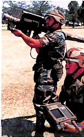
TRW INC. The Army's FAAD C2 (Forward Area Air Defense Command and Control) system, developed by TRW's Systems Integration Group, gathers battlefield intelligence and air defense targeting data and distributes it to commanders and two-man gunner teams.
