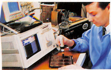
WESTINGHOUSE ELECTRONIC SYSTEMS Using nothing more than a screw driver, a company engineer assembles multi-chip packages, without solder, for an electronic module of the Comanche helicopter's mission computer cluster, demonstrating the Westinghouse-developed Solder-Free Interconnect technology.
