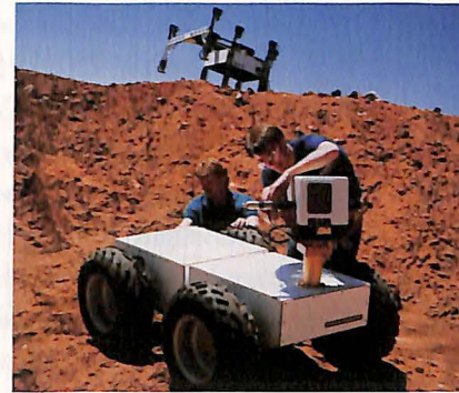
MARTIN MARIETTA CORPORATION Undergoing test at Martin Marietta is a pair of robotic systems designed for 21st century Mars exploration. In foreground is a wheeled rover and in background a "walking beam" rover.
