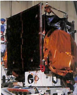
HUGHES SPACE AND COMMUNICATIONS COMPANY In May, an Ariane launch vehicle boosted Hughes' Astra IC satellite, which will provide direct-to-home broadcasting services across Europe under the sponsorship of Société Européenne des Satellites. In photo, a pre-launch view of Hughes technicians adjusting the satellite's thermal blankets.
