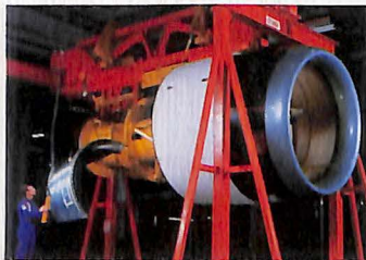
ROHR, INC. In production at Rohr are nacelle systems for the GECF6-80C2 engine; in photo, a core cowl is test fitted with an engine.
