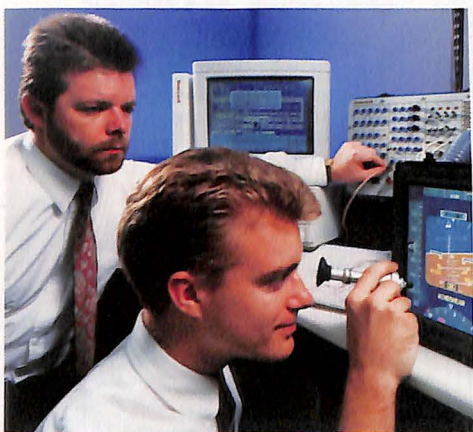
HONEYWELL INC. At Honeywell's Air Transport Systems, engineers check the resolution of a new-generation flat panel cockpit display developed for the Boeing 777.
