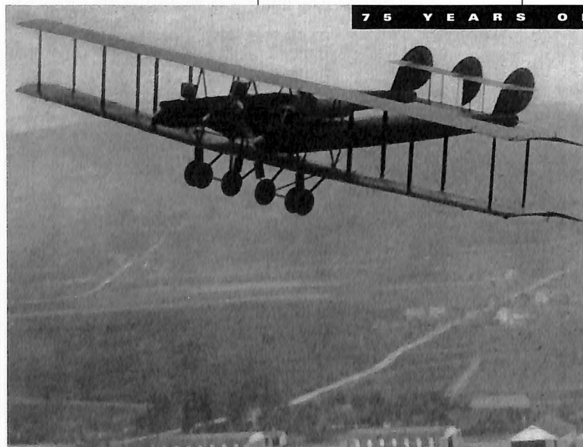
Described as "America's largest airplane" in 1920, the three-engine, 107-foot wingspan Model H Giant was built by L-W-F Engineering Company.
