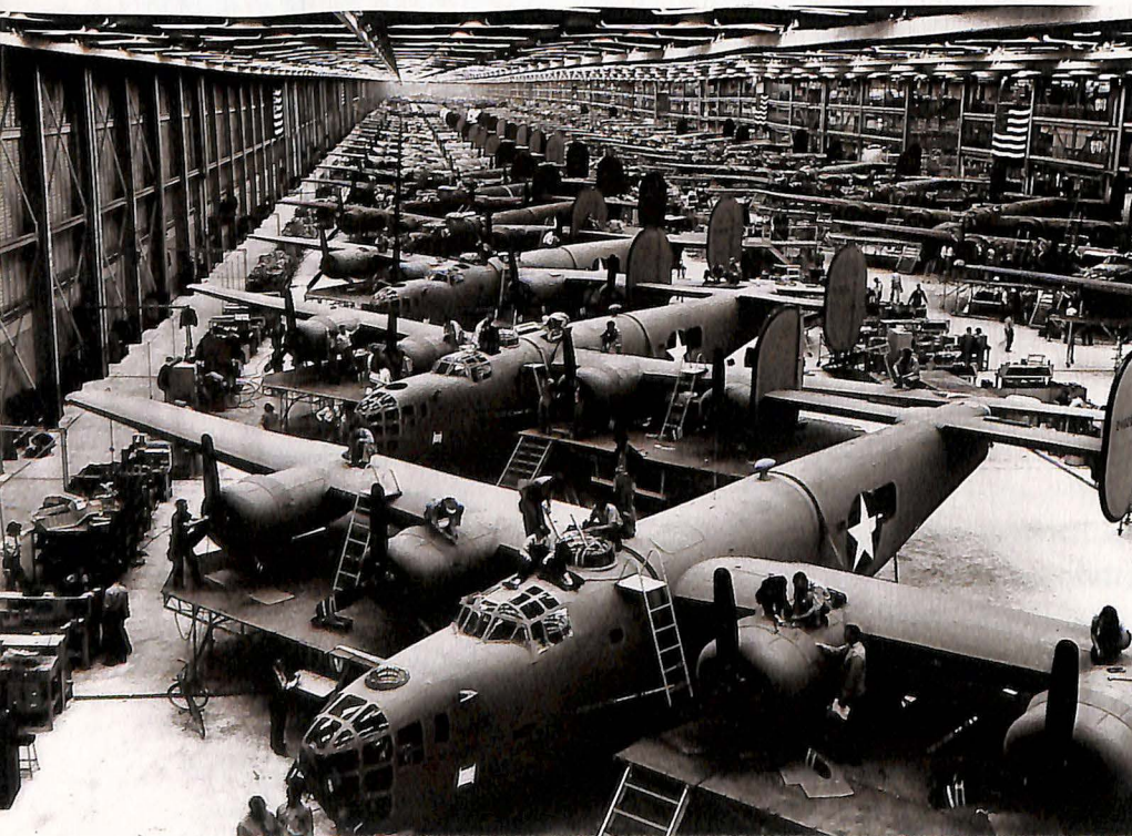
THE PRODUCTION MIRACLE OF WORLD WAR II Barely out of its adolescence, the U.S. aircraft industry incredibly produced more than 277,000 planes in the four-year span 1942-45. In photo, B-24s under construction at Consolidated Vultee Aircraft Corporation.
