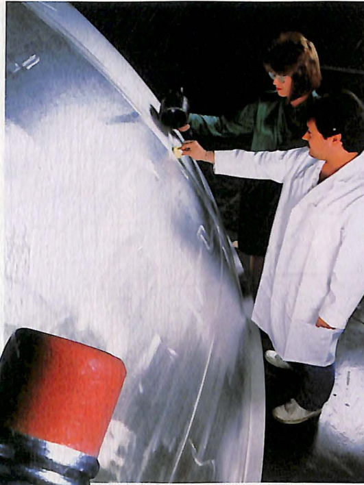
MARTIN MARIETTA CORPORATION At year-end, Martin Marietta Manned Space Systems awaited a NASA go-ahead for development of a Superlightweight External Tank for the Space Shuttle; substitution of aluminum-lithium components could reduce the weight of the 66,000 pound (empty) tank by 8,000 pounds. In photo, a full-scale aluminum-lithium quarter dome assembly developed by the company.
