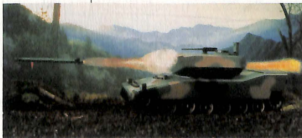
LORAL VOUGHT SYSTEMS CORPORATION In technology demonstration status was the LOSAT (Line of Sight Anti-Tank) missile system. In photo, the new, lighter LOSAT vehicle that offers easier transportability and greater firepower.
