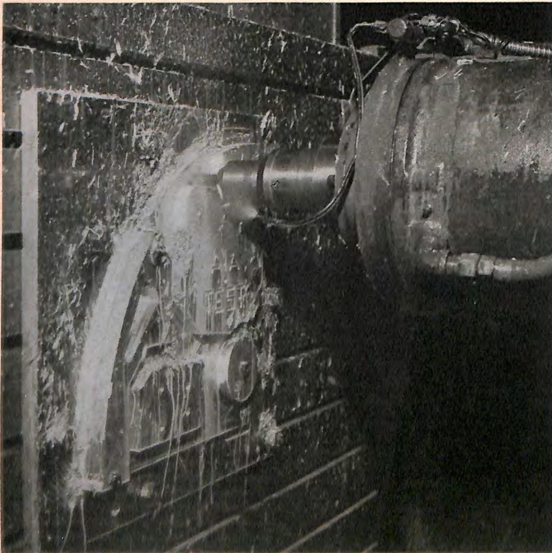
Milling machine cutting the "AIA Test part." This "part", designed to show observers the capabilities of APT III, was programmed automatically by a digital computer.
