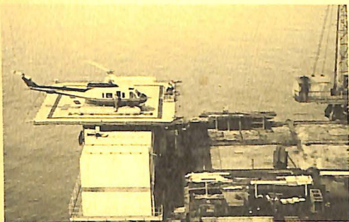
A Bell 204-B, 10-place helicopter daily transports crews to and from oil rigs in the Gulf of Mexico. There are more than 100 of these helipad-equipped oil rigs in the Gulf serving the petroleum industry.
