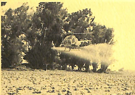
A Hughes 269A helicopter can be equipped with spray booms. It is estimated that one agricultural type helicopter can do the spray work of 3 fixed-wing airplanes.
