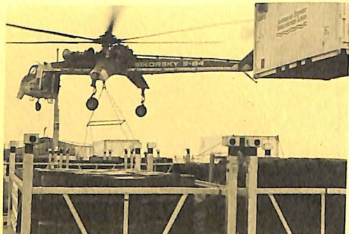
A Sikorsky Sky-Crane heavy lift helicopter off-loads cargo from ship to shore.
