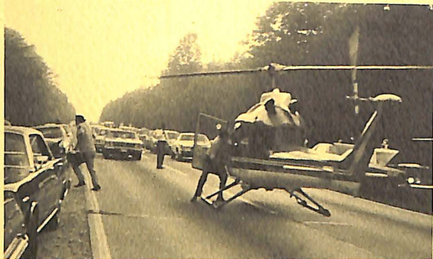
A Fairchild Hiller turbine-powered FH-1100 ambulance helicopter, equipped with two inside litters, seat for medical attendant, plus pilot, lands near a highway accident.
