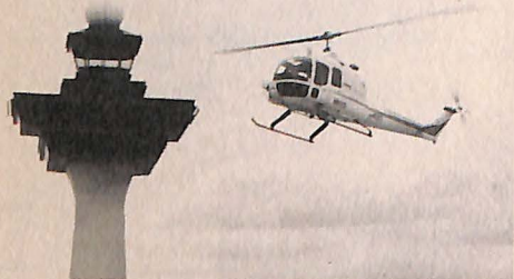
An executive model of the Fairchild Hiller FH-1100, 5-place, turbine-powered helicopter, lands company executives at Dulles International Airport for connecting airline flights.
