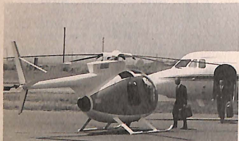
The Huey 500, a 5-place, turbine-powered helicopter, is used by modern industries for fast portal-to-portal transportation for company executives.
