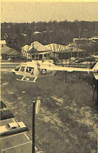
Atlanta (Ga.) Citizens & Southern Bank uses 5-place, turbine-powered Bell JetRanger helicopters for daily pick-up of checks and drafts from its 30 branch banks. Where no heliport is available, a unique pole-pick-up is used. With a long metal hook, the plastic tube containing the deposits is lifted off a 60 feet high pole into the hovering helicopter.
