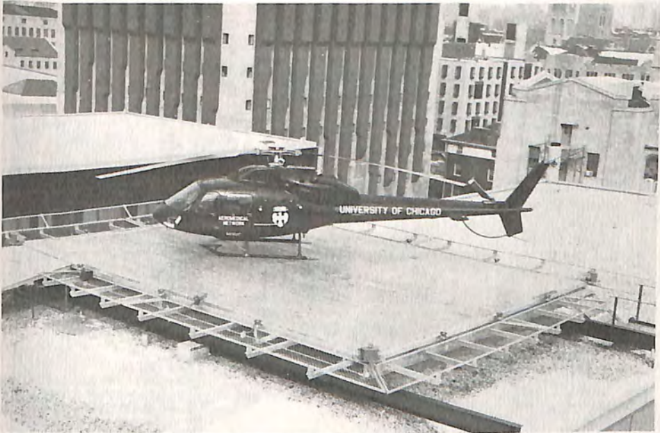
An Executive Helicopters ambulance helicopter lands on the University of Chicago Medical Center's rooftop pre-fabricated, aluminum Norsk-Lander Helideck.
