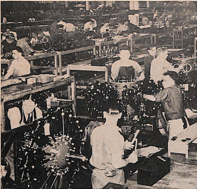
This is how the production line at Pratt & Whitney's East Hartford, Conn., plant looked during the war, when P&W was building the R-1830 engine. "Impossible" deadlines and frequent design changes made job difficult, but it was done.
