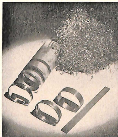
Finished parts (above) show savings with new method. Left, two pounds of scrap remain after part is machined. Right, completed part formed from strip stock with no loss of material.
