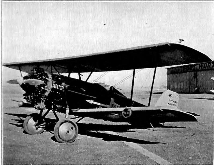
(Top) Cessna 6-passenger monoplane with Wright Whirlwind . (Bottom) Texas Air Transport's Pitcairn Mailwing , Whirlwind powered.
