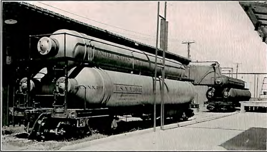
Tank cars for helium. Each car has 200,000 cu. ft. capacity under pressure of 2,000 lbs. to the square inch.
