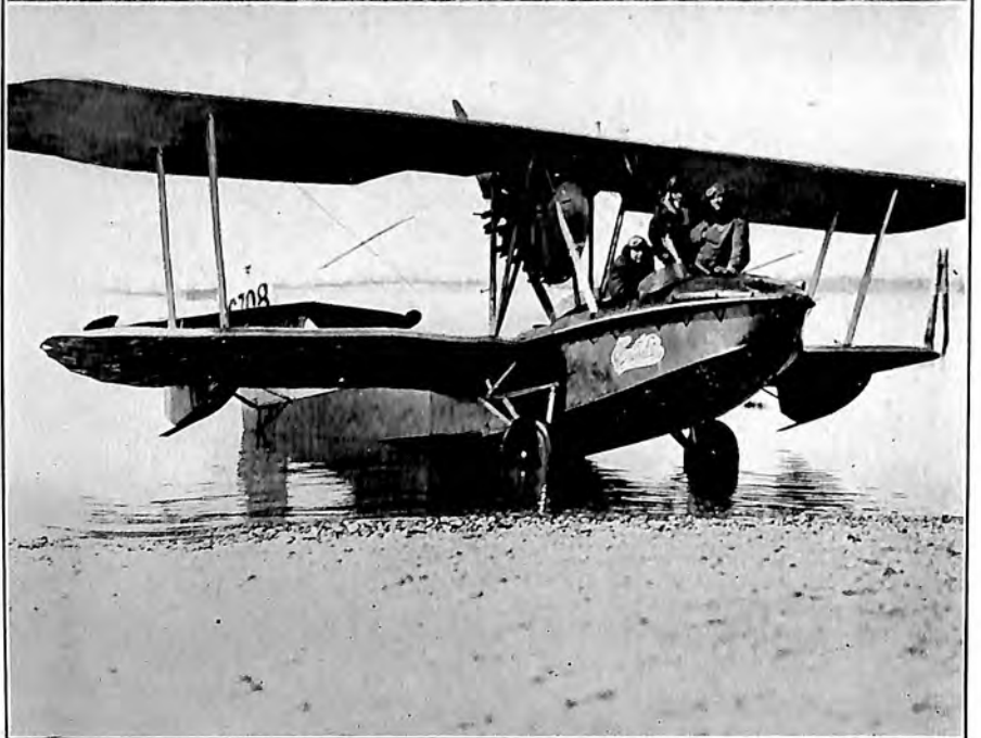
(Top) Hamilton Cabin Metalplane, Pratt and Whitney Wasp . (Bottom) Ireland Amphibian, Wright Whirlwind .
