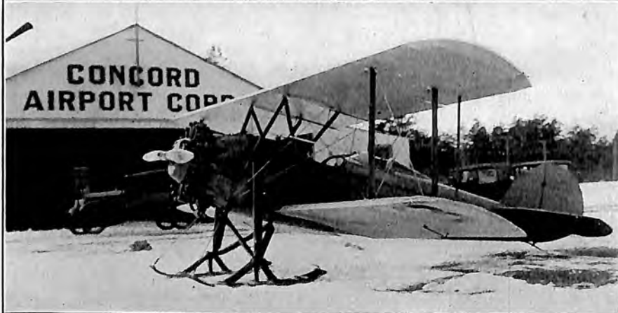
(Top) Curtiss Falcon mail plane built for National Air Transport. (Center) One of the Interstate Airlines Fairchild passenger planes. (Bottom) R. S. Fogg's Sport Waco , Whirlwind powered, equipped with skis, at Concord, N. H.
