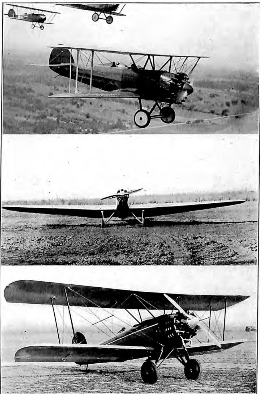
(Top) Advance Sport Waco planes, Whirlwind powered. Center) Aero-marine Klemm, Salmson engine, monoplane. (Bottom) Kreider-Reisner, Warner Scarab .
