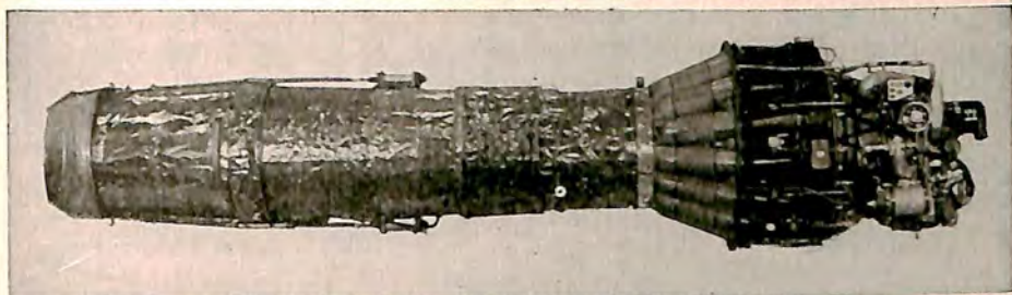
Allison J-33-A-33 is equipped with long afterburner for bursts of added power in Lockheed F-94
