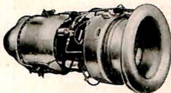
DUCTED FANS with wide potential utility as means of increasing speeds of small and medium-sized military and civilian utility aircraft. 500-800 lbs. thrust.
