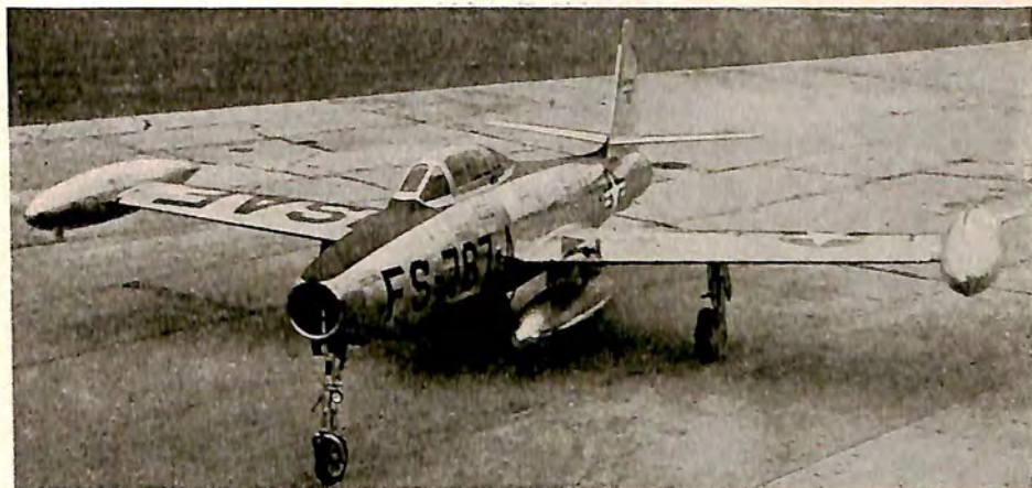
Republic Thunderjet equipped for mid-air refueling
