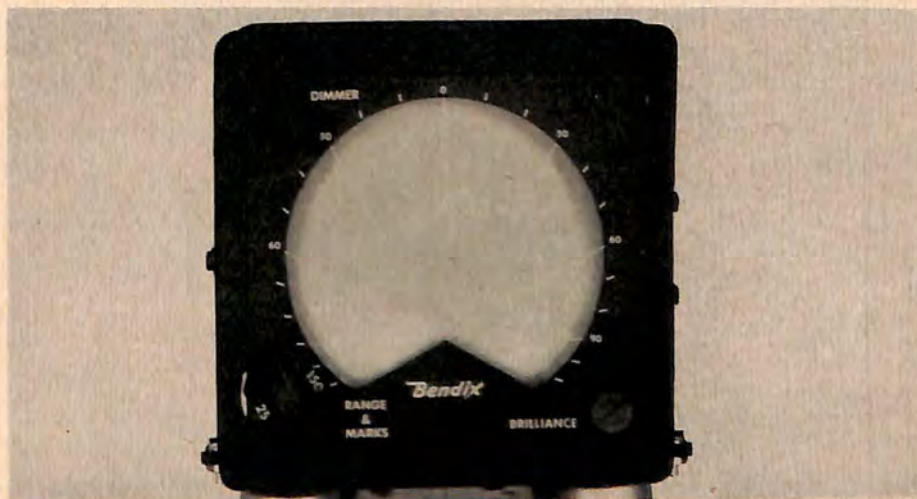
PPI Indicator on Bendix Airborne Radar System
