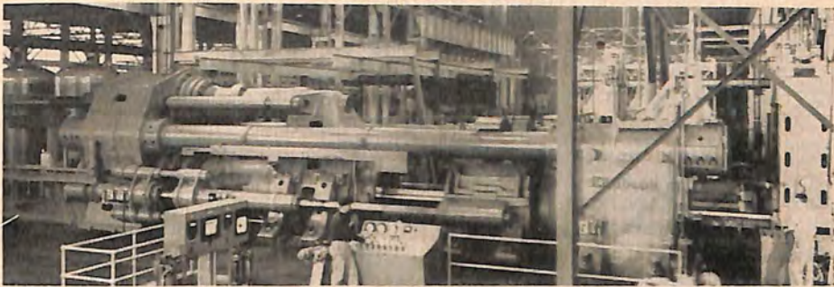
Alcoa's 14,000-ton extrusion press
