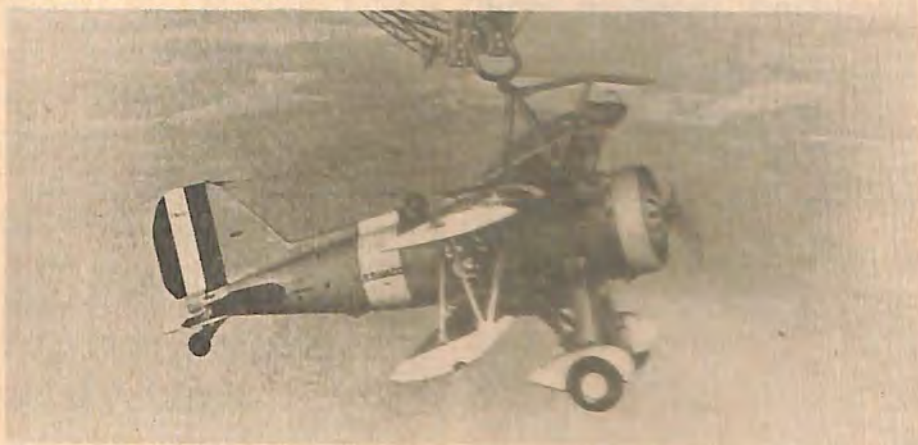
Curtiss F9C-2 engaging hook landing gear on bottom of Airship Macon
