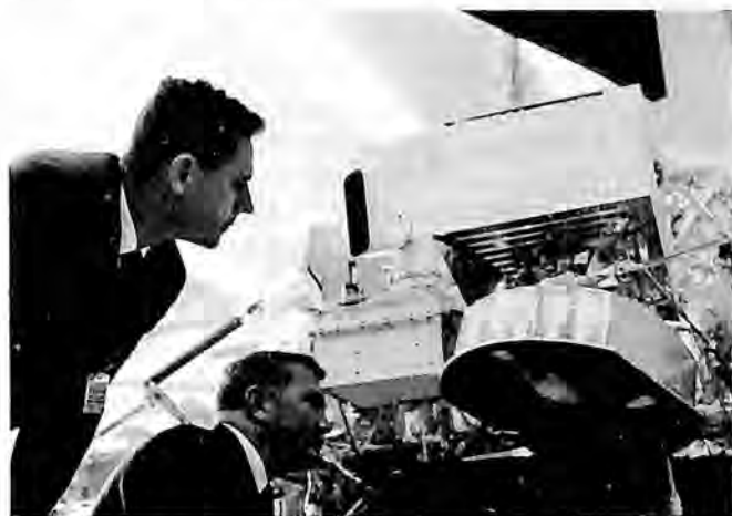
Ryan officials inspect company-built Radar Altimeter Doppler Velocity Sensor System, a key element in Surveyor soft-landings.
