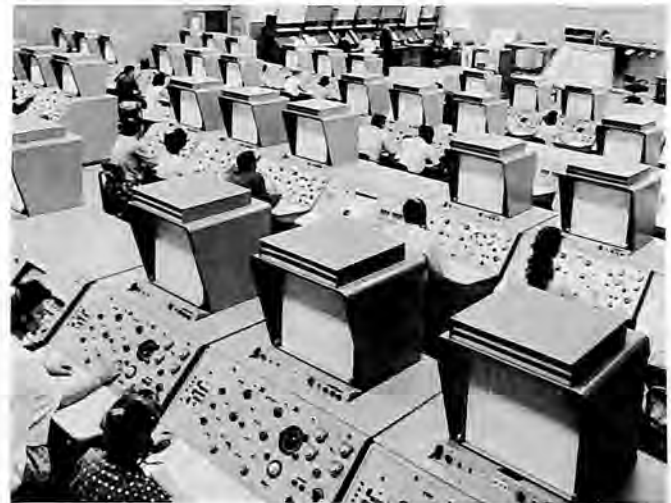
FAA "pilots" at the National Aviation Facilities Experiment Center simulate aircraft flights which show up on radar scopes in an adjoining radar as "blips" or "slashes."
