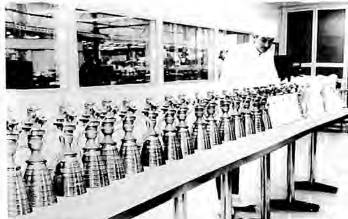
Marquardt 100 pound thrust rocket engines, used in Apollo and Lunar Orbiter spacecraft, are assembled and inspected under sterile clean room conditions.
