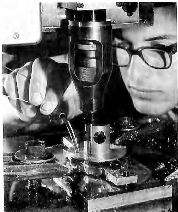
Example of precision is this special machine used by Aerojet-General's Downey plant to make a part for the Apollo propulsion system. In 1½ hours, the machine drills 2,300 precisely-spaced holes .030 inches in diameter.
