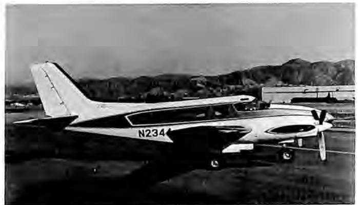
PAC's turboprop Tradewind, a remanufactured airplane engineered around the Twin Beech airframe, was certificated in May.
