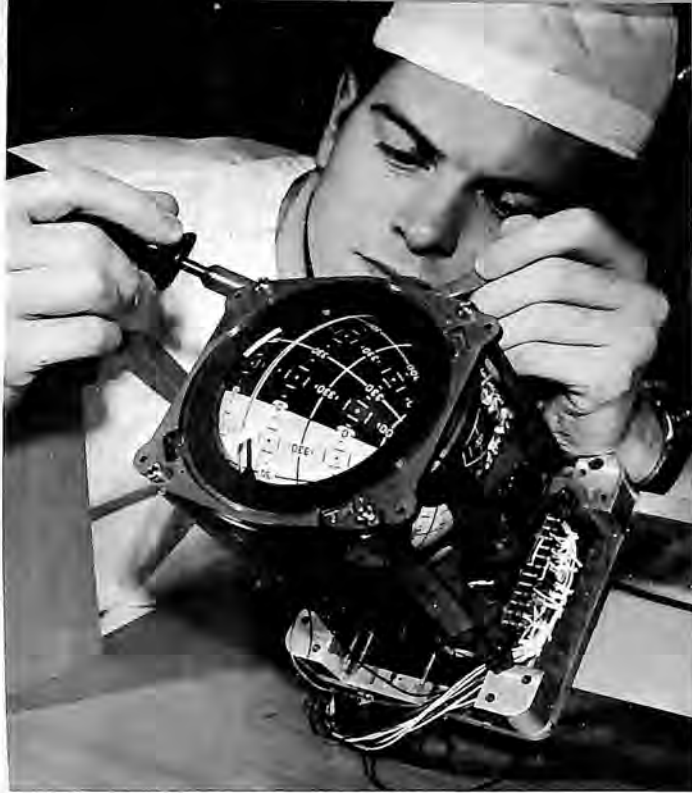
Honeywell technician adjusts flight director attitude indicator, Apollo instrument being produced by the company's Aerospace Division.
