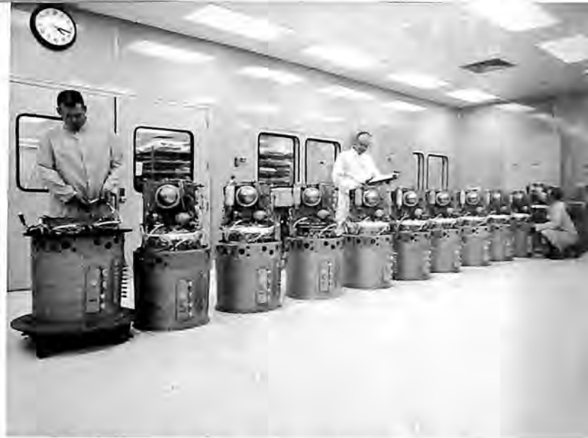
Pratt & Whitney Aircraft was supplying Powercels, trademark name for its fuel cell powerplants, for the Apollo spacecraft.
