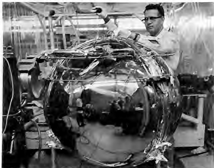
Beechcraft Boulder Division worker assembles cryogenic storage vessel for Apollo Lunar Module.
