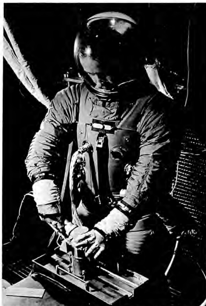
Being tested at simulated 380,000-foot altitude is Hamilton Standard's experimental hand-held beam welder, under development for space repair and assembly tasks.
