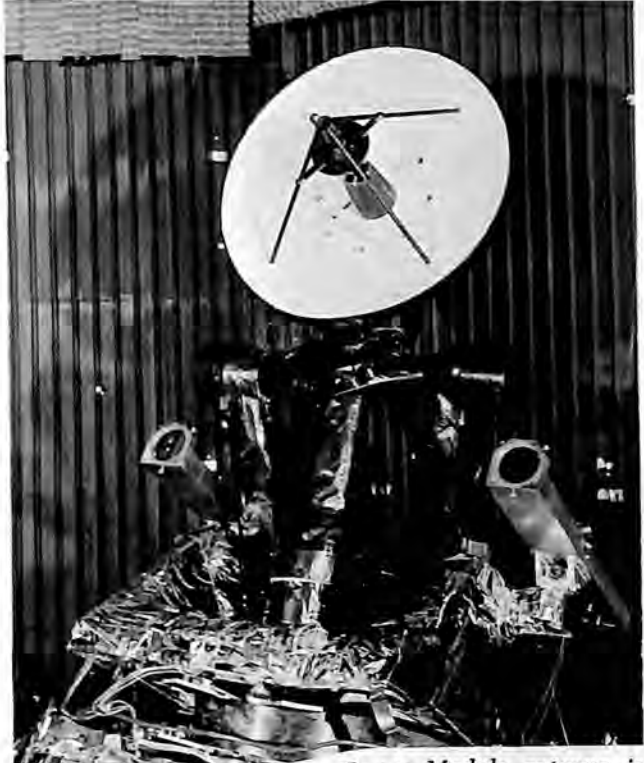
Engineering model of the Lunar Module antenna is tested in a vacuum chamber at RCA Space Center.
