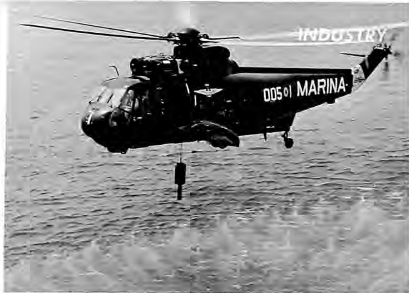
Sikorsky SH-3D practices sonar work in Long Island Sound before delivery to Spanish Navy.
