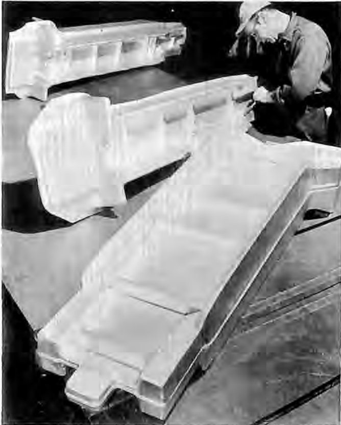
Alcoa's Cleveland Works produced high-strength forgings for the Uprated Saturn I launch vehicle.
