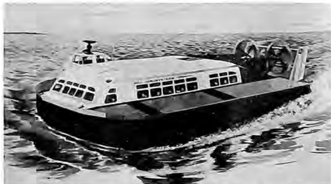
Bell Aerosystems announced plans to produce this 25-ton, 90-passenger Air Cushion Vehicle.
