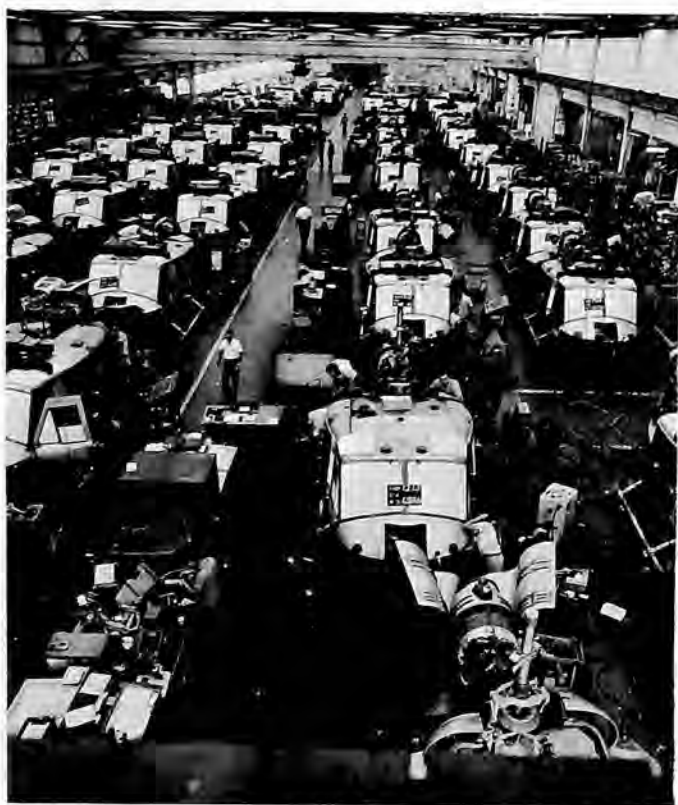
UH-1D's on final assembly line at Textron's Bell Helicopter Company.
