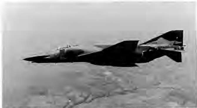
McDonnell was using an F-4 Phantom as a test-bed for mating the General Electric Vulcan cannon to the USAF/Navy fighter. USAF ordered a cannon-equipped F-4E.
