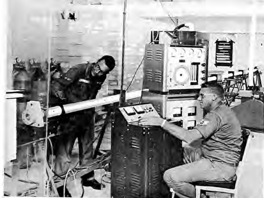
USAF technicians check control system of a carbon dioxide continuous-beam laser during installation of the free world's most powerful laser at the Air Force Weapons Laboratory.
