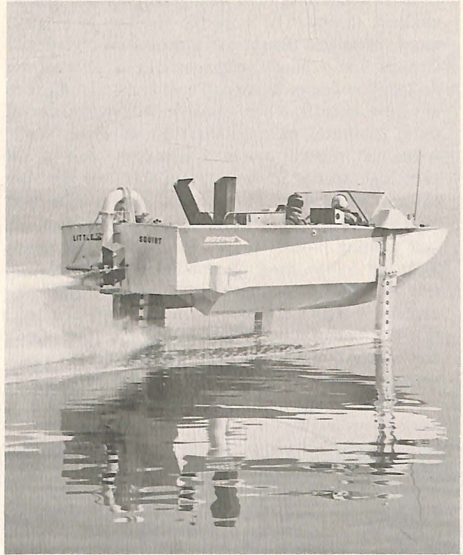
A Boeing Company crew takes an experimental hydrofoil on a test run.
