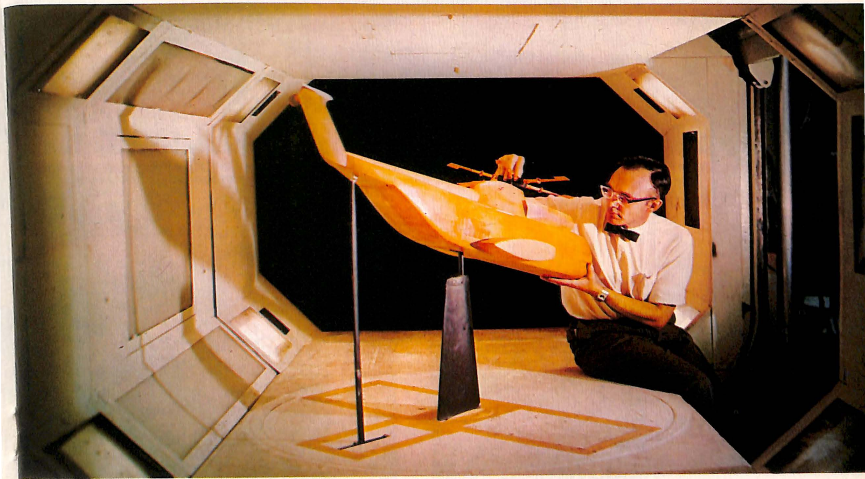
Charles Banning, United Aircraft Research Laboratories, makes a configuration change on a helicopter in a low speed wind tunnel.
