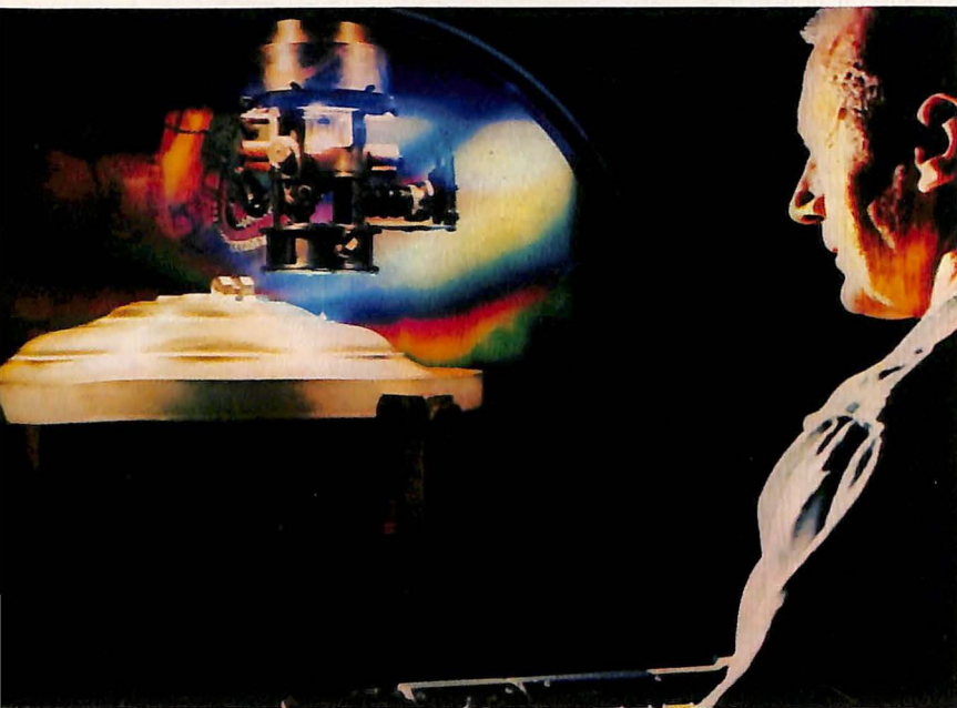
An Aerojet-General Corporation technician uses an electron beam to weld an injector for a rocket engine.
