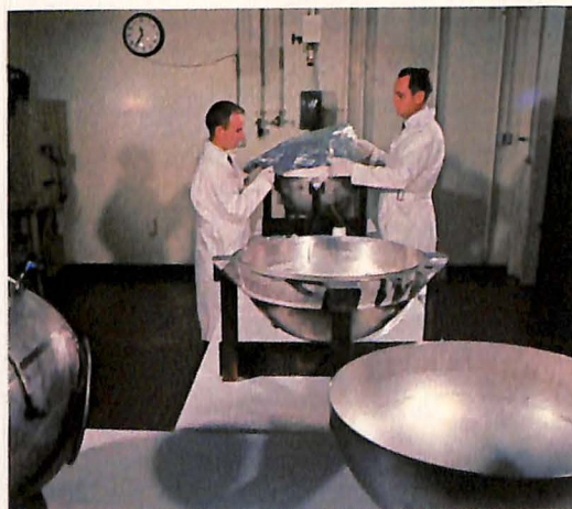
AiResearch Manufacturing Company experts apply insulation around a vessel used for storing liquid oxygen and hydrogen at super-cold temperatures aboard spacecraft.
