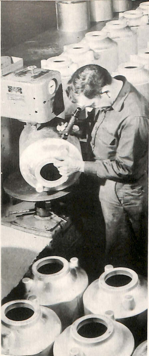
An Aluminum Company of America production worker welds forgings for a liquid rocket engine.
