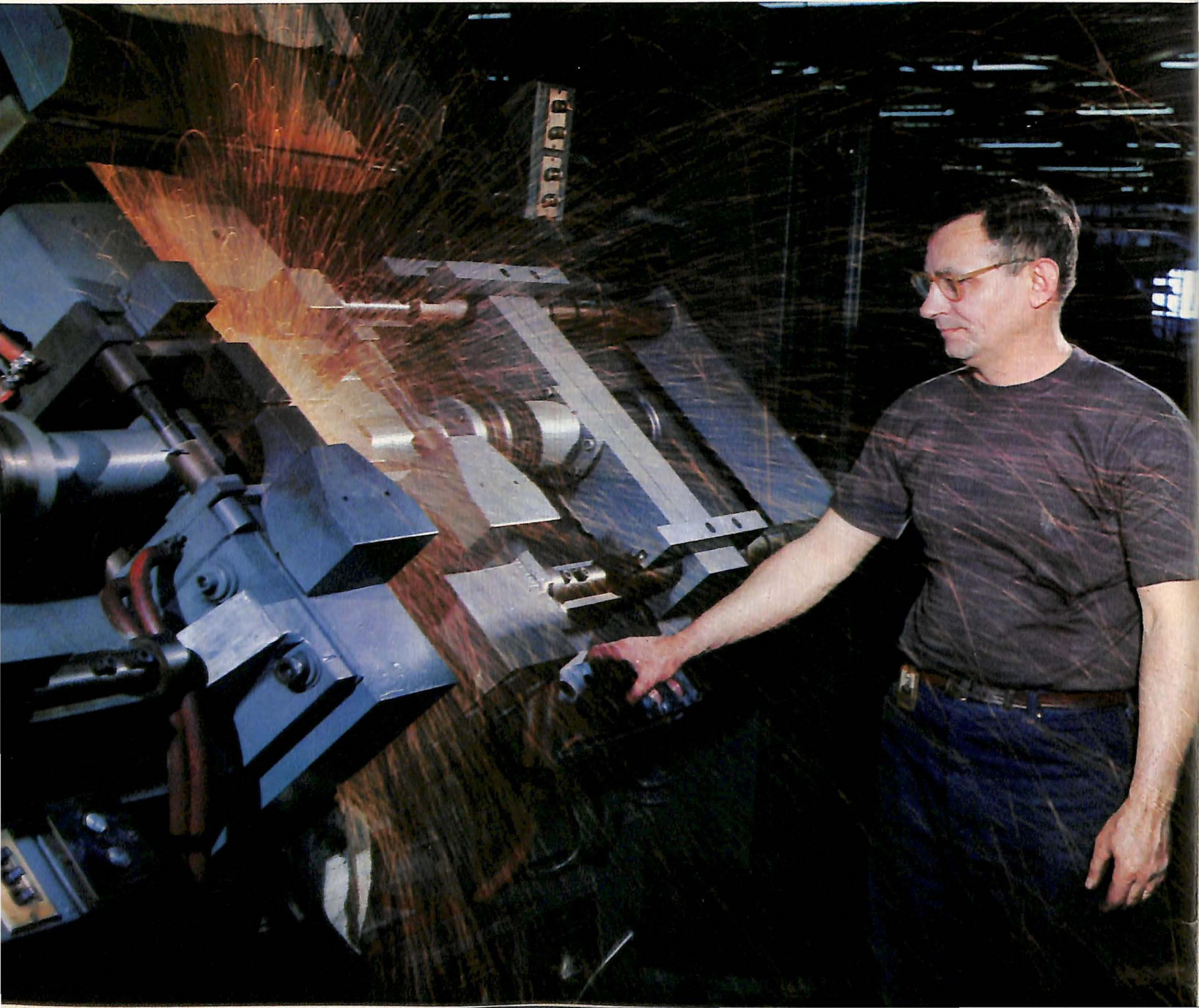
A production technician for the Sikorsky Aircraft Division of United Aircraft Corporation spot welds parts for a helicopter.
