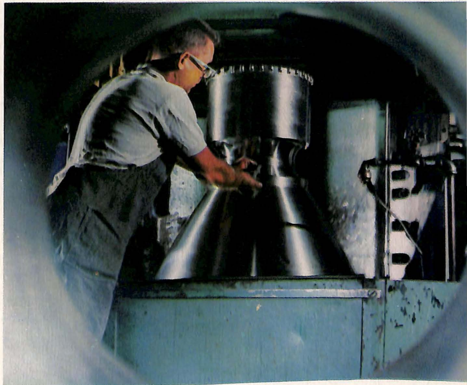
A descent engine for the Lunar Excursion Module is machined by a Ryan Aeronautical Company technician.
