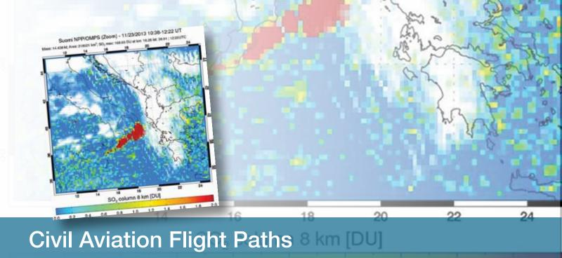
The Ozone Mapping and Profiling Suite (OMPS) that flies on the Suomi NPP spacecraft measures more than just ozone concentration. This Ball Aerospace-built sensor is useful for tracking dust and sulfur dioxide from volcanic eruptions.
