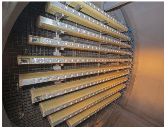
Figure 11: Spray bars mounted in PSL-3 inlet plenum (Ref 1)
