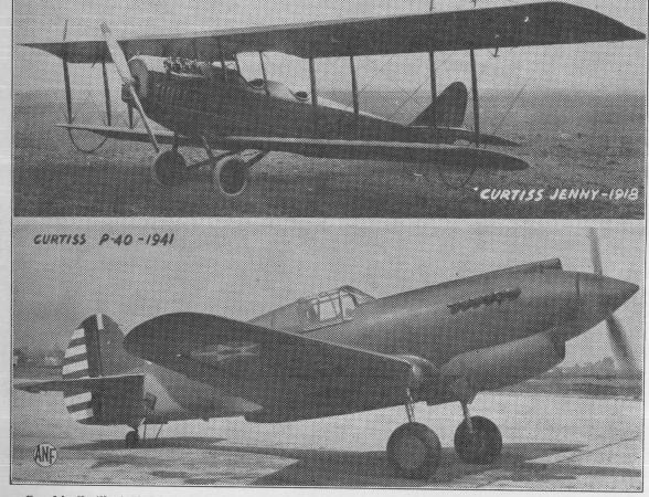
Graphically illustrated here is the progress made by American aircraft builders since 1918 in producing fast combat aircraft. The Curtiss JN or "Jenny" (upper) was powered with a 90-horsepower OX-5 motor. The modern Curtiss P-40, nicknamed the "Tomahawk" (below), is powered with a 1,090-horsepower Allison engine. This low-wing single-seater fighter has a maximum speed exceeding 360 mph, is among the world's fastest
