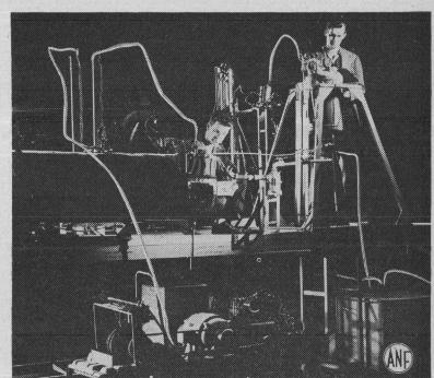
This strange-looking arrangement of tubes is really the complete fuel system of a modern fighting airplane, brought out into the open where it can be studied under test conditions. The picture, from the Aviation News Committee, shows engineers of Vultee Aircraft, Inc., subjecting the fuel system to the widely divergent pressures which would be encountered at various altitudes during flight. By such methods the American aircraft industry is speeding the building of the world's finest
