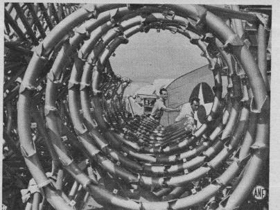
Futurism makes an unconscious debut at a busy aircraft factory. In this photograph from the Aviation News Committee, the camera's eye is focused through scores of tubular steel engine mounts ready for installation on Army bombers being rushed to completion at the plant of North American Aviation. In the background is a bomber wing bearing the Army Air Forces' insignia.
