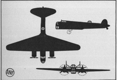
The Japanese "98" Heavy Bomber," used by the Japanese Army, is illustrated in this fifth of a series prepared by the Aviation News Committee to aid in recognition of enemy aircraft. A low wing, cantilever, metal monoplane, this bomber has full retractable landing gear and wing flaps. Note the broad taper of the wings from rounded tip to fuselage, and twin tail assembly.
