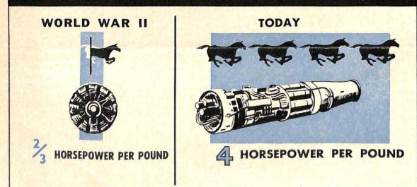
The engines which powered America's military aircraft at speeds in the neighborhood of 400 m.p.h. in World War II produced one horsepower for every pound-and-a-half of engine weight.
