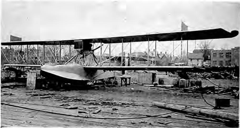
The Standard HS-2-L Flying Boat, with 12-Cylinder 320 H.P. Motor
