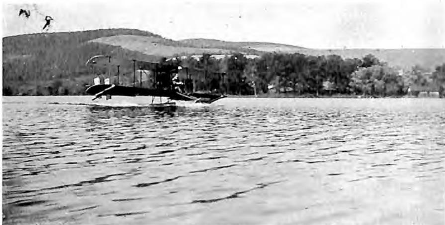
Model TA, with Pontoons, rising from the water for a flight
