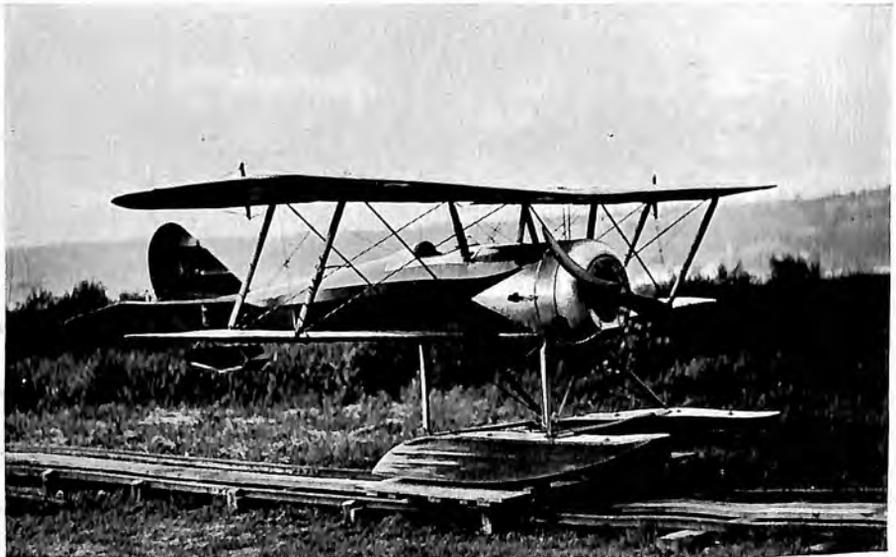
S-5 Scout, One Place, Twin Float, Hydro-aeroplane, 100 H. P. Gnome Engine
