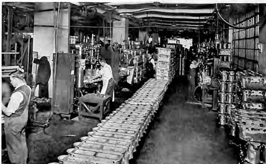
Machining line for the Aluminum Water-Jacket Casting in the Wright-Martin Foundry
