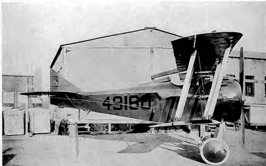
Model E-1—a defense advance training Tractor Aeroplane, single-seater with a 100 H.P. 9-Cylinder Rotary Gnome Engine
