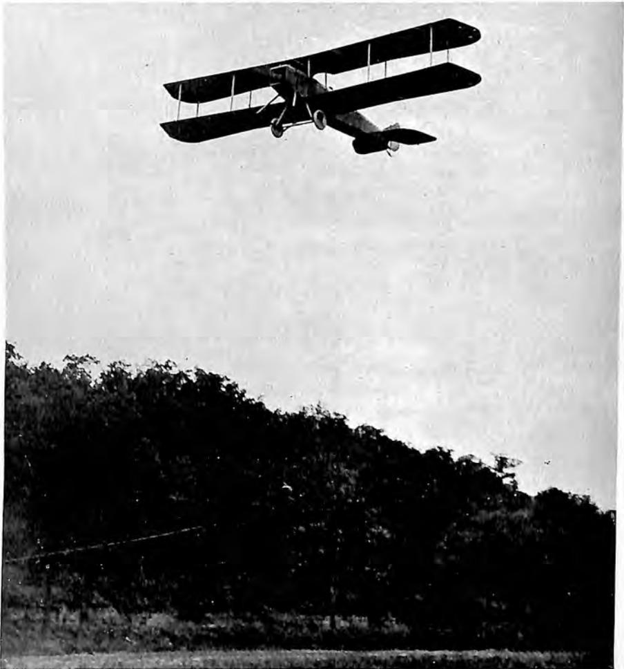
Model T-2 fitted with 90 H. P. Austro-Daimler Engine
