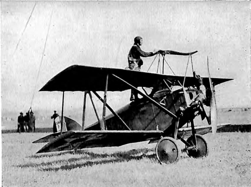
(Top) Army Air Service Blimp TC5 with Sperry-Messenger airplane that was launched while airship was in full flight. (Bottom) Close-up of Sperry-Messenger, Wright engine.—*U. S. Air Service.*
