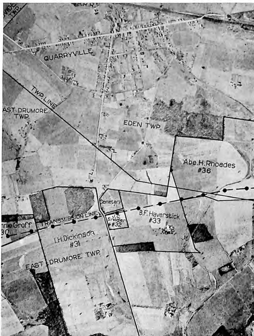
Section of aerial photographic map used in projecting high tension transmission line. Savings of over 50% in cost of right of way have been reported from such use of aerial maps.—Fairchild Aerial Surveys, Inc.
