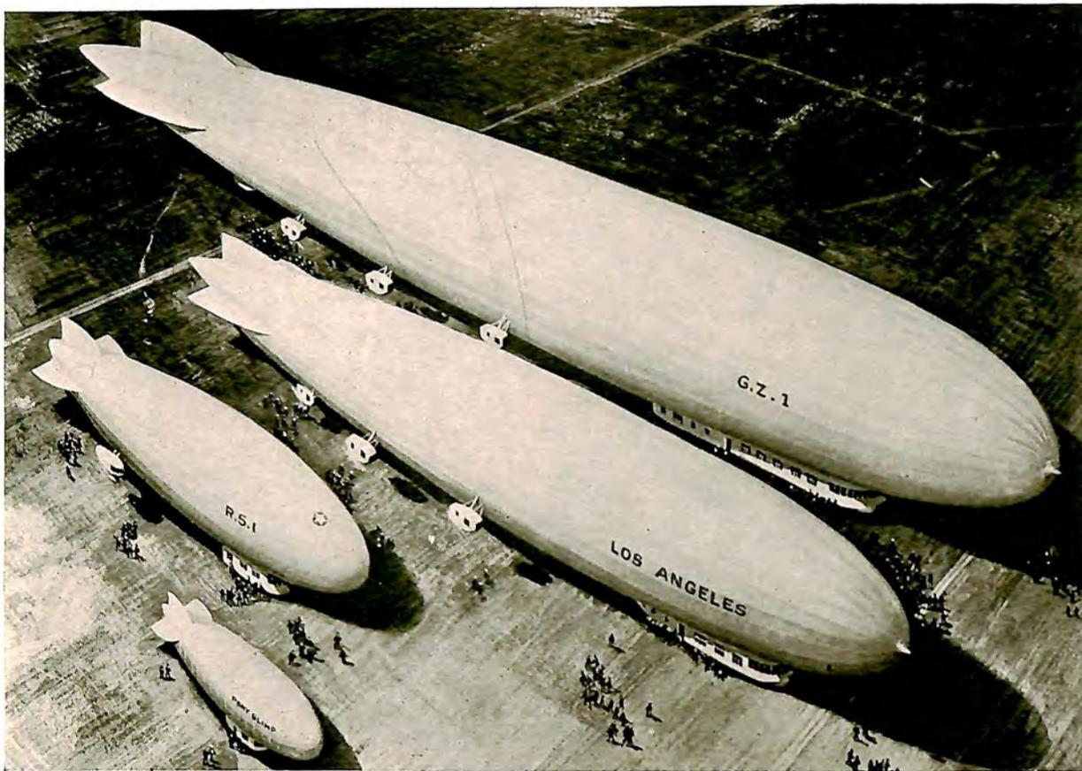
Comparative drawing of commercial airship development. *Pony Blimp* and *RS1* constructed by Goodyear Tire & Rubber Co. *Los Angeles* built by German Zeppelin Co. Type *GZ1* Super-Commercial-Dirigible under designs by Goodyear-Zeppelin Corp.
