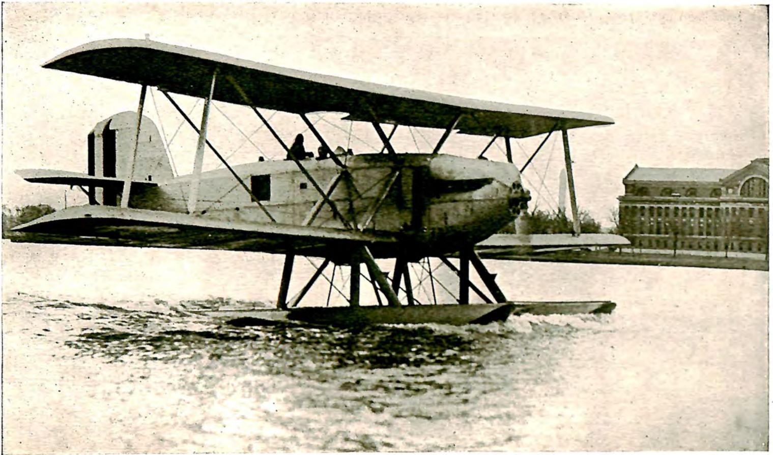
Navy Curtiss C.S.2, Wright engine. Three purpose, scouting, bombing and torpedo seaplane. Holder of World's records for seaplane endurance and distance flown in non-stop flight.—*Navy Bureau of Aeronautics.*
