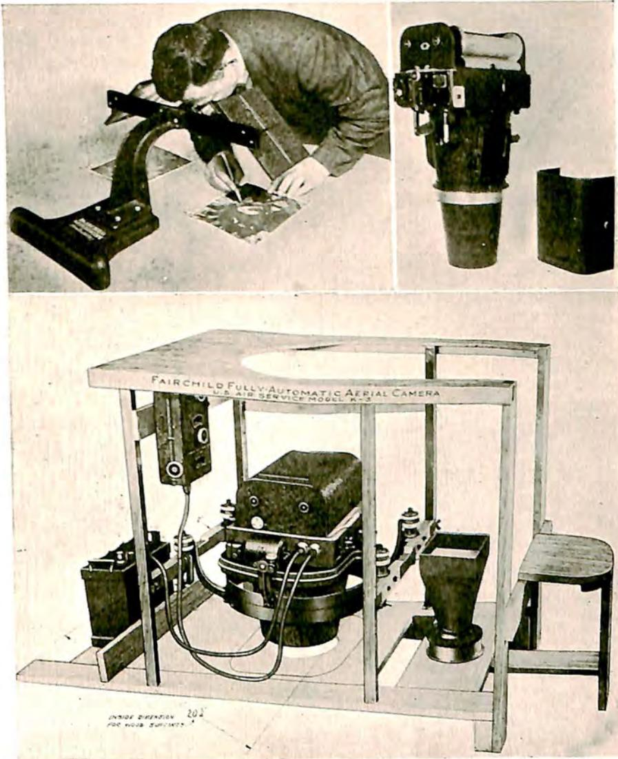
(Upper Left) Fairchild mirror stereoscope which brings into relief position of terrain common to overlapping vertical aerial photographs. (Upper Right) Fairchild K6 Aerial Camera. (Bottom) Fairchild K3 Automatic Aerial Camera, official mapping camera of United States Army and Navy Air Services and Canadian and Brazilian Governments.
