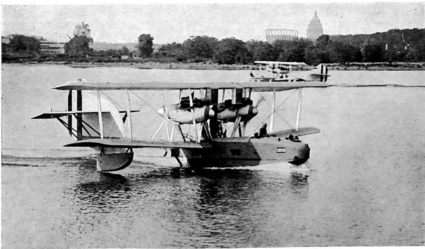
Navy P.N.-7, Metal Hull Patrol Seaplane, 2 Wright engines, with which weight carrying records were made at Naval Air Meet, Bayshore Park, Md., October 25, 1924.—*Navy Bureau of Aeronautics.*
