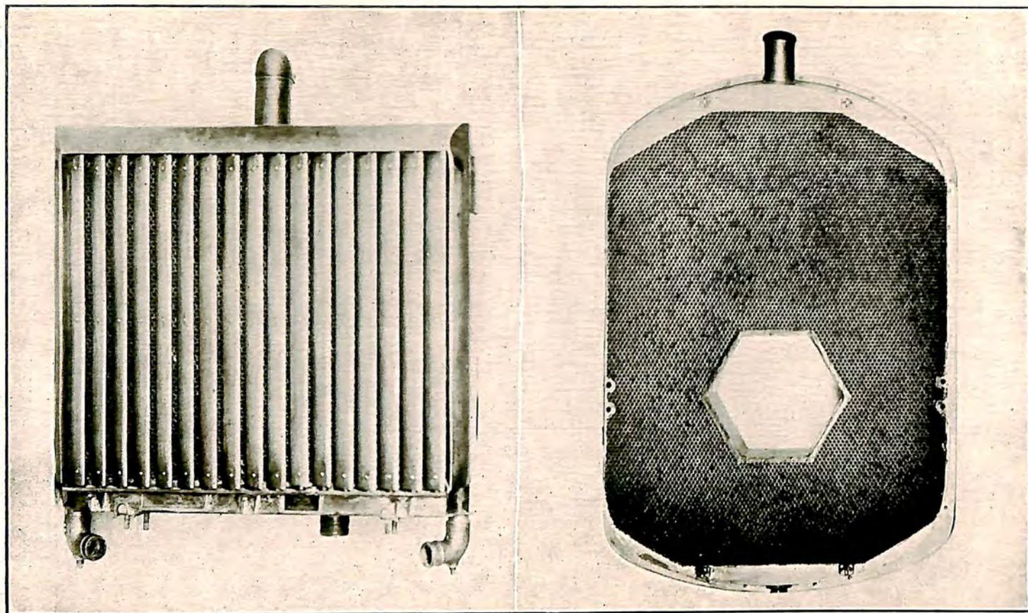
(Left) Radiator developed by U. S. Cartridge Co. for Glenn L. Martin Bomber. (Right) Radiator developed by U. S. Cartridge Co. for Stout Metal Airplane Co.
