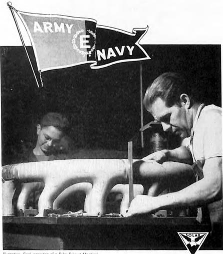
Illustration Final inspection of a Solar Exhaust Manifold.
