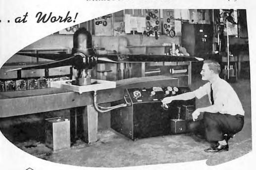
Hydromatic Propeller Test Stand, for testing distributor valves and feathering action of Hydromatic Propellers.
