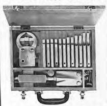
The production type Jacoel Splicer has a capacity for 1/16 to 5/16 diameter cable for Thimbles, Bushings, Spacer. Used by U.S. Government, Aircraft Factories, Schools, Repair Stations.
