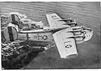
BIGGER THAN A BOXCAR, the Consolidated Coronado (PB2Y) carries many tons of cargo, has a range of thousands of miles, can stay aloft for more than a whole day at a time. Mass-production built, these monsters are completely equipped with galleys and crew quarters.
