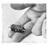
Although it's small, the G-F Switchette has double-break contact construction. It weighs only ½ ounce and measures 134 by ½ by ½ ½ in. Made in single or two-circuit form. One contact normally open—one closed; or vice versa.
