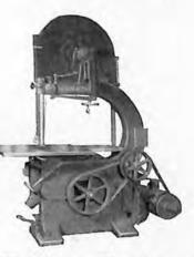
DIES can be sawn with the Type 24M in a small fraction of the time required by other methods. Also files and polishes. Available in 24" and 36" throat capacity.
