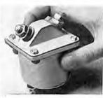
Dynamotor contactor—will handle an inrush of 500 amperes at 32 volts. It operates on either 12 or 24 volts, d-c. Provides one single-pole normally open contact; has a 50-ampere rating based on NEMA 8-hour test.
