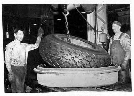
GOODYEAR NON-SKID PLANE TIRE Thousands of spiral metal springs are embedded into the tread to increase resistance to skidding.
