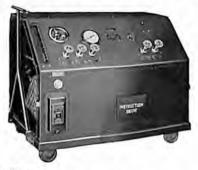
Stand for determining burst pressures of devices in hydraulic systems.
