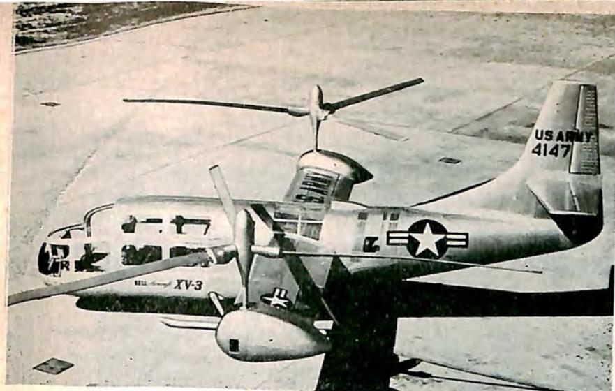
Convertiplanes came out of the laboratories into the news. Bell flew its VTOL test vehicle, with two jet engines that rotate from vertical to horizontal for take-off, landing and flight. The same company announced its XV-3, with rotor props for vertical lift which tilt forward for normal flight.
