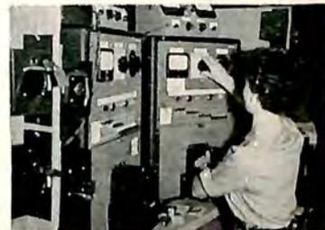
Some sealed relays have as many as 90 possible voltage breakdown points. This tester checks them automatically.
