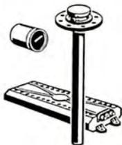
**CAPACITOR TYPE TRUE FUEL WEIGHT MEASURING SYSTEMS** . . . to provide an indication of the true weight of fuel remaining. Unlike either uncompensated or compensated type gages, these systems measure density and volume *directly* rather than depending on the highly variable relationship between fuel density and its dielectric constant. Density measurements are made by an electric hydrometer known as the Liquidensimeter. For further information, write for Bulletin 522.
