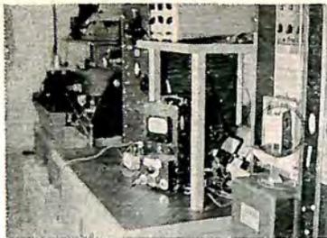
Tester built to JAN specification provides shock of over 100G's. Contact reactions are indicated on special equipment.
