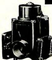
**FUEL PUMPS** Vane type for reciprocating engines, flow to 700 gph, pressures to 35 psi. Gear type for jet engines, flow to 200 gpm, pressures to 1500 psi, designed to supply main, after-burner, and emergency fuel requirements.
